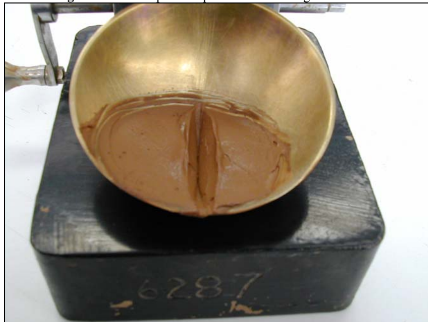
Figure 3.10 - Completed liquid limit test with groove closed.
