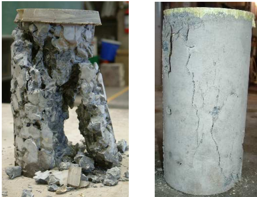
Figure 7.3 – Shows the shear failure mechanism of the no-fines concrete (left) and conventional concrete (right) after compressive strength testing
