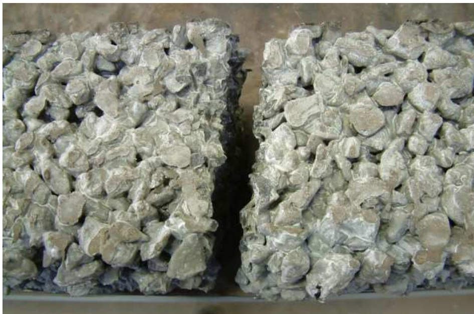
Figure 7.15 – The no-fines concrete Flexural Test failure on completion of the four-point loading test
