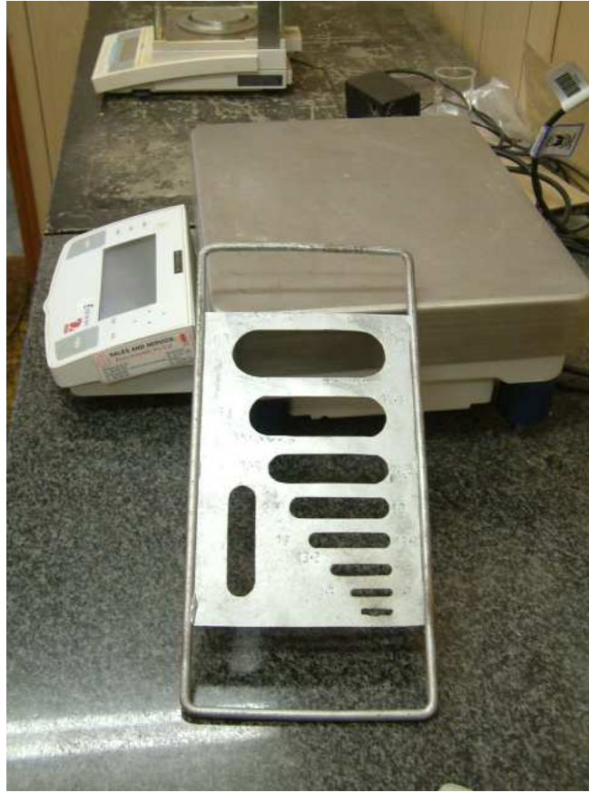
Figure 5.2 – Shows the slotted gauge used to determine the Flakiness of the aggregate particles
