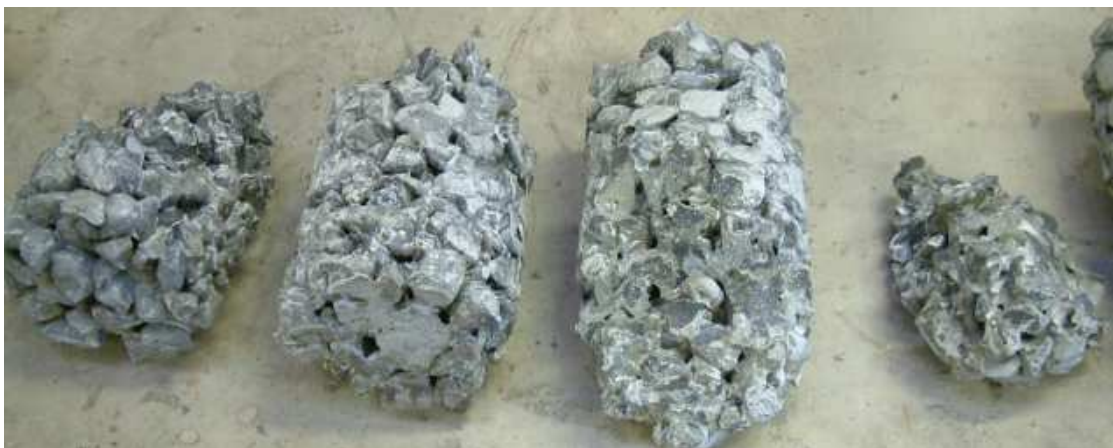
Figure 4.2 – The failure of Mixes 1 and 2
