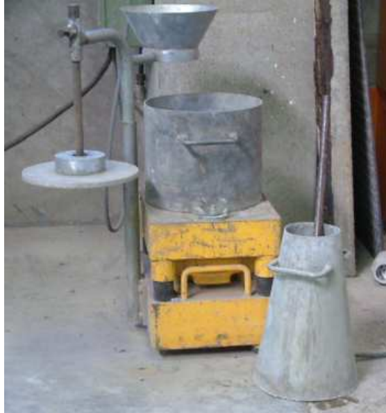
Figure 5.3 – Shows the Consistometer and other major components used in the VEBE Test
