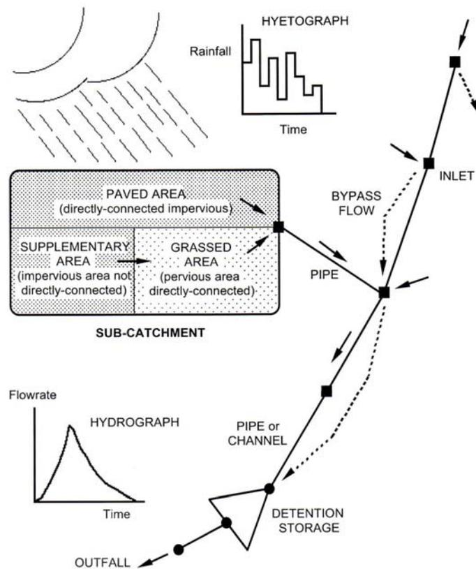
**Figure 4-7 – The Layout of the IIsax Model (O’Loughlin & Stack 2002, p. 6.8)**
