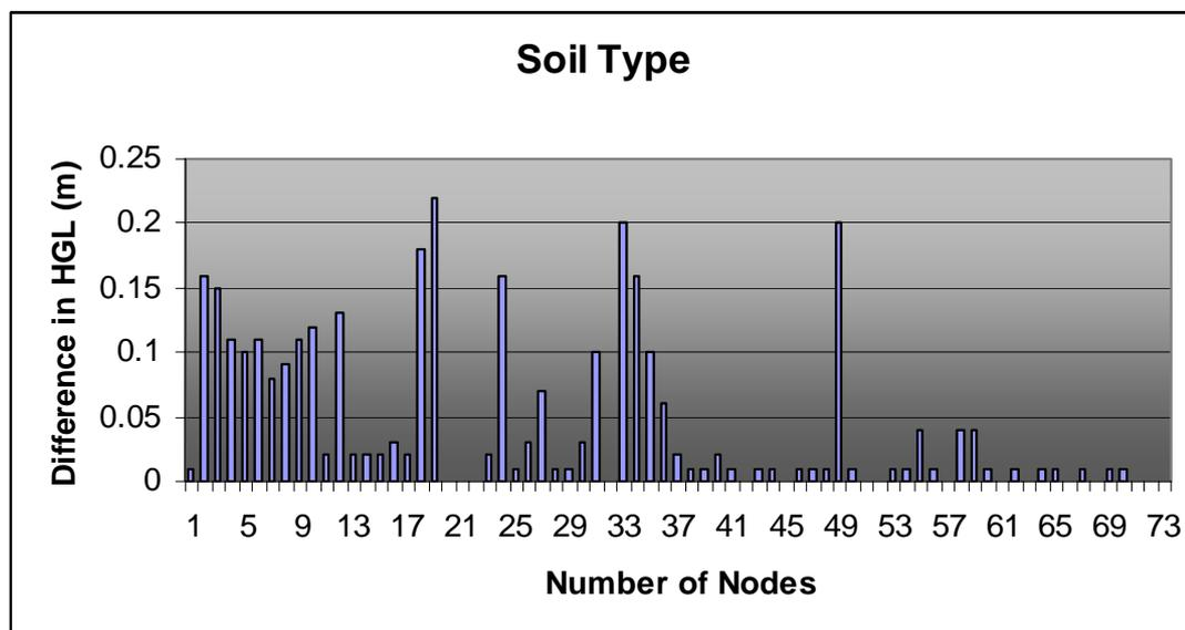
Figure 5-13 – Sensitivity of the model to varying soil types
