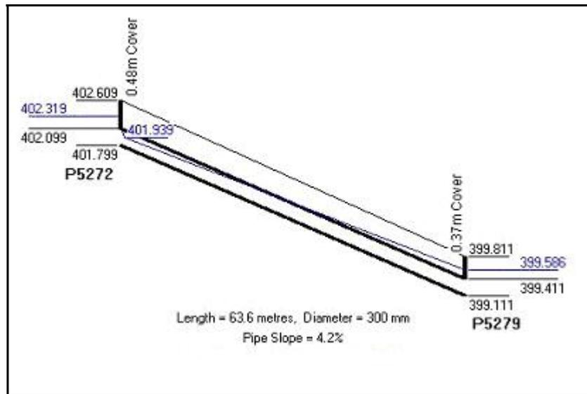
Figure 6-18 – Lowering the 300mm pipe to give a cover of 0.48 m
