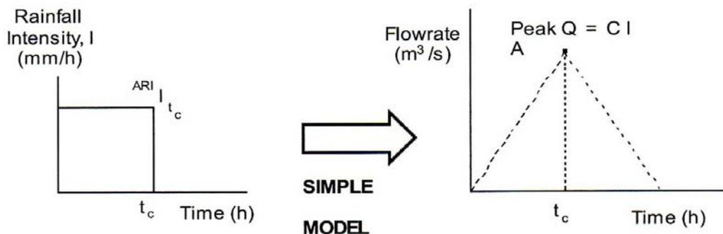
Figure 4-3 - Simple Rainfall Runoff Models (O’Loughlin & Stack 2002, p. 6.6)
