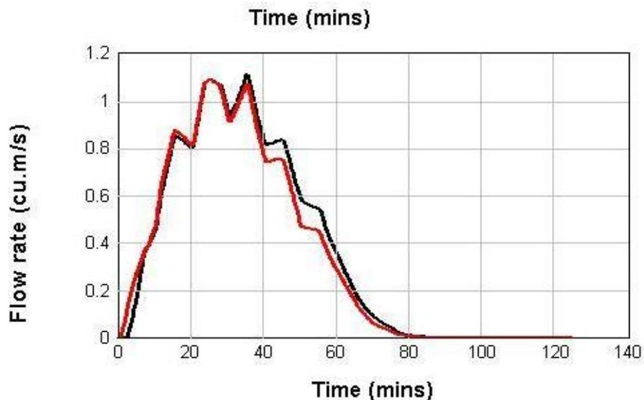
Figure 5-11 – Discharge Hydrograph for Major Design
