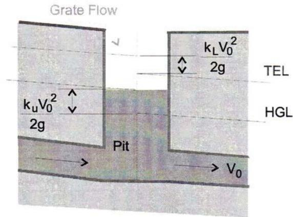
Figure 4-9 – Pit Energy Losses and Pressure Changes (O’Loughlin & Stack 2002, p. 6.40)
