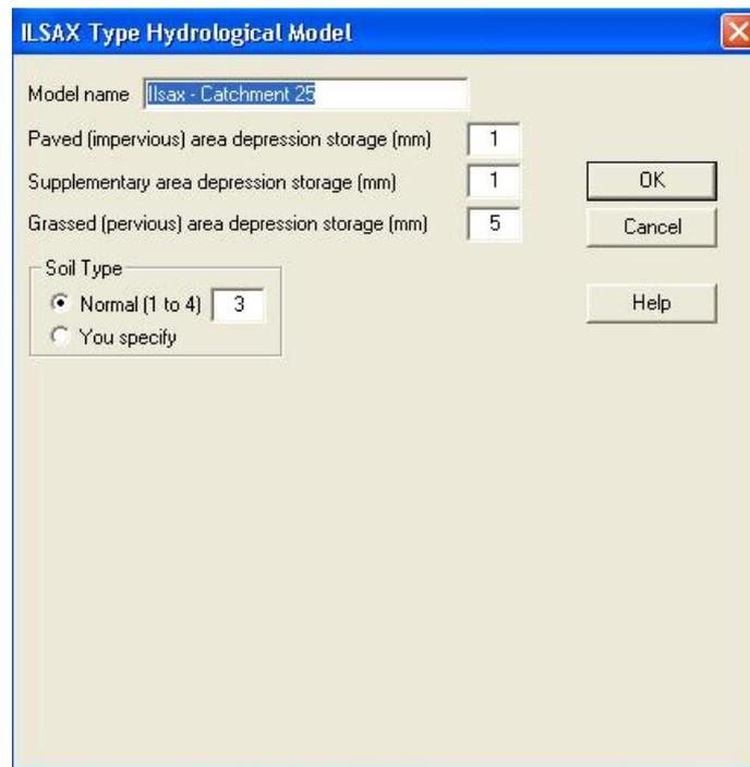
Figure 5-6 – IIsax type hydrological Model
