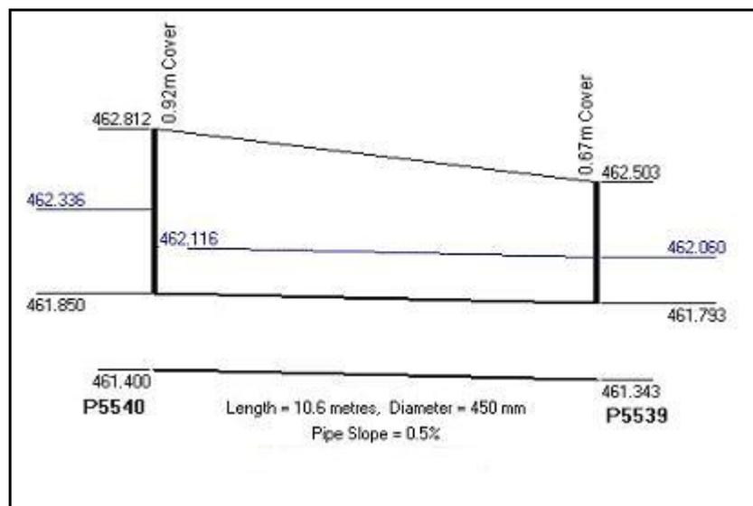
Figure 6-14 – Effect of a 450mm diameter reinforce concrete pipe on HGL
