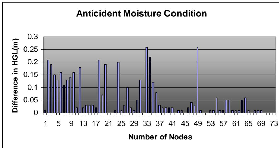
Figure 5-12 – Sensitivity of the model to varying antecedent moisture condition
