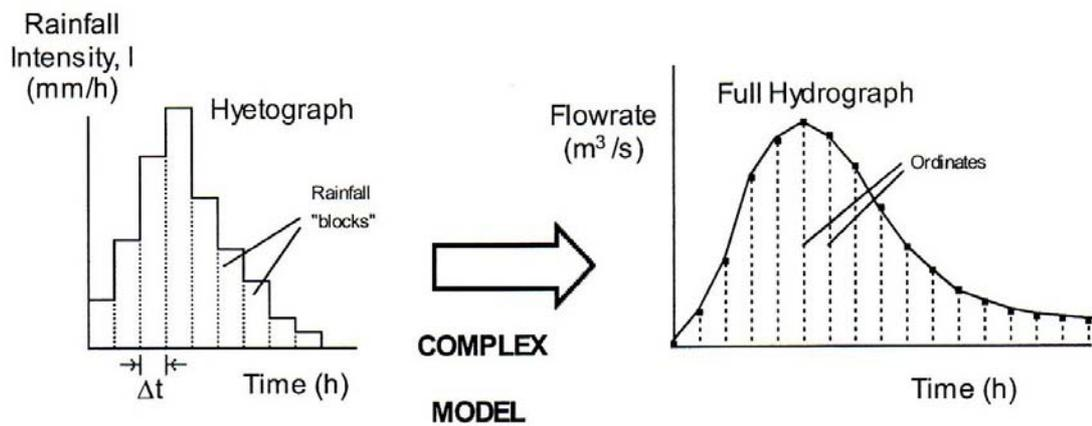
Figure 4-4 – Complex Rainfall Runoff Model (O’Loughlin & Stack 2002, p. 6.6)
