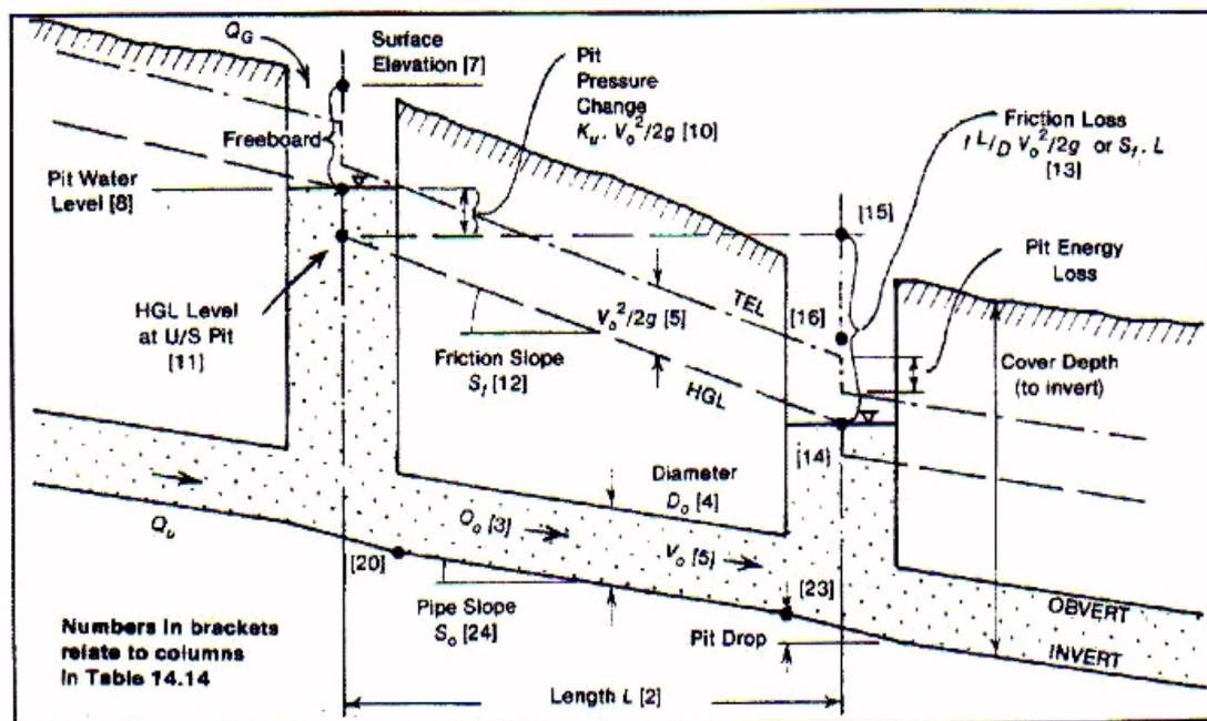
Figure 4-5 – Energy Level of Water Flowing in a Pipe (Engineers Australia 2001b, p. 42.)
