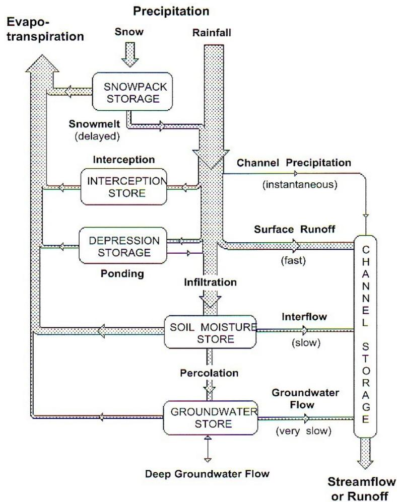
Figure 4-2 – The Rainfall-Runoff Process (O’Loughlin & Stack 2002, p. 6.5)
