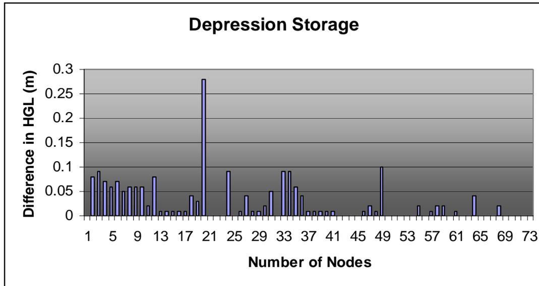
**Figure 5-14 – Sensitivity of the model to varying depression storage coefficients**
