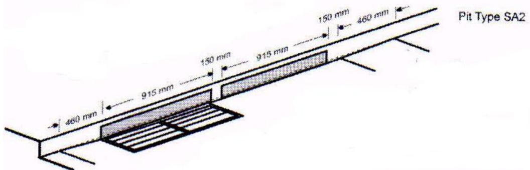
Figure 5-3 – NSW Road and Traffic Authority Inlets with depression Grates (O’Loughlin & Stack 2002, p. 6.35)
