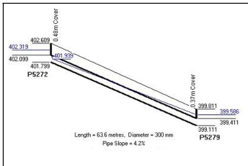
Figure 6-19 – Effect of pipe duplication on HGL
