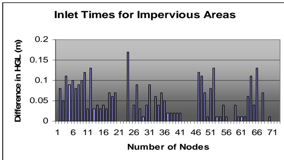
Figure 5-15 – Sensitivity of the model to varying inlet times, for impervious areas
