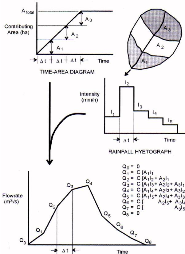
Figure 4-8 – Time-Area Calculations (O’Loughlin & Stack 2002, p. 6.10)
