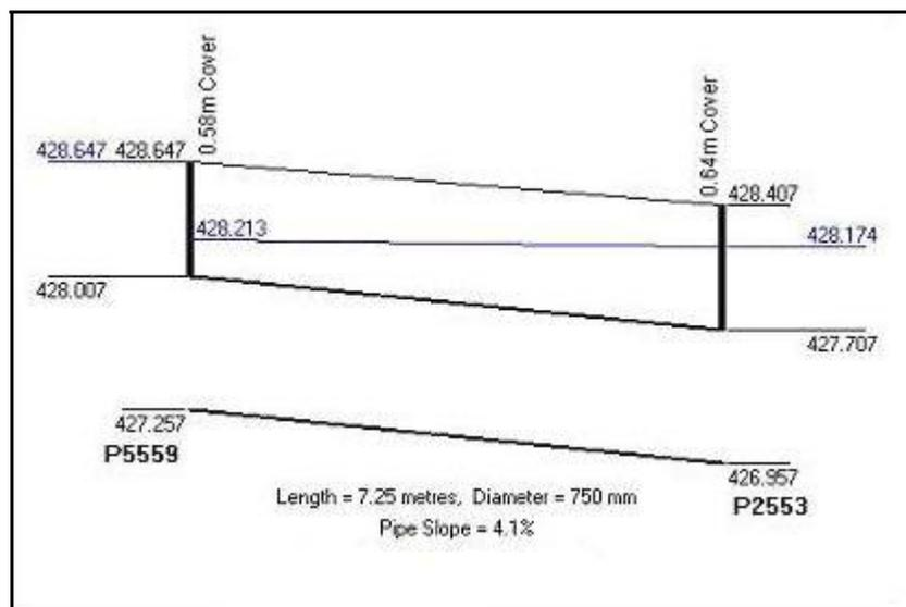
Figure 6-8 – Long Section of identified problem area
