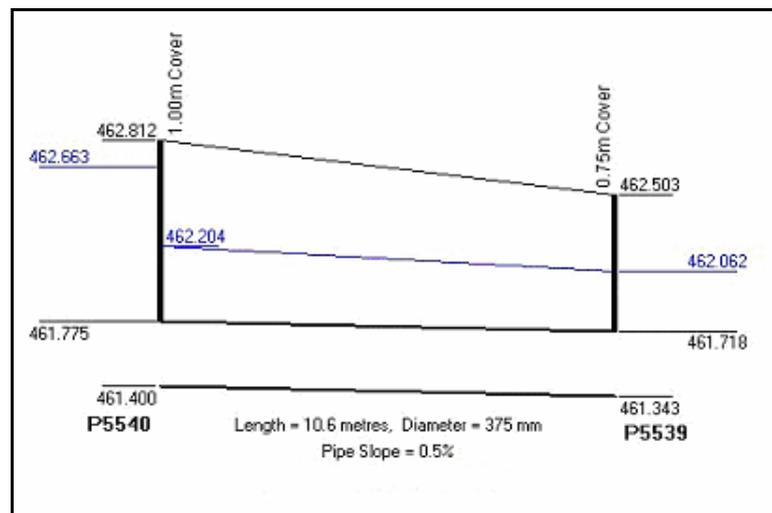
Figure 6-12 – Long Section of identified problem area
