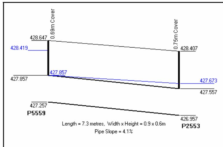
**Figure 6-9 –Effect of Reinforced Concrete Box Culvert on HGL**
