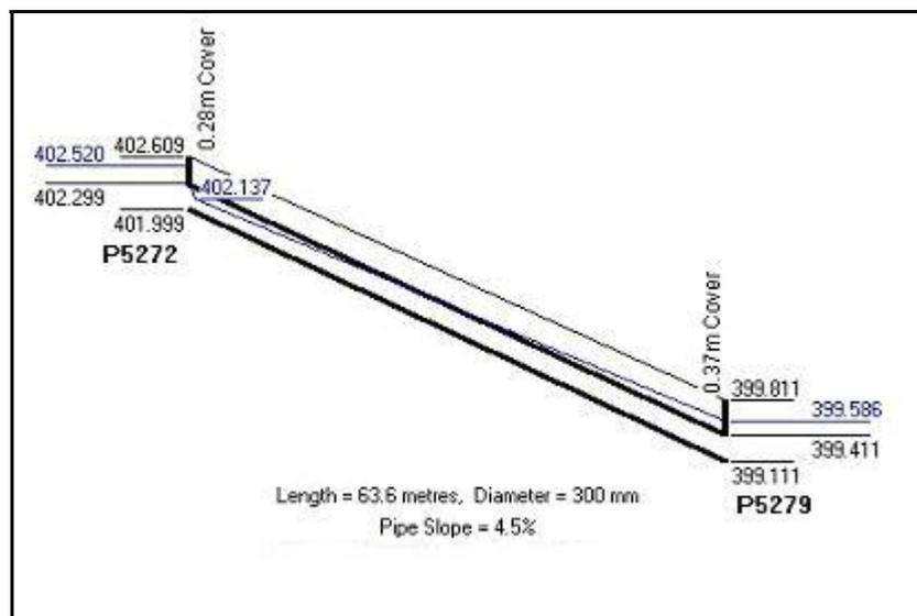
Figure 6-17 – Long Section of identified problem area
