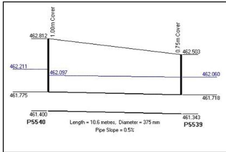
Figure 6-13 – Effect of pipe duplication on HGL
