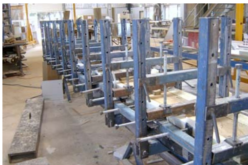
Figure 5.7 Clamps applied to entire length during gluing of centre section.
