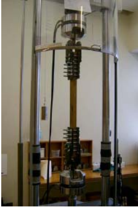
Figure 3.8 Tension test piece in MTS machine. testing
