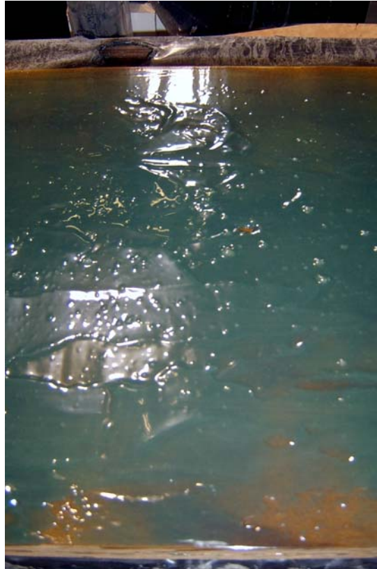
Figure 5.4 Glue after it has been spread on the LVL.
