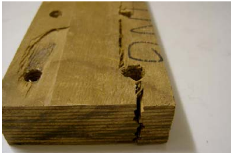
Figure 3.10 Shear failure of test piece through boltholes.
