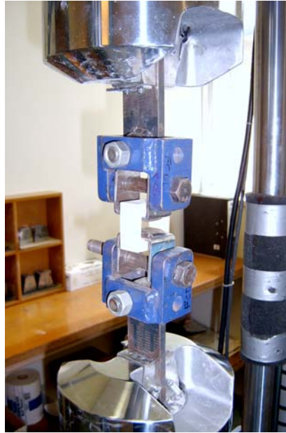
Figure 3.5 Cross tensile specimen during test.
