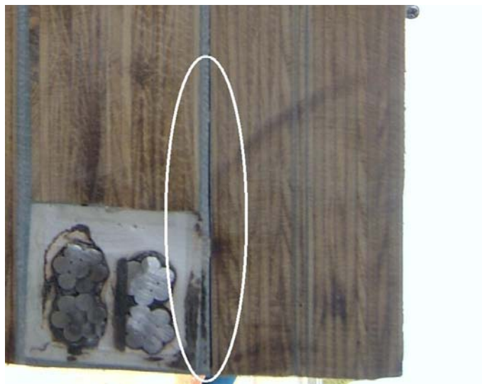
Figure 7.1 Break in bond between laminate and LVL.
