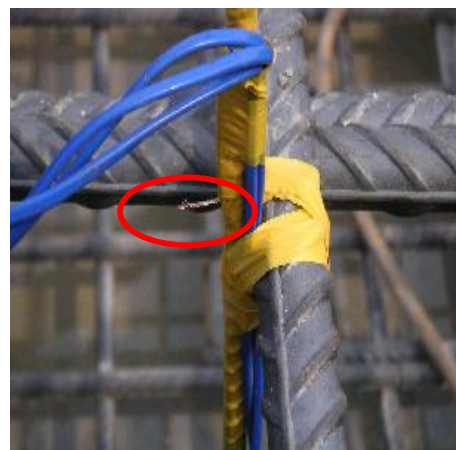
Figure 5.9: Make sure end of the thermocouple wires are in good condition
