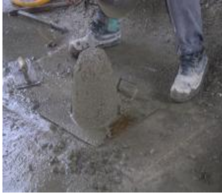
Figure 4.7: Lift the mould carefully
