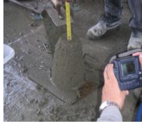
Figure 4.8: Measure the slump
