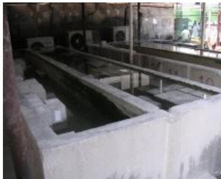
Figure 4.11: Cured in curing tank.
