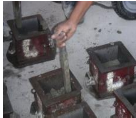
Figure 4.10: Fill in 3 layers and compact in standard manner (Compressive Strength test)
