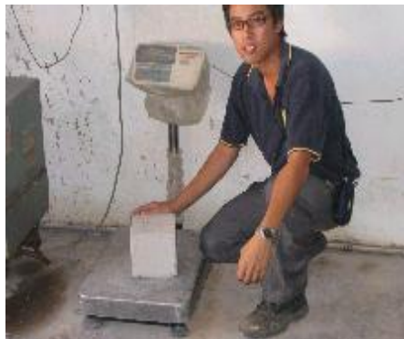
Figure 4.13: Measure the weight to make sure the densities are same.
