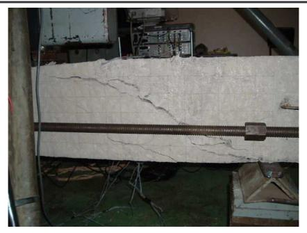
Figure 5.4: Failure Crack in Specimen B2
