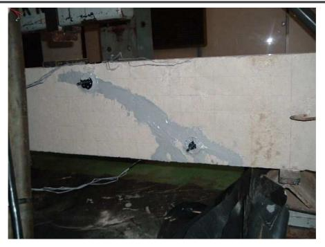
Figure 4.12: Sealing of Cracks Using Lokfix E
