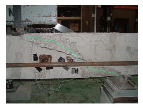
Figure 5.6: Failure Crack in Specimen B3
