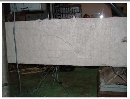
Figure 5.3: Initial Crack in Specimen B2
