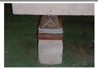
Figure 4.14: Test Beam Supports
