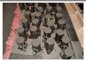
Figure 4.7: Freshly Cast Concrete Test Cylinders
