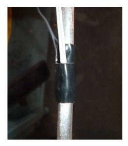
Figure 4.5: Steel Strain Gauge
