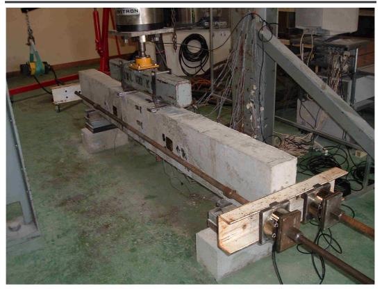
Figure 4.13: Test Configuration
