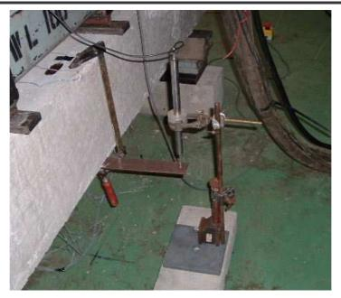
Figure 4.15: LVDT Measuring Midspan Deflection
