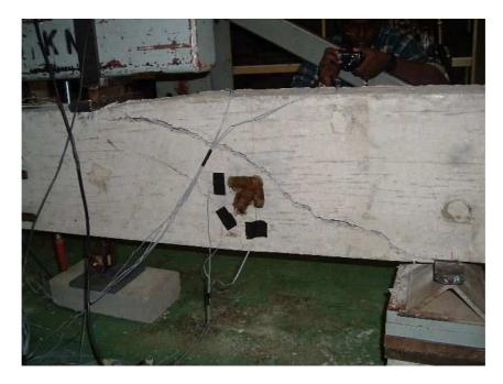
Figure 5.2: Failure Crack in Specimen B1
