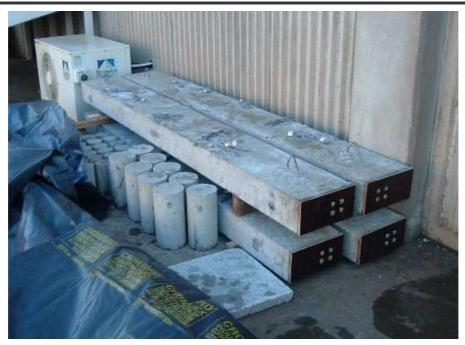
Figure 4.8: Beams and Test Cylinders after Stripping
