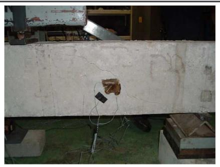
Figure 5.5: Initial Crack in Specimen B3
