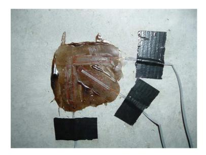
Figure 4.10: Strain Gauge Rosette
