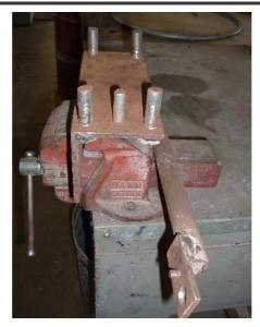
Figure 4.2: Bending Jig
