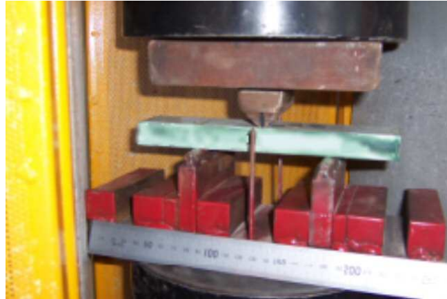
Figure 7.5: Sample Set-up in Test Jig and Machine
