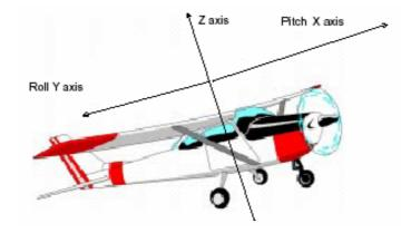
**Figure 10** The position of an aircraft can be described by roll and pitch combined with a compass bearing. Pitch is the position of the nose, either up or down, roll is the amount of tilt with respect to the wings, either left or right and is most commonly represented in the cockpit by a gimballed instrument. Course is derived from a magnetic compass and displayed with respect to magnetic north. Caruso (2004)
