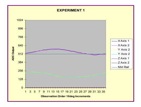
**Figure 39** Magnetic sensor output from x, y and z sensors with mid rail included. The graph shows substantial offset in the y sensor output with the z sensor response = 0. The experiment was conducted twice hence the data are labelled '1' and '2'. The difference between readings indicates the presence of noise in the circuit.
