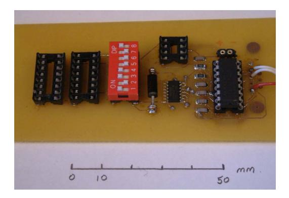
Figure 32 Communications Board No.1. Only a handful of components are necessary to provide the level switching to enable a PC to communicate with the microcontroller effectively.
