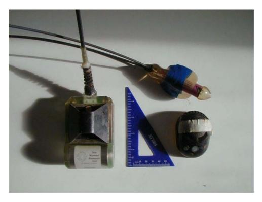
**Figure 4** SLTDR (L), VTDR (R) and VHF locator beacon (top R). The scientific payloads attached to seals are small in comparison to the target animal, an adult cow being in the order of 300kg and 2.5m in length.
