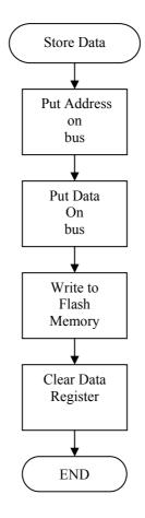
Figure 27 The writing of data to external memory requires precise sequential steps indicated in the flow chart.
