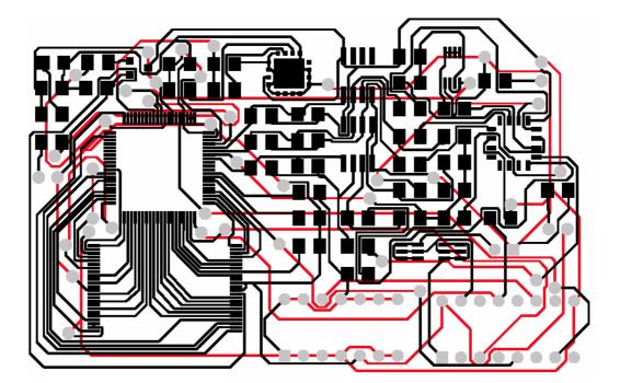
**Figure 29** PCB design of instrument using a two layer board. Top layer copper tracks and pads are presented in black, bottom layer in red, vias and through holes in grey. The actual dimension of the board is 77mm X 50mm.
