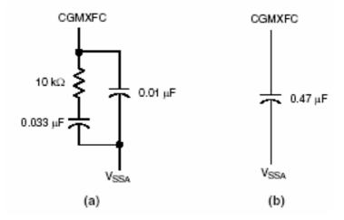
**Figure 16** Two options for external filtering was provided in data sheets, option (a) is for applications where stable PLL operation is important and option (b) is suggested for applications where stability is not critical as described in *MC68HC908LJ24 Data Sheet (2004)*.
