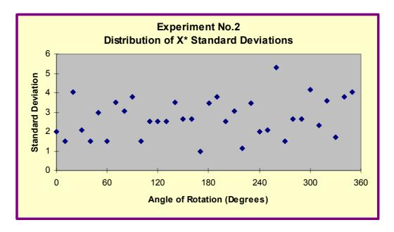
Figure 42 Each point represents the standard deviation of three x axis readings  $X^*$  taken at 10° increments over a full 360° rotation.
