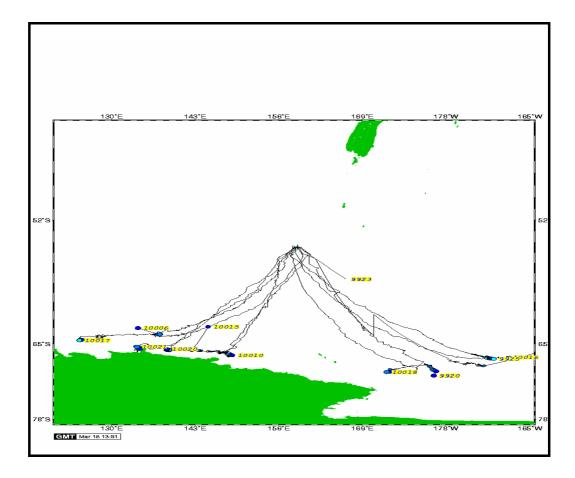
**Figure 7** Satellite tracks of deployed SLTDR units on 18 March 2005. Eleven tracks are recorded emanating from Macquarie Island (centre) extending well south towards Antarctica, a distance travelled of 2000km. New Zealand is visible at the top, Antarctica at the bottom of the frame with latitude and longitude inscribed on the boarders. Image courtesy of S. Wall.
