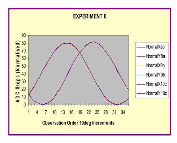
**Figure 44** Data obtained by the instrument with external sources of noise removed. The readings demonstrate the quality of data obtainable and offer an insight into the repeatability of the instrument. The improvement in data quality is evident when compared with Figure 41.
