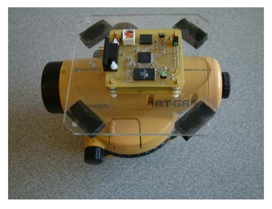
Figure E. 1 Topcon Surveyors Level with instrument in position prior to securing using cable ties and insulating tape.
