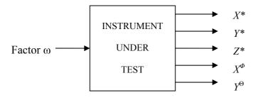
**Figure 37** The basic concept of a factorial design, in this case the system is reduced to one factor and five response variables. The assumption made under this design is that the factors and response variables are independent of each other.
