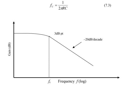
**Figure 33** Single Pole low pass filter used to remove switched capacitor noise components from accelerometer. Frequency components of noise above the corner frequency of 1600Hz are attenuated by the filter at a rate of -20dB/decade.
