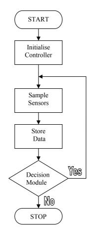
**Figure 24** The top down approach promotes a modular design capable of modification, thereby aiding both subsequent optimisation and maintenance. Each of the main functional modules are further exploded into sub modules before structured programming is applied to build the code sections.
