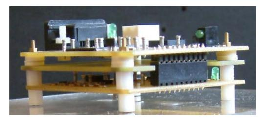
Figure 34 Prototype No.2 The ground plane is visible between the upper data logger and the lower sensor board and is constructed of unetched copper PCB cut to size.
