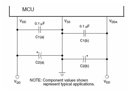
**Figure 17** Power supply bypassing recommended to reduce noise effects on the microcontroller. MC68HC908LJ24 Data Sheet (2004). Copyright material owned by Freescale Semiconductor, Inc. used with permission, 2005
