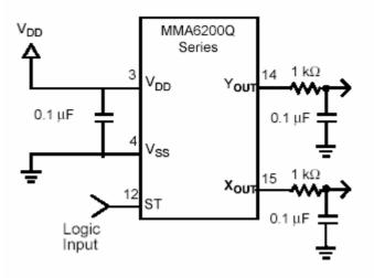
**Figure 22** The accelerometer IC samples the internal micro machined sensors at a rate of 52kHz. The output filter circuit of  $1k\Omega$  and 0.1uF removes the noise generated from the internal switched capacitor filter circuit.  $\pm 10g$  Duel Axis Micromachined Accelerometer (2004)
