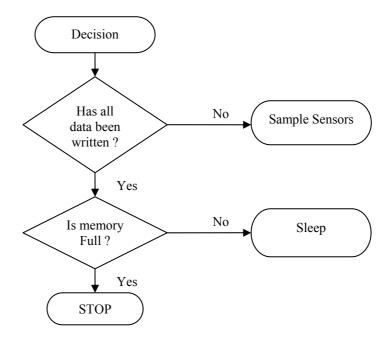
Figure 28 The decision to continue recording data is critical to prevent overwriting earlier data should the memory address exceed 3F FF FF.
