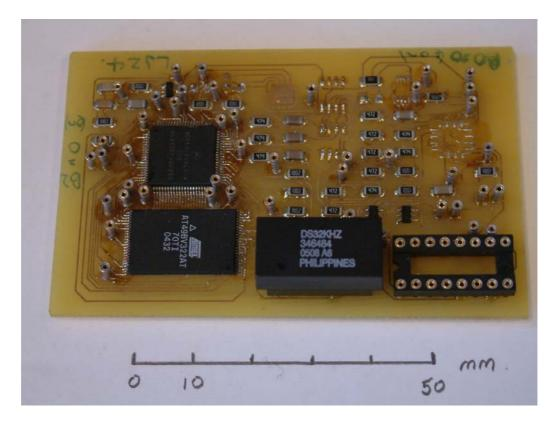
**Figure 31** Prototype No.1. Using surface mounted components in the design made the instrument compact. To further miniaturise the device using decreased track widths and clearances, commercial PCB manufacturing would be required. Several footprints are unpopulated as the components were robbed for the construction of the second prototype.
