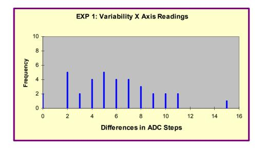
Figure 40 The variability between x axis trials is substantial, the average variation is 5.8 ADC steps, this represents a voltage difference of approximately 20mV and the worst case is 15 ADC steps which is equivalent to around 52mV.
