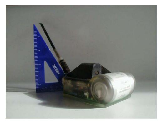
**Figure 3** The Series 7000 SLTDR uses the Argos satellite system to relay data from a surfaced seal and provides researchers with close to real time geographical positioning via a secure web address generated at the Sea Mammal Research Unit at the University of StAndrews, Scotland. Time, depth and velocity is also recorded on board and downloaded when the unit is recovered.
