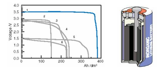
**Figure 8** Discharge curves of different battery chemistries listed in Table 3. The curves are recorded at 25°C at the 1000 hour rate. A cut away diagram of a lithium battery shows the structural elements. Data Sheet: Sonnenschein LBT Brochure (2003)
