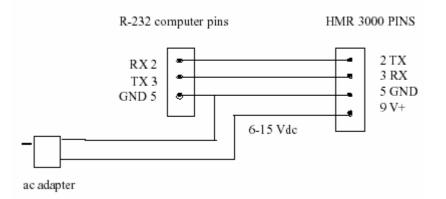
Figure 12 Schematic of connecting cable to provide power and communications lines between the HMR3000 and a PC. *DCM Users Guide (2004)*
