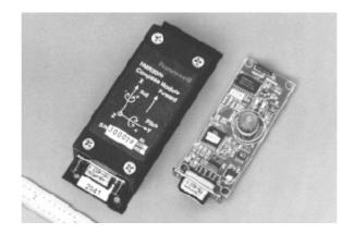
**Figure 11** The HMR3000 provides compassing information by combining a two axis magnetoresistive sensor in conjunction with a two axis electrolytic tilt sensor. Honeywell Australia provided a demonstration unit for evaluation purposes. HMR3000 DCM (2004).
