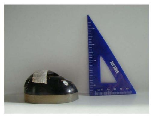
**Figure 2**. The Wildlife Computers MK8 VTDR is configured to record depth, light level, temperature and velocity at 30 second intervals and stores the information using 16MB of memory for later retrieval.
