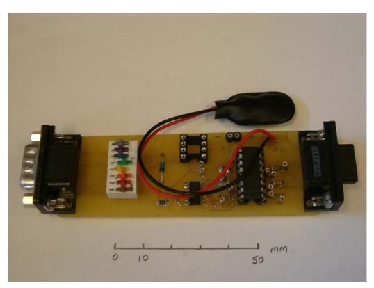
**Figure 36** Communications Board, second prototype. The communications board is a simple arrangement using DB9 connectors at either end of the board. The connectors are polarised to prevent incorrect connection.
