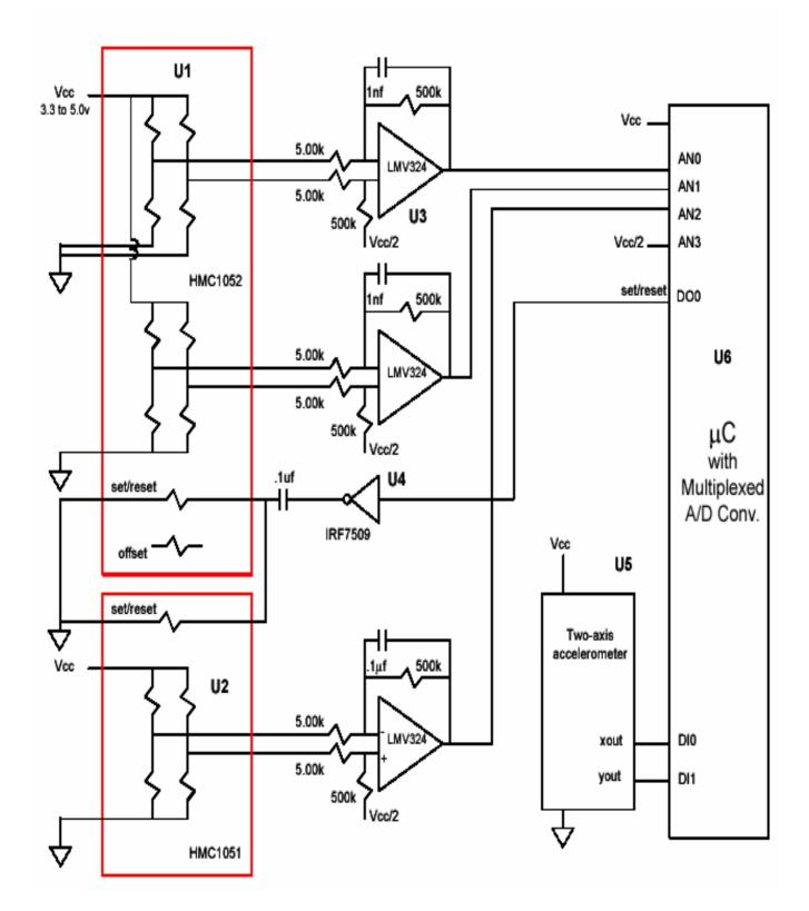
Figure 20 Each of the bridge networks is arranged to represent one axis of magnetic detection, either x, y or z. The output of the bridge provides the input to the operational amplifier stage then directly into an analogue to digital converter. *1,2 and 3 Axis Magnetic Sensors (2004)*
