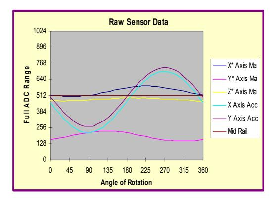
**Figure 45** Collating ADC inputs graphically demonstrates the effectiveness of the design. Offset is evident in all sensors, provided the sensors do not make excursions too close to the top or bottom rail clipping will not occur and the data will be complete.
