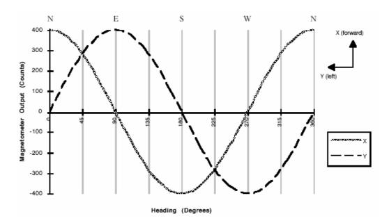
Figure 13 Hx and Hy Magnetometer readings for different compass headings. A full explanation is provided in *Compass Heading using Magnetometers AN203 (2004)*.
