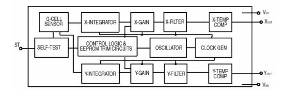
**Figure 14** Functional block diagram of accelerometer showing the complex stages within the integrated circuit which result in compact sensing solutions requiring little external biasing circuitry.  $\pm 10$ g Duel Axis Micromachined Accelerometer (2004).
