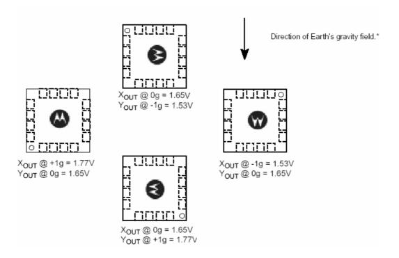
**Figure 15** Anticipated output of accelerometer to the effect of gravity in a static application. When the component is positioned as shown the X and Y output voltages represent a 1g output.  $\pm 10g$  Duel Axis Micromachined Accelerometer (2004).
