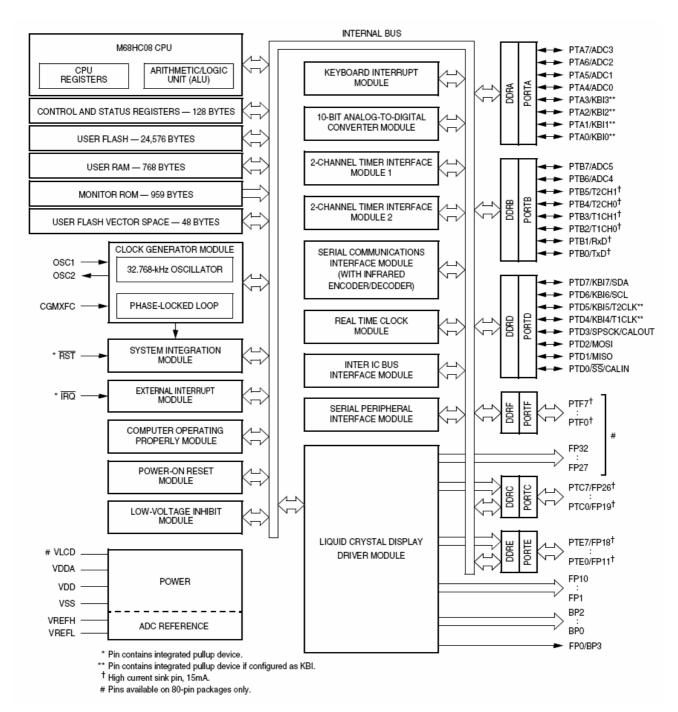
The input/output pins are arranged as ports with registers correspondingly assigned and shown in Figure 18.
