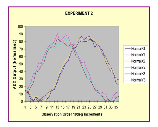
**Figure 41** Variation between three experimental runs of  $X^*$  and  $Y^*$  magnetic ADC readings. The general shape is similar to Figure 13 showing the 90° phase difference between  $X^*$  and  $Y^*$  magnetic readings and the general sinusoidal waveform in quadrature as expected.
