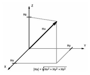
**Figure 46** Diagrammatic representation of the components of magnetic field detected by the instrument and the relationship to the horizontal plane. AN200 (1996)
