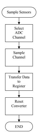
Figure 26 The ADC transforms the output from the sensor circuits into a digital representation of the voltage so that it can be stored in the flash memory for later retrieval.
