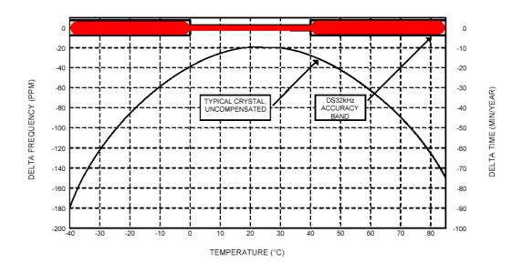
**Figure 9** The DS32kHz produces a temperature compensated output of 32.768kz. The oscillator corresponds with the specified frequency needed for the RTC in the selected MC68HC908LJ24 microcontroller. DS32Khz TCXO (2004).
