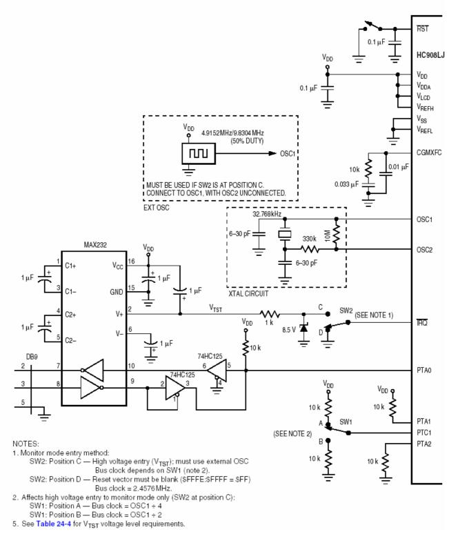
**Figure 23** Conditions required to enter Monitor Mode as outlined in MC68HC908LJ24 Data Sheet (2004). Copyright material owned by Freescale Semiconductor, Inc. used with permission, 2005.
