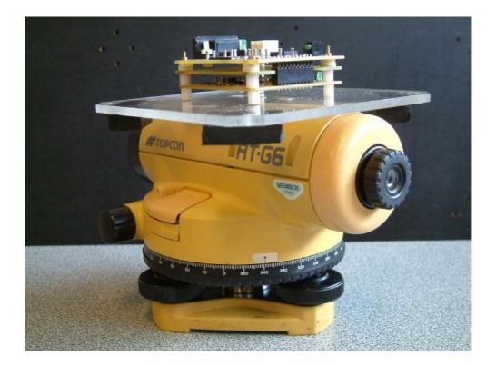
Figure 38 Attaching the instrument to the surveyors sight permitted accurate rotation, strengthening the repeatability of the experimental method. The graduation ring seen at the bottom of the sight is marked with  $1^{\circ}$  increments with experimental measurements taken at  $10^{\circ}$  intervals.
