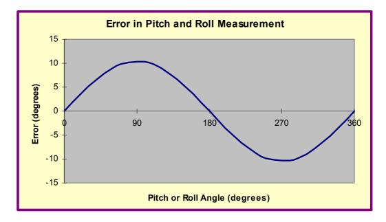
**Figure** 47 The error in pitch and roll clearly shows the device is more accurate for small values of tilt and increases to a maximum at  $\pm 90^{\circ}$  tilt.
