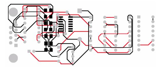
**Figure 30** PCB design of Communications Interface board using a two layer board. The dimension of the board is 90mm X 33mm.
