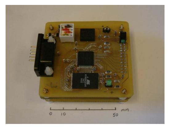
**Figure 35** Instrument Prototype No.2. The second prototype is constructed of two PCBs connected by a pin header. To reduce noise a ground plane is also inserted between upper and lower boards.
