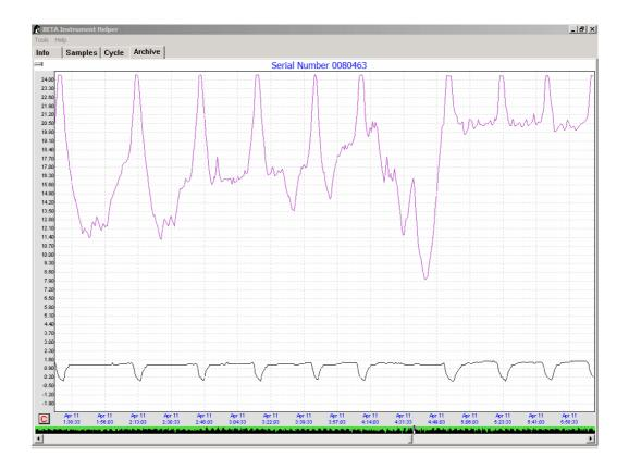
**Figure 6** VTDR data. The screenshot frame represents 9 dives on the 11<sup>th</sup> April 2004 at 4am. The water temperature is plotted as the lower curve towards the bottom of the frame. By superimposing the dive profile, upper curve, on the same frame, the relationship between depth and temperature can be explored. Data courtesy of Dr M Hindell.
