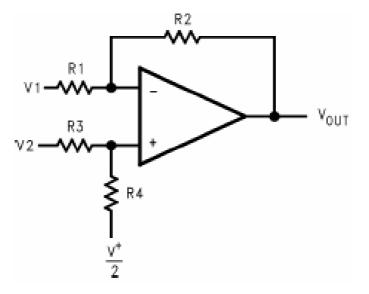
**Figure 21** Operational amplifier used as a difference amplifier to increase the output of the magnetoresistive bridge circuit. In this application R1=R3=4.7k and R2=R4=470k. *1,2 and 3 Axis Magnetic Sensors (2004)*.
