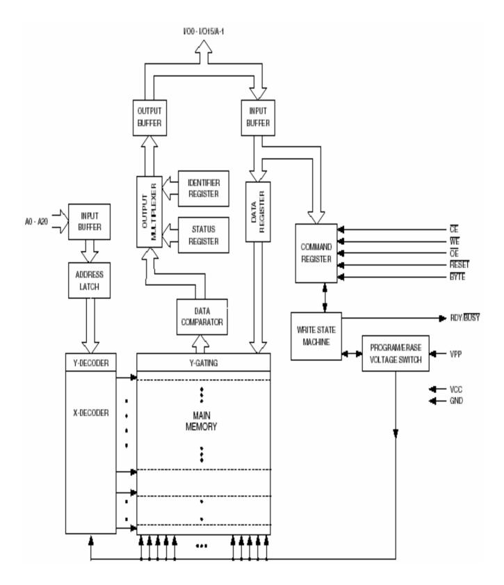
Figure 19 The AT49BV322AT provides a choice of 16bit word or 8 bit byte data bus width, for this application the 8 bit byte option was selected. *32Mbit Flash Memory (2004)*.
