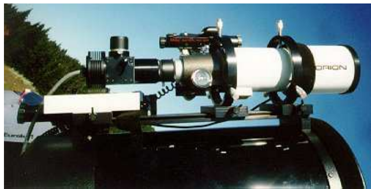
Figure 4.2: ST-4 CCD camera (pictured to the left of the image) attached to a telescope, how it is designed to be used (Haworth 2003).
