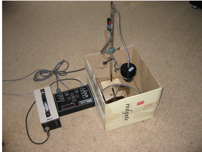
Figure 5.6: The setup of the ST-4 and mirror to determine the appropriate height the camera should be placed above the mirror plane.
