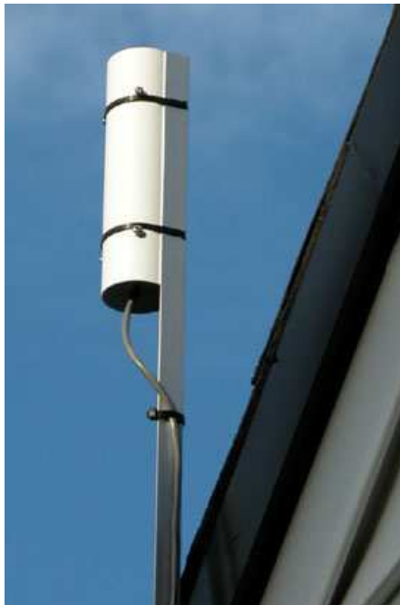
Figure 2.2: Boltwood Cloud Sensor (Boltwood 2004).
