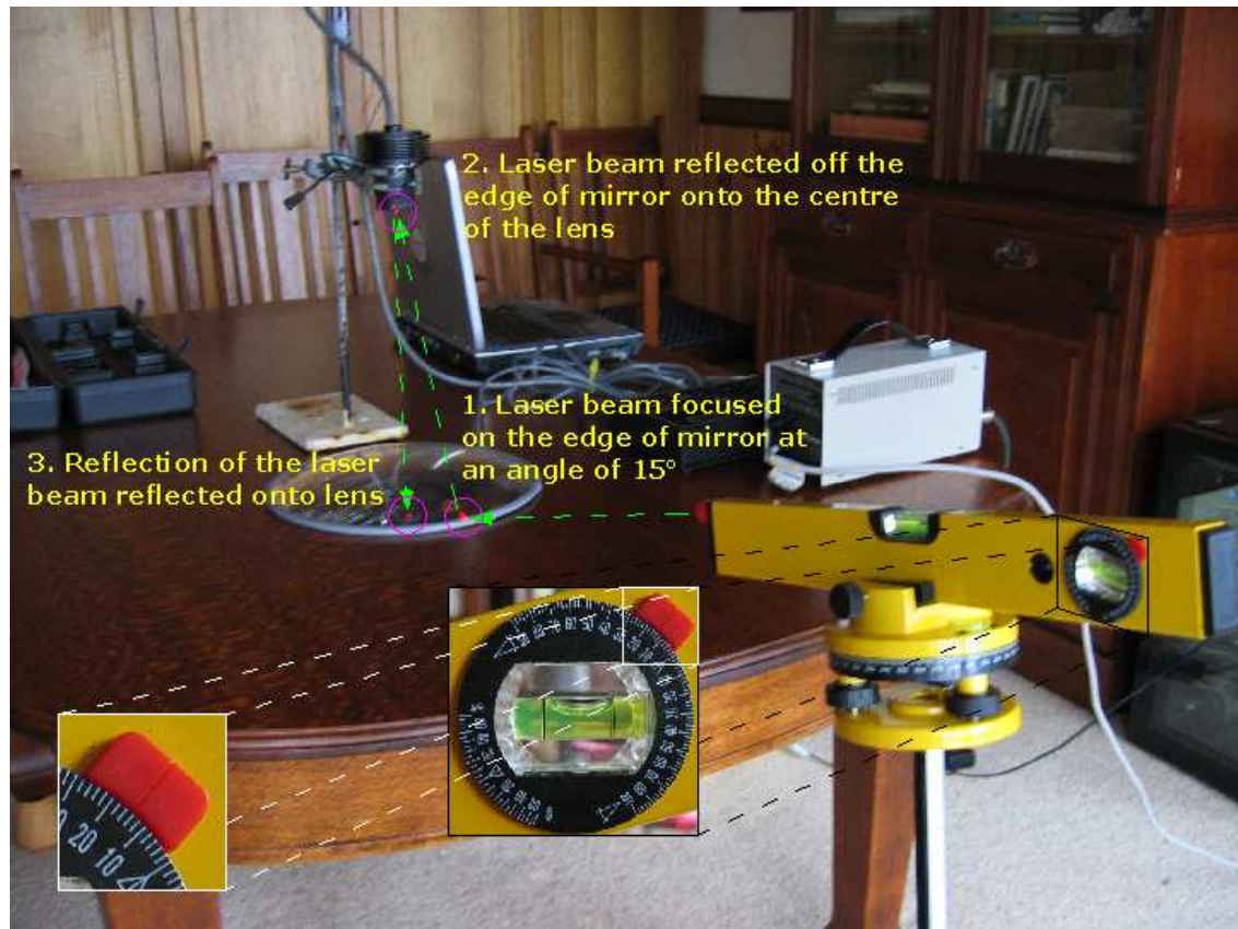
Figure 5.8: System setup to verify the viewing angle of the sky would be approximately 155^\circ if the ST-4 is placed 27cm above the base of the mirror. The laser is focused on the edge of the mirror at an angle of 15^\circ off the horizon, and is reflected directly onto the centre of the lens.
