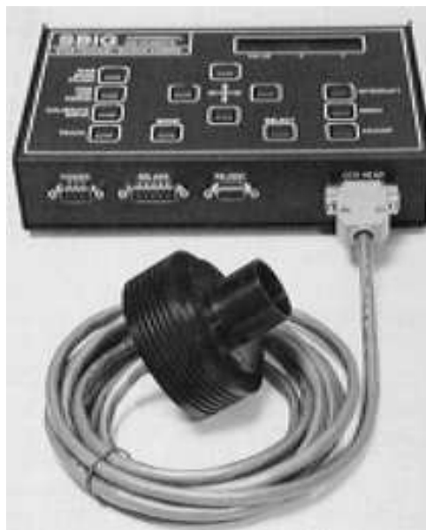
Figure 4.1: ST-4 CCD camera and microcontroller (SBIG 2005).
