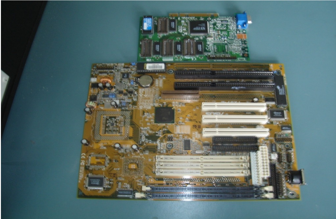
Figure 5-1A: shows the motherboard and the daughter board of the PC
