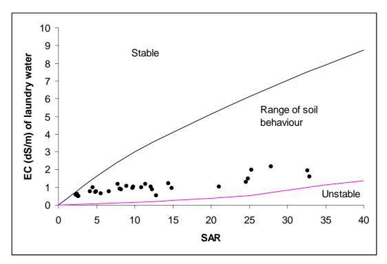
Figure 7. 2: Comparison of laundry water quality in this project with a permeability threshold values for soil types as a function of SAR and EC (adapted from Myers et al. 1999).
