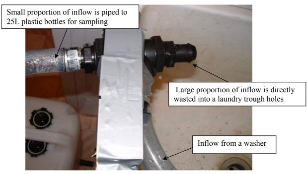
Figure E2: Top view of the flow splitting device after installed
