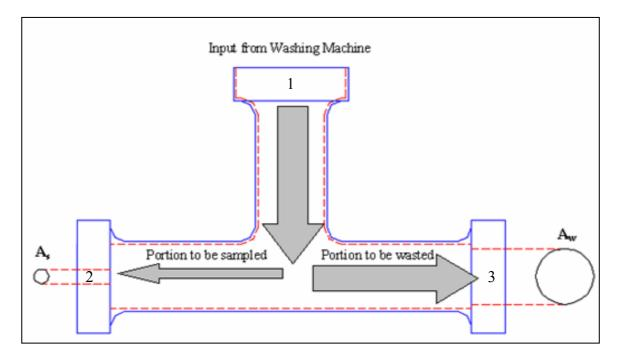
Figure 4. 8: The T-sectioned flow splitting unit with different outlet diameters
