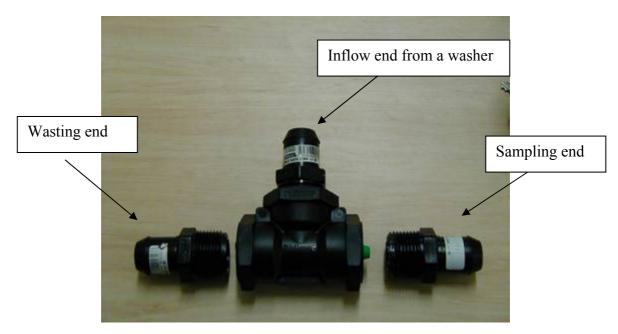
Figure F3: Positions of parts before assemblage
