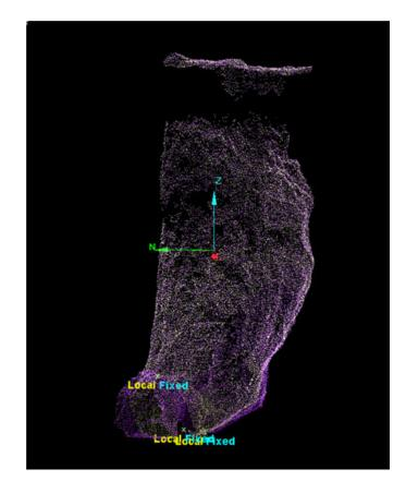
Figure 3.11: Voidworks screen capture of 3597 stope showing matching point pair registration
