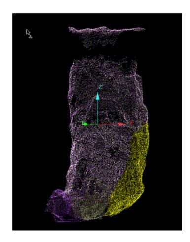
Figure 4.2: Voidworks screen capture of 3597 stope. The yellow points show the area of shadow captured by realigning the scanner on the CMS trolley.
