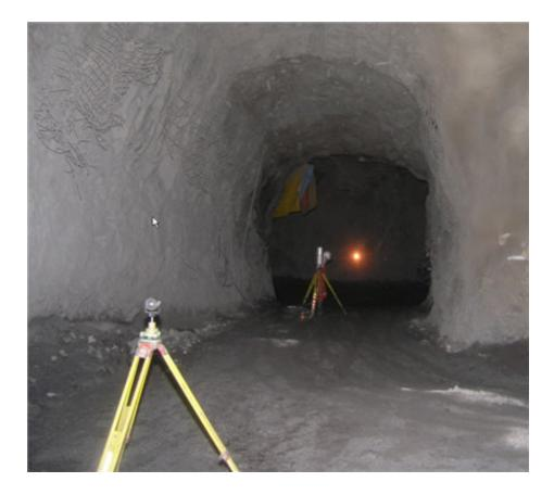
Figure 3.9: Photograph of the drive survey on 280 Level performed with the scanner.
