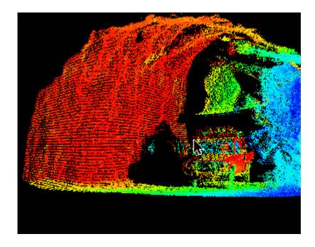
Figure 4.8: Voidworks screen capture of the extent of the data capture. Notice the survey vehicle clearly visible.
