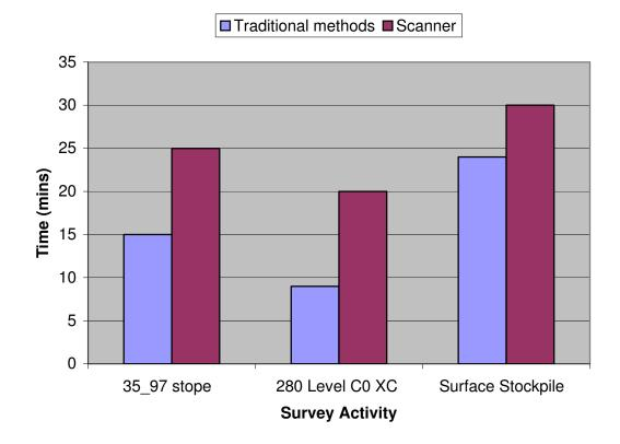
Figure 4.1: Time taken to set up instruments in order to start surveying
