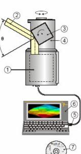
The range finder electronics (1) of the 3D scanner *RIEGL* LMS-Z210i is optimized in order to meet the requirements of high speed scanning (fast laser repetition rate, fast signal processing, and high speed data interface).
