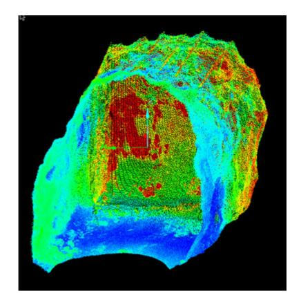
Figure 4.14: Voidworks screen capture of the 280 Level drive showing different reflectance values
