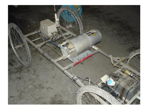
Figure 3.6 Scanner attached to the CMS trolley in the lateral position
