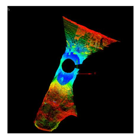
Figure 4.3: Voidworks screen capture of the scanner drive survey showing shadow areas above and below the scanner.
