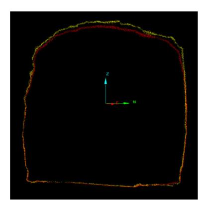
Figure 4.13: Voidworks screen capture of a cross-section of 280 Level CO XC before and after fibrecreting.
