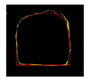
Figure 4.11: Voidworks screen capture of a cross-section of the two solid models of 280 Level C0 XC. The scanner model is gold and the total station model is red
