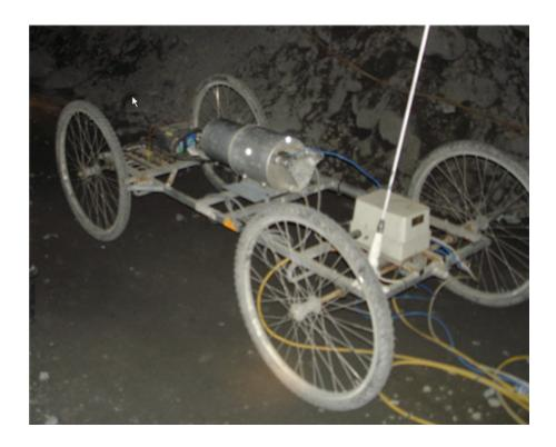
Figure 3.7 Scanner attached to the CMS trolley in the longitudinal position
