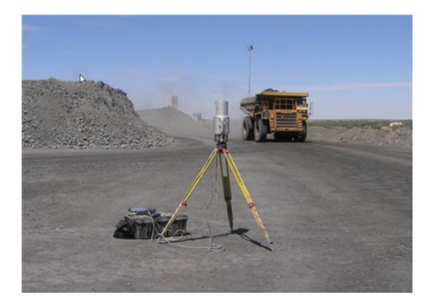
Figure 3.10: Photograph of the scanner set up on the ROM (Run of Mine) stockpile
