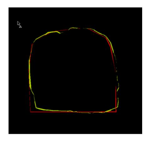
Figure 4.10: Voidworks screen capture of a cross-section of the two solid models of 280 Level C0 XC. The scanner model is gold and the total station model is red
