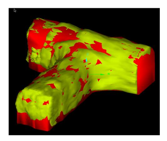
Figure 4.7: Voidworks screen capture of solid models of 280 Level drive surveys. The scanner data model is gold and the total station data is red.
