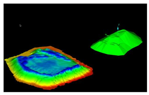
Figure 4.12: Voidworks screen capture of a surface stockpile. Notice the difference in detail between stockpiles
