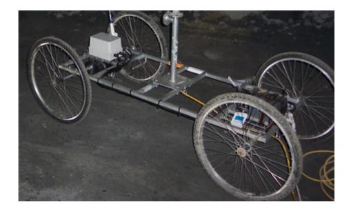
See Figure 3.8: Photograph of CMS trolley with the scanner base plate removed and the CMS arm replaced
