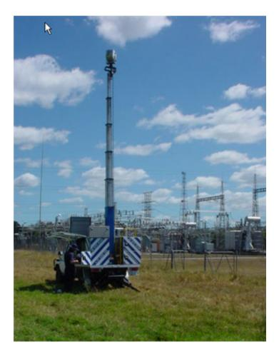
Figure 5.1: Photograph of North Surveys survey vehicle with a scanner on the top of the boom.
