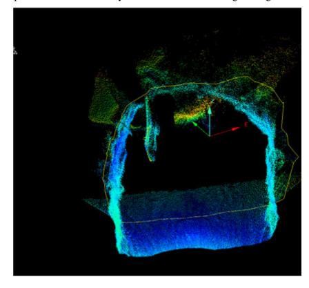
Figure 4.9: Voidworks screen capture of the loop wrap function. This function creates a polygon around the outermost points selected.
