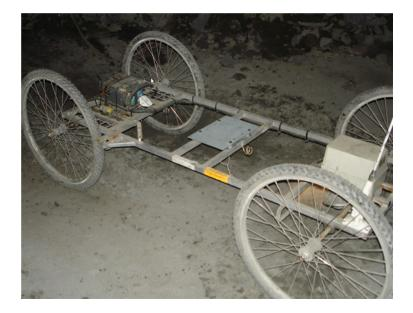
Figure 3.5: Photograph of the CMS trolley with scanner base plate attached
