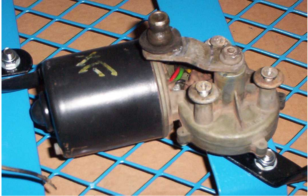
Figure 25 - The ‘windscreen wiper’ steering actuator to be used in the project
