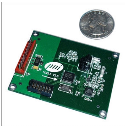
Figure 19 - The TCM 2.5 Compass Module by PNI Corp.
