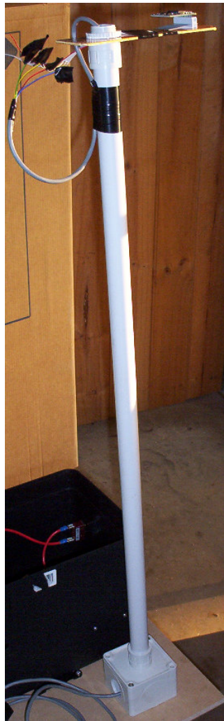
Figure 40 – The 850mm PVC mast to hold compass clear of interference.
