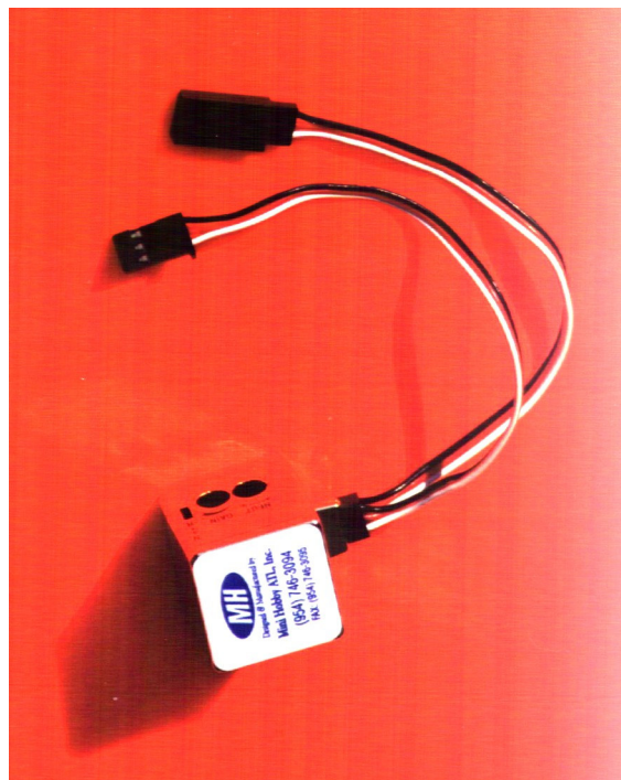
Figure 15 – mini gyroscope as used in hobby model aeroplanes
