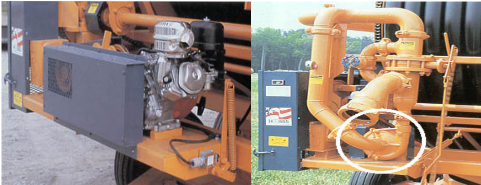
Figure 2.13 and 2.14 Picture of Auxiliary Engine and Turbine Drive Mechanism Attached to Travelling Irrigators
