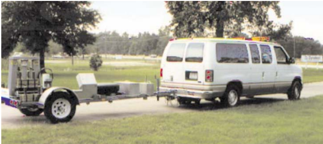
Figure 3.3: Falling Weight Deflectometer [8]
