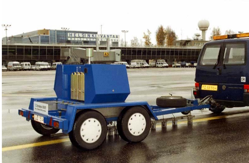
Figure 3.4: Heavy Weight Deflectometer [8]
