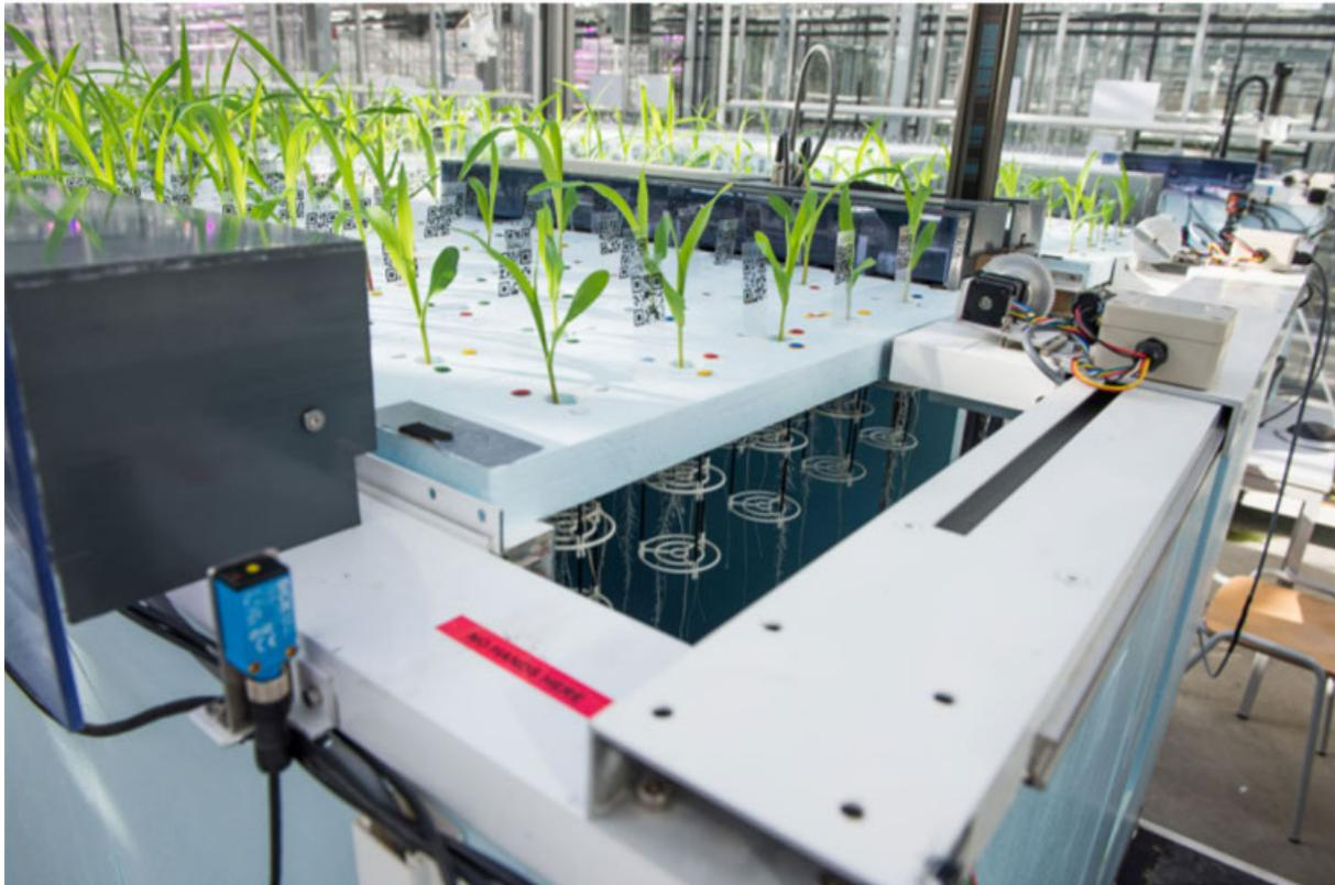
Figure 1.2: The aeroponic high-throughput phenotyping platform which was used in the collection of the plant root tip data. Roots dangle freely and can easily be misted with water/nutrients. The camera can run underneath the platform to take many high quality images of the plant root systems in a non-destructive manner.
