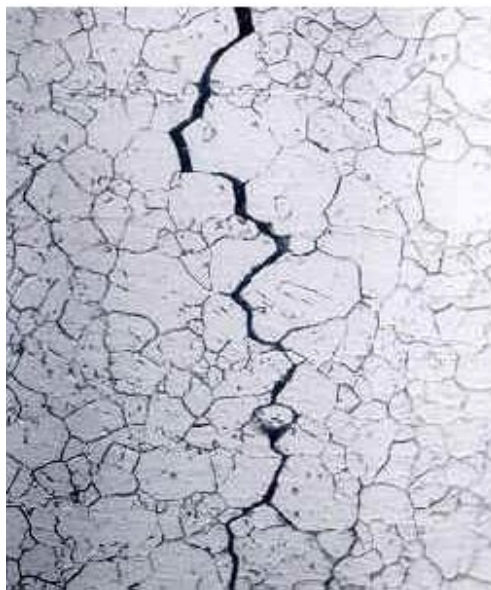
Figure 2.20: Intergranular SCC on grain boundaries (Stress corrosion cracking 2021)
