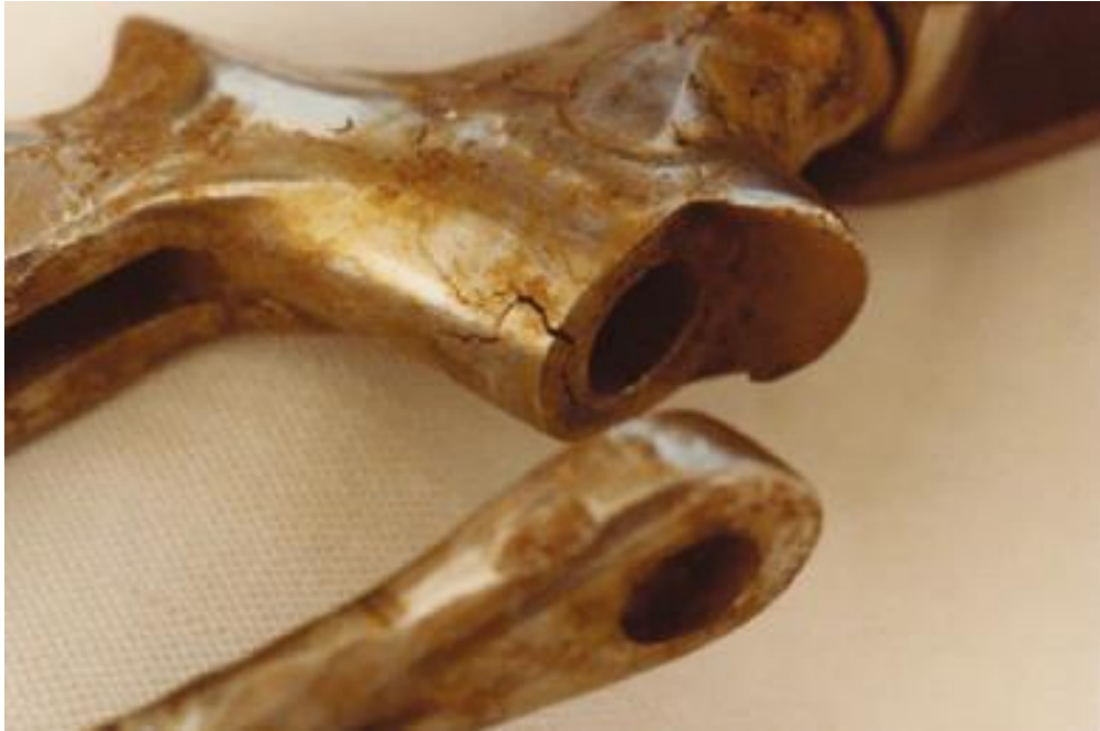
Figure 2.19: Example of SCC related failure of a carbon steel (Pedefferri 2018)
