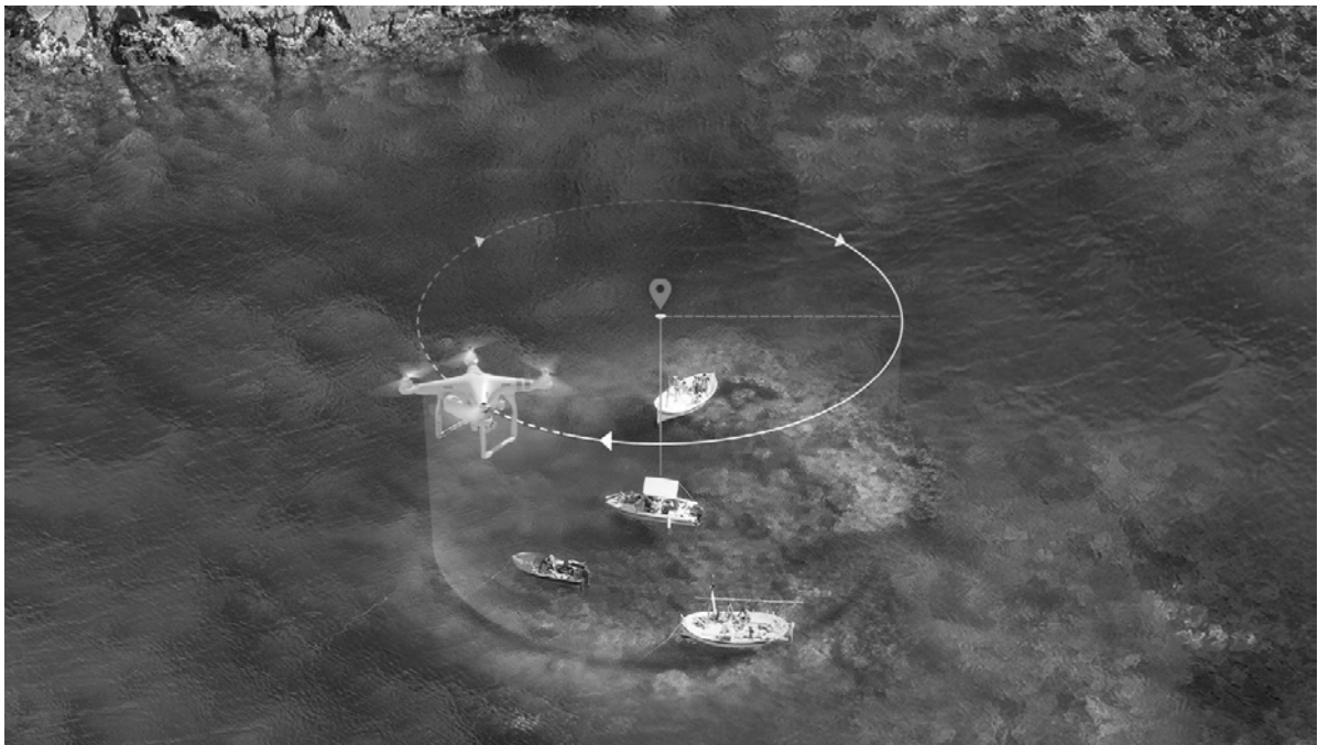
Figure 3. Point of Interest Flight Mode - Drone Automatically Revolves Around Designated Target (DJI 2015).
