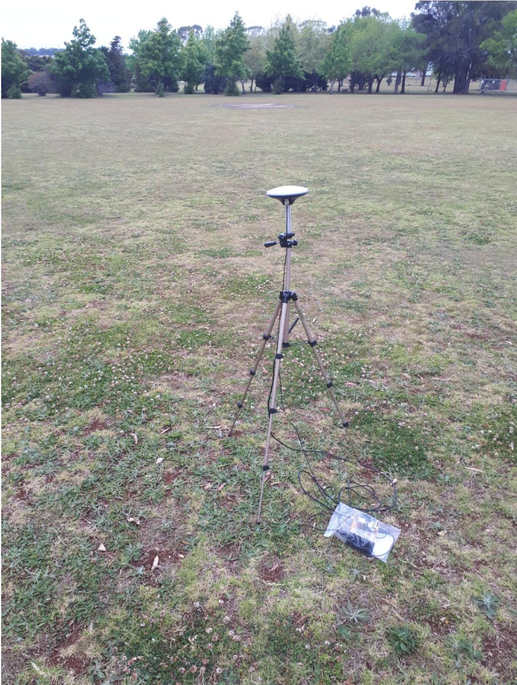
Figure 3.3: Base station deployed
