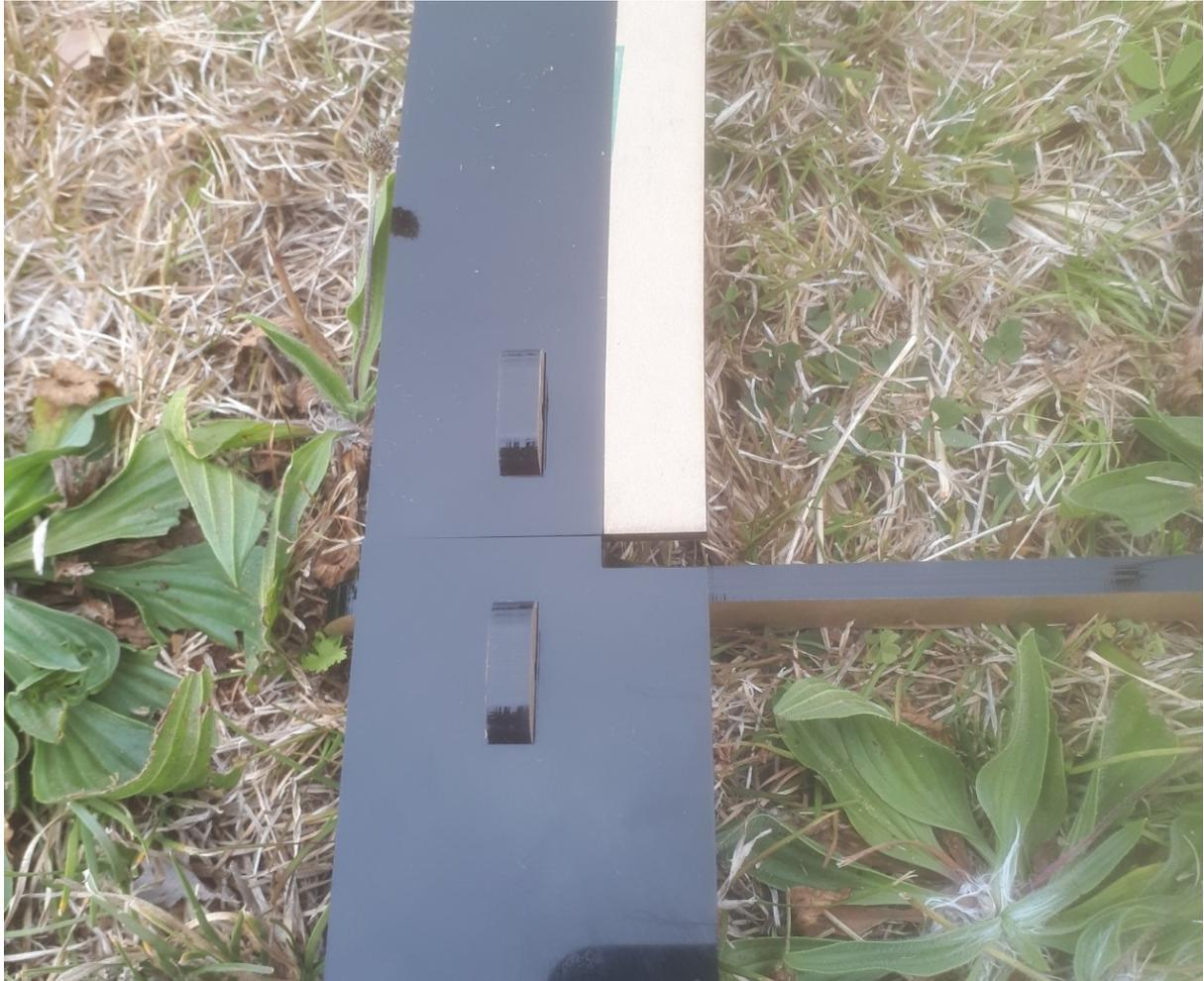
Figure 4.5: The cut slot at the end of straight track segment.
