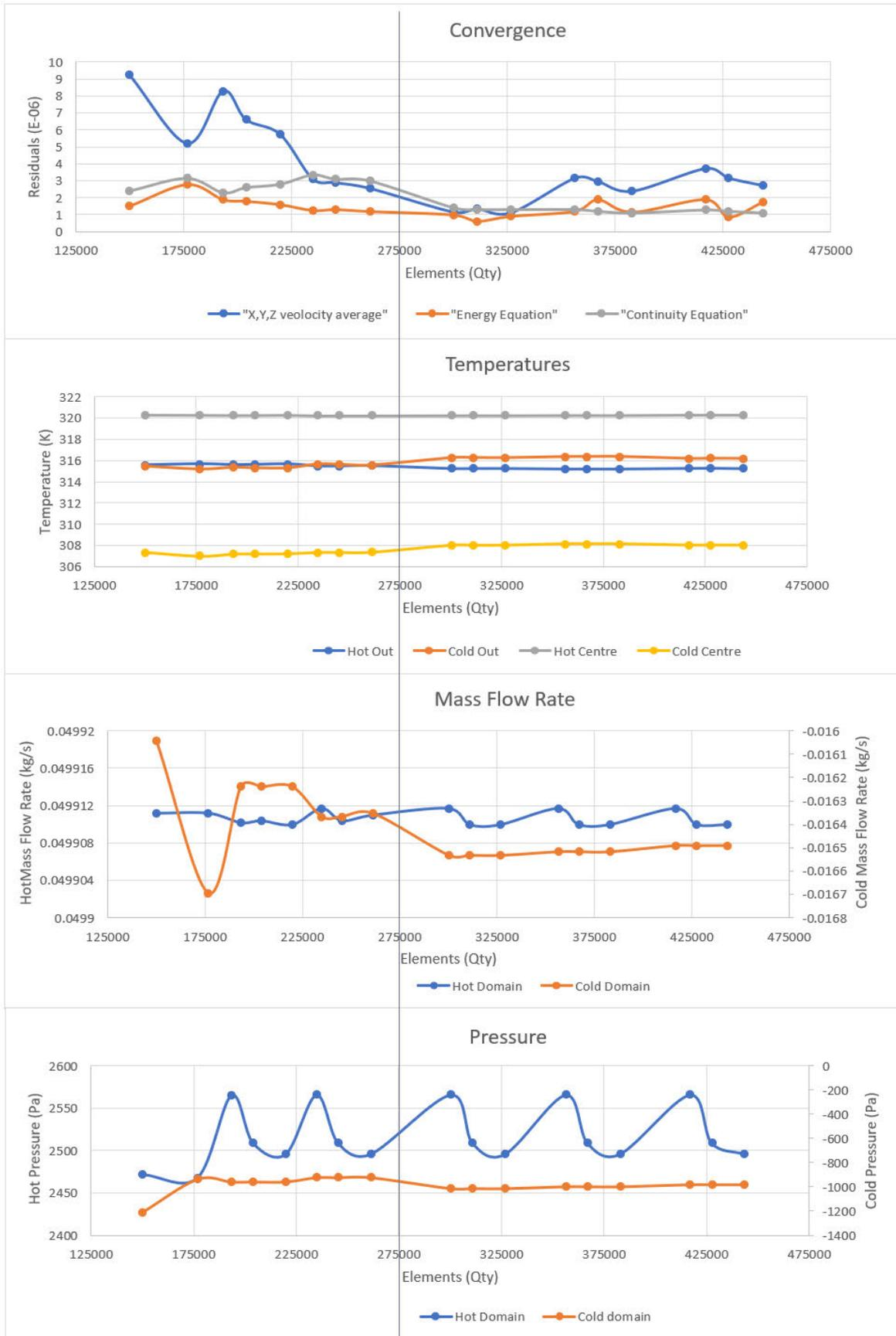
Figure 4-20: Mesh Independence Study results showing stability after approximately 275,000 elements.
