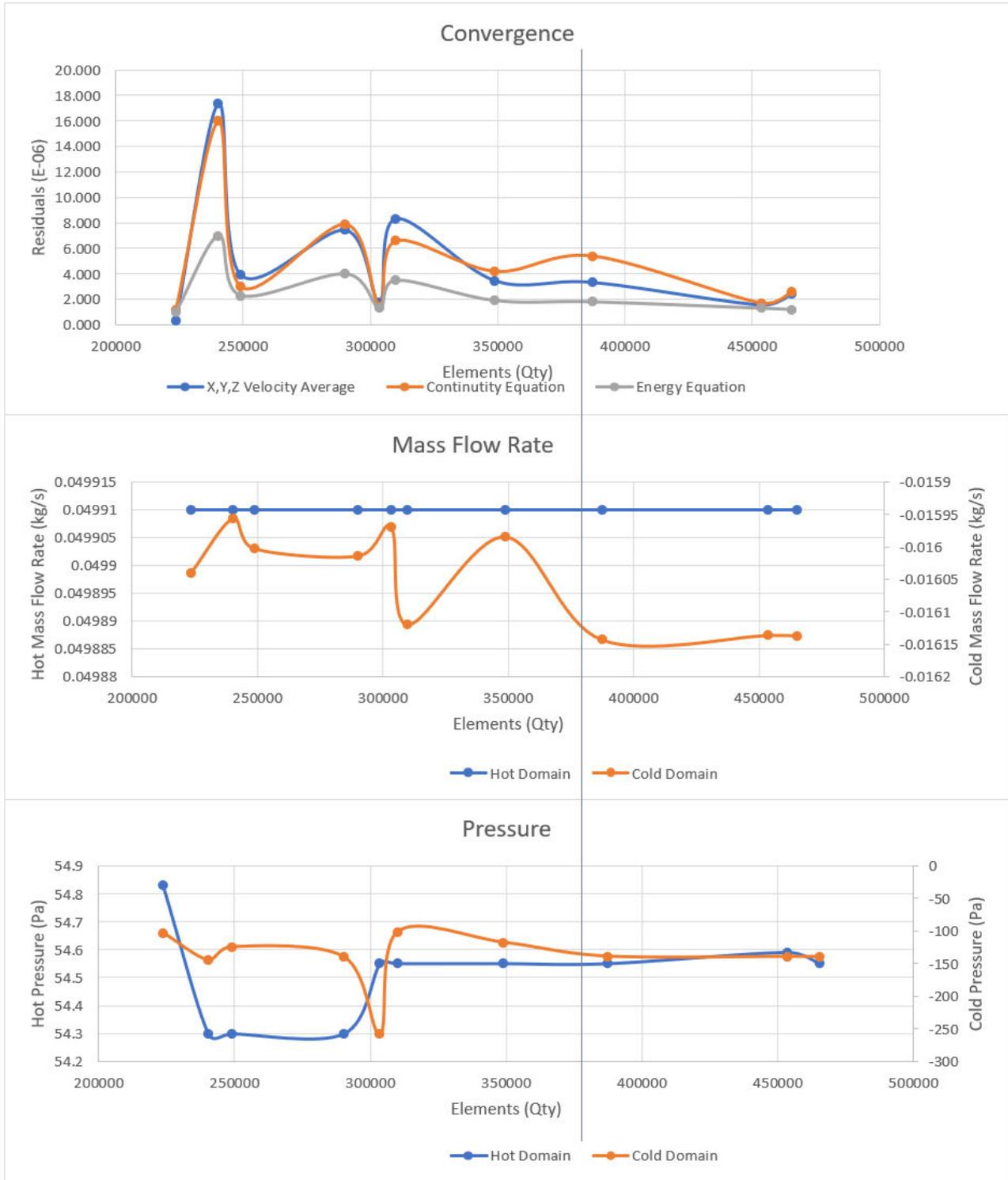
Figure 4-57: Mesh independence study results showing stability after approximately 375,000 elements.
