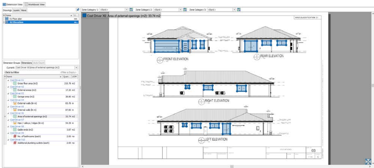
Figure 37 – External opening measured example
