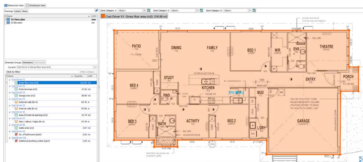
Figure 32 – Gross floor area measured example
