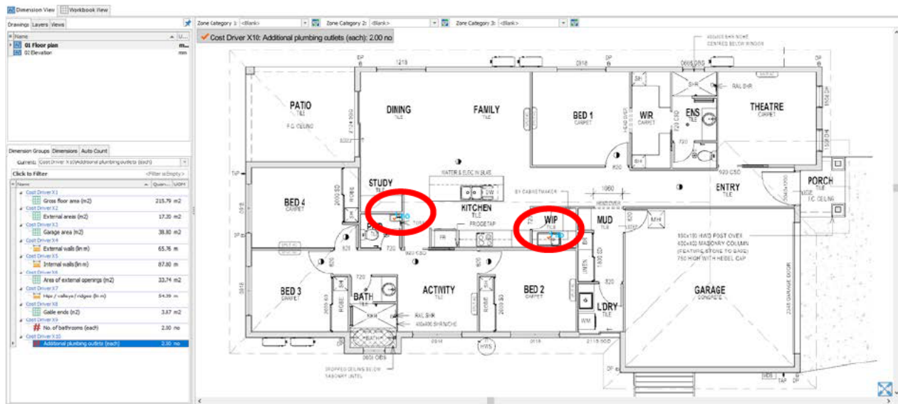
Figure 41 – Additional plumbing outlets measured example
