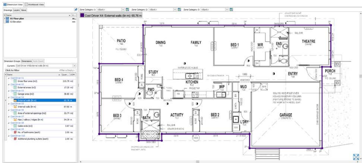
Figure 35 – External walls measured example
