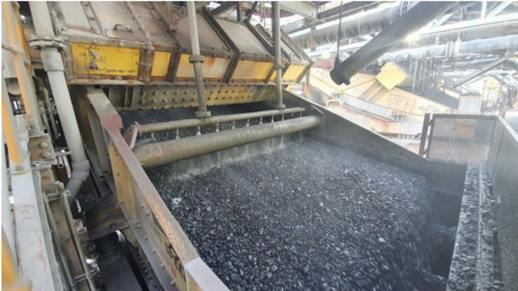
Figure 1.4: Top deck of banana screen.
