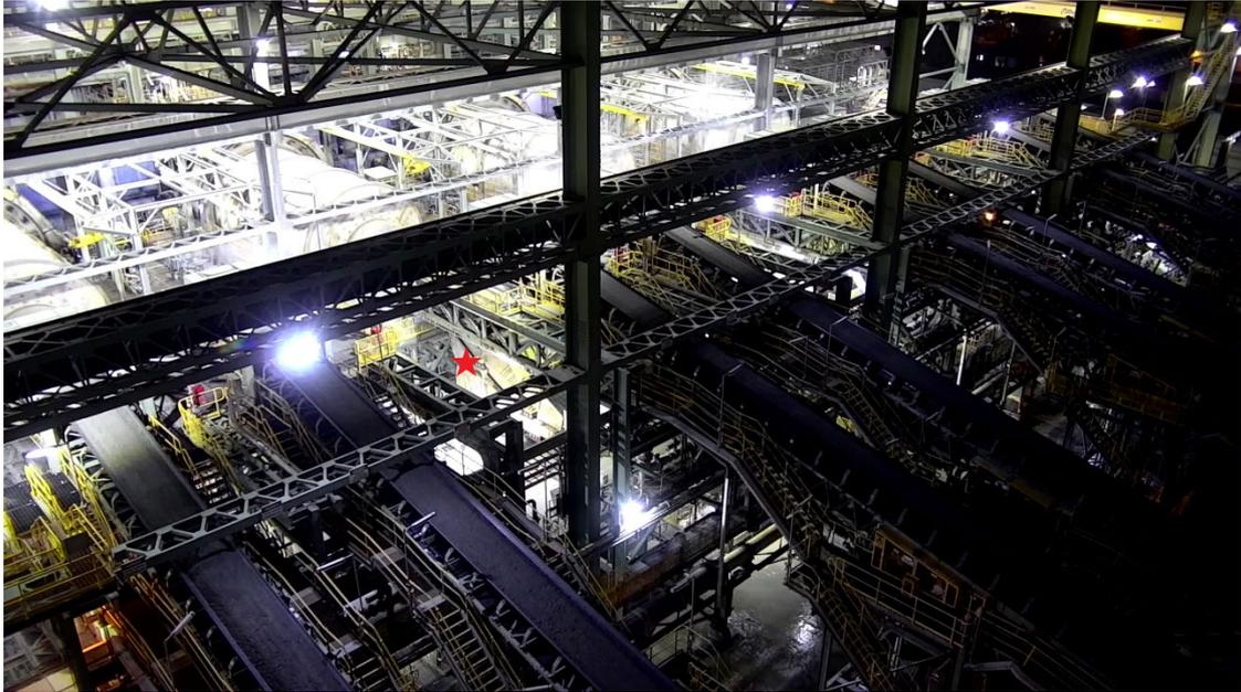
Figure 1.1: Top-down view of mill feeders (foreground) as they feed onto fine screens (red star) prior to feeding the ball mills (background).
