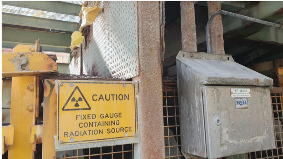
Figure 1.6: One of four nucleonic weightometers on the oversize return conveyor.
