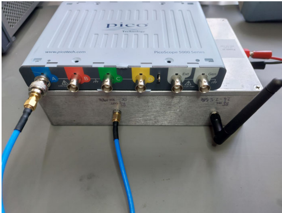
Figure 4.6: The acquisition system, showing RF downconverter connected to the PicoScope 5444B.
