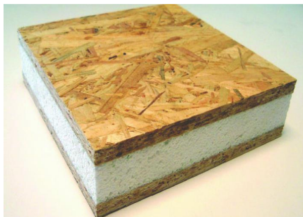
Figure 4 - Typical Structural Insulated Panel (SIPs) Formation
