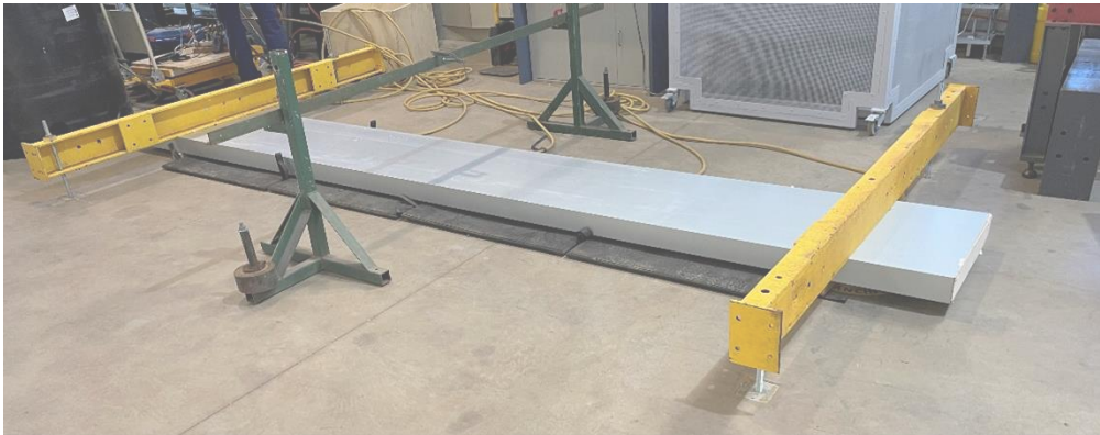
Figure 19 - Simply Supported Plank Setup with UDL
