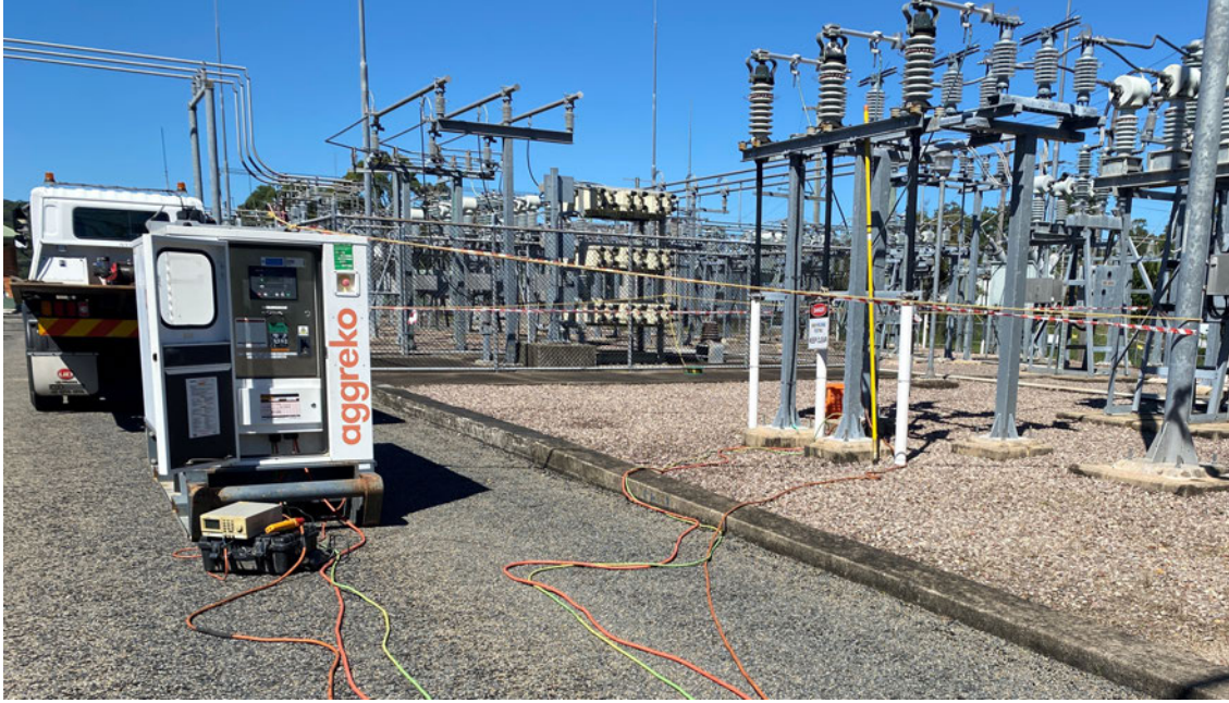
Figure 4.7: Generator connected to sealing end and set up for injection as part of remote earth testing.
