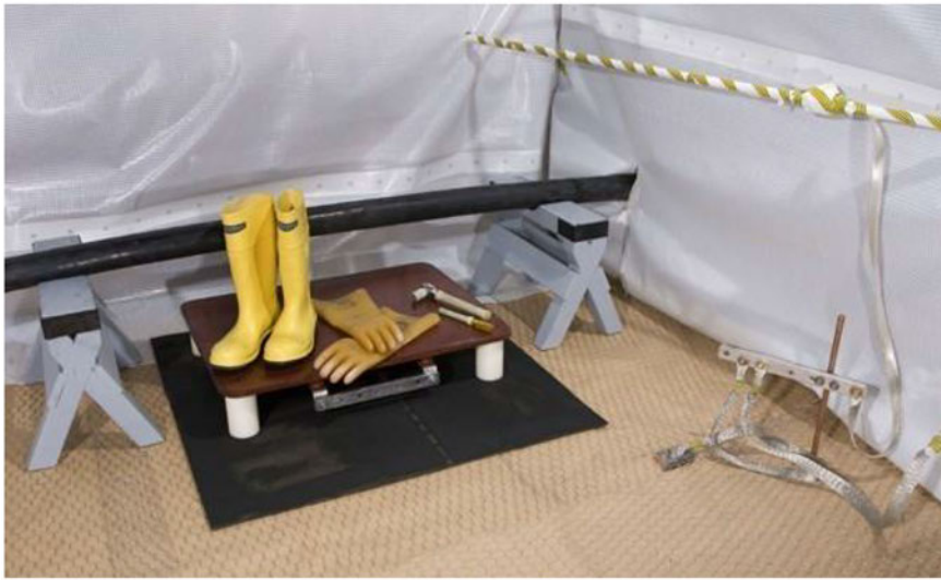
Figure 2.14: Examples of insulating working tools. (Cigré 2020a)
