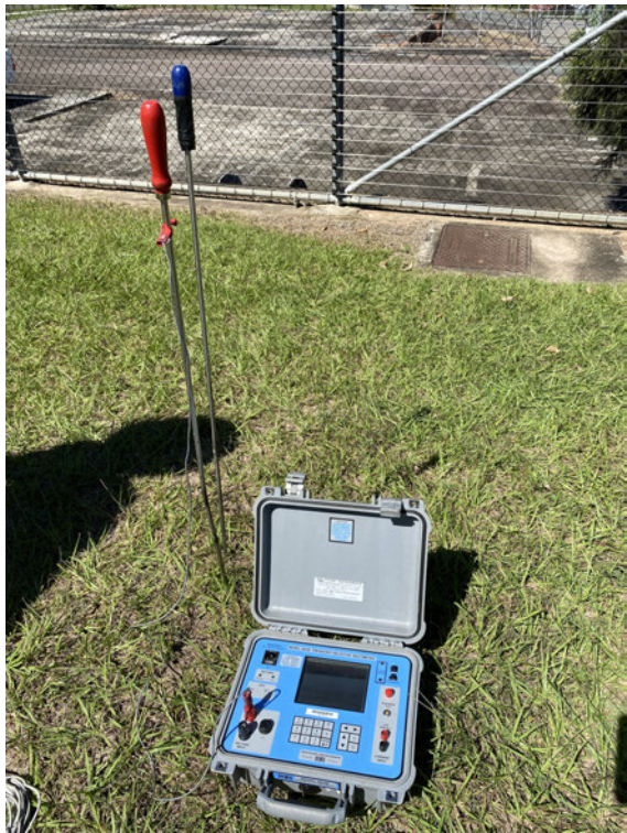
Figure 4.9: Probes and frequency selective multimeter which are used for remote earth injection testing.
