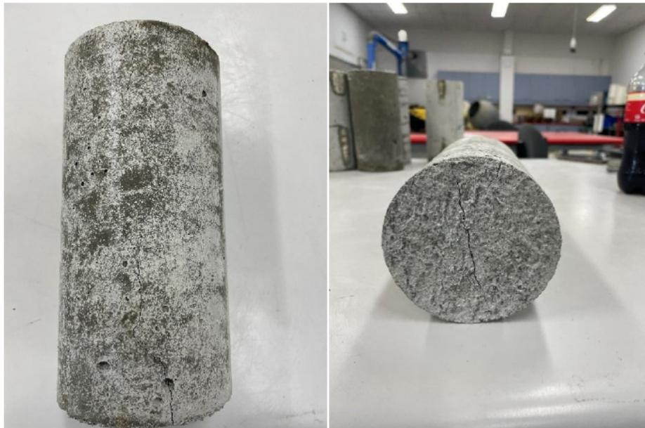
Fig. 5.14 – Sample from Batch – 1 after failure under tensile stress
