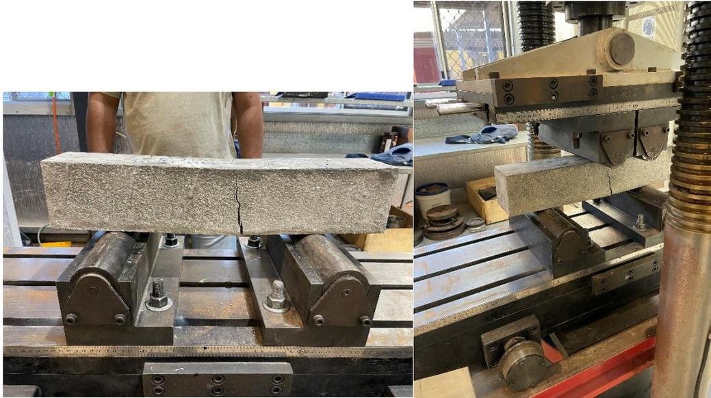
Fig 5.21 - Sample from Batch – 1 after failure under bending
