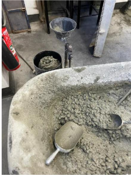
Fig. 5.2 – Vebe Test Z1 Civil Lab USQ
