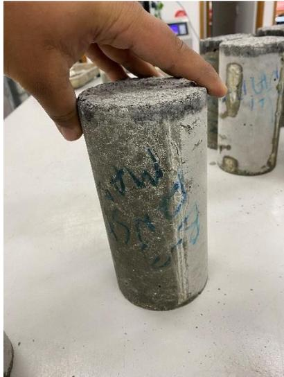
Fig. 5.10 – Sample from Batch – 3 after failure
