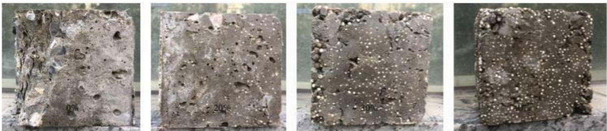
Fig. 2.5 – Failure mode of the EPS concrete with different EPS particles percentage (Rajah R.. 1999).
