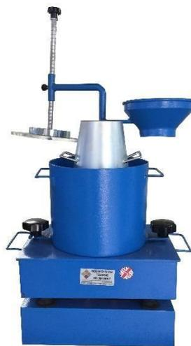
Fig. 3.4 – Consistometer at Toowoomba Campus. (USQ, Z1)
