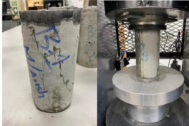
Fig. 5.8 – Sample from Batch – 1 after failure
