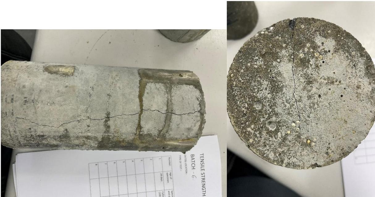
Fig. 5.17 – Sample from Batch – 7 after failure under tensile stress
