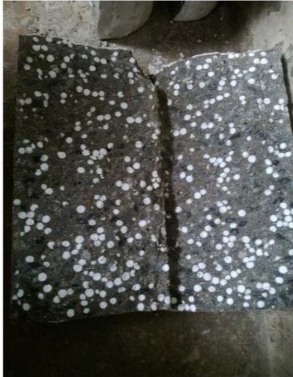
Fig. 2.10 – Broken surfaces of failed cylinders. (Thomas. T)
