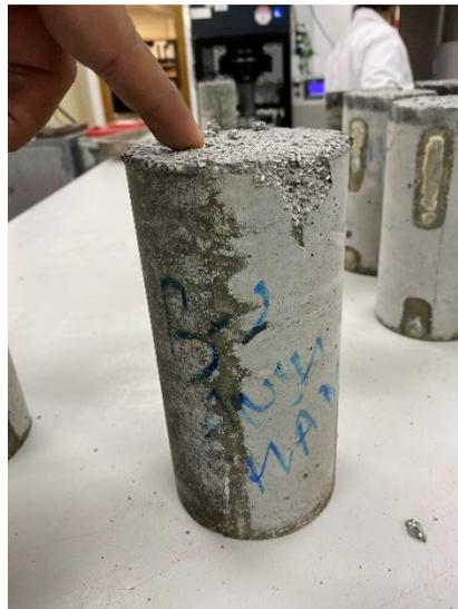
Fig. 5.9 – Sample from Batch – 2 after failure
