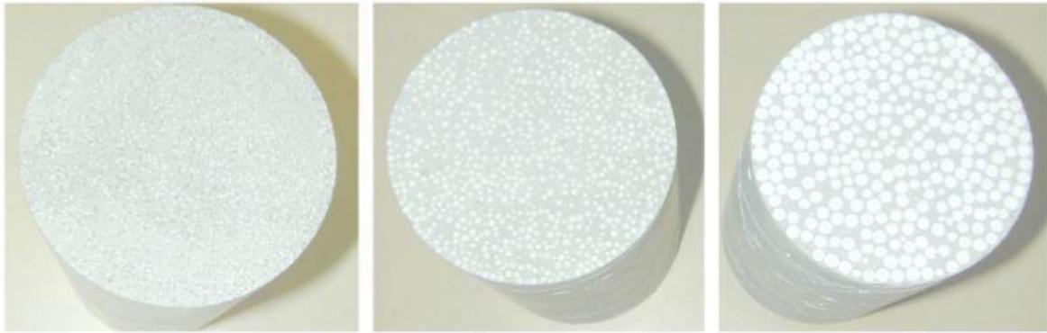
Fig. 2.1 – EPS concrete cylinders containing respectively 1 mm, 2.5 mm, and 6.3 mm EPS beads. (Shi, W., Miao, L. and Luo, J., 2016)
