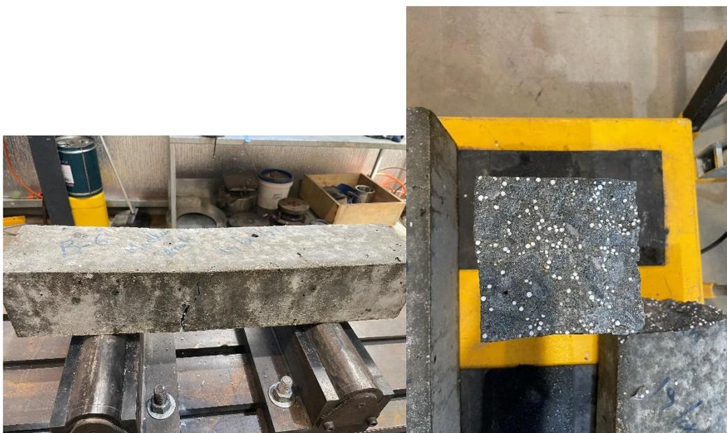
Fig 5.22 - Sample from Batch – 6 after failure under bending
