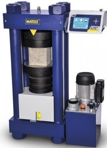
Fig. 3.2 – Compression Machine at Toowoomba Campus. (USQ, Z1)
