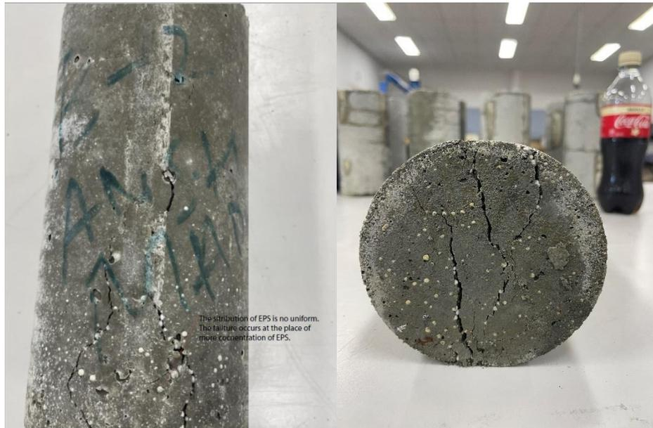
Fig. 5.15 – Sample from Batch – 2 after failure under tensile stress
