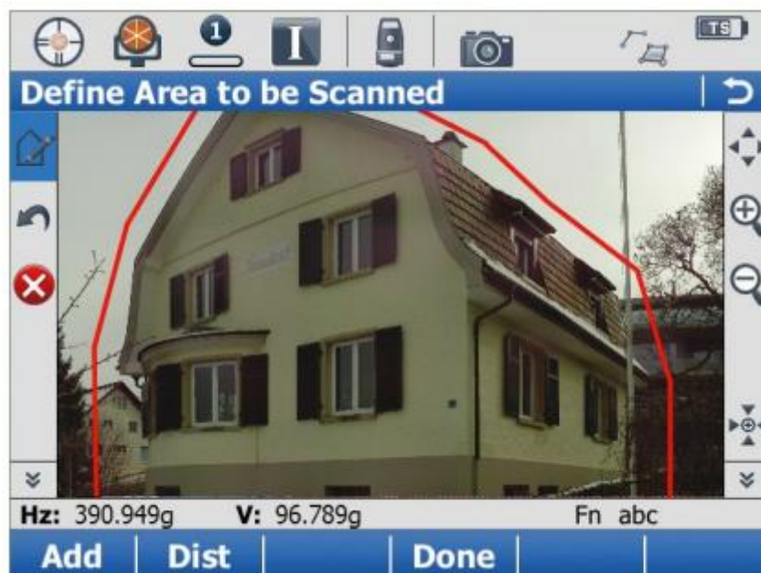
Figure 5. Leica Nova MS50 Scanning selection screen with polygon (Leica, 2013)
