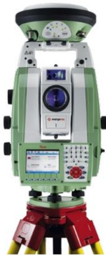
Figure 4. Leica Nova MS50 with SmartStation setup with GNSS receiver on top (Leica, 2013)
