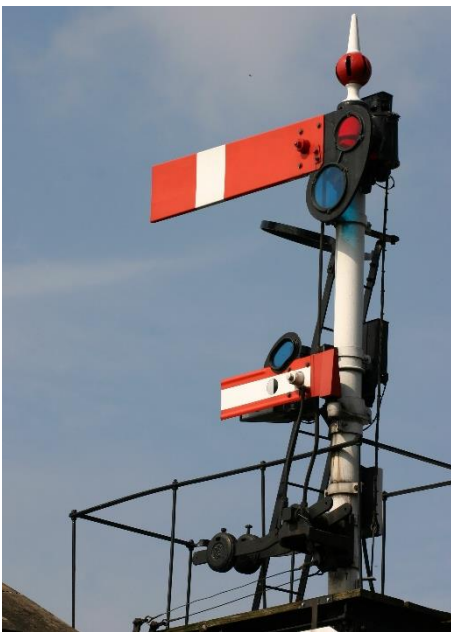
Figure 3: British lower-quadrant semaphore stop signal (absolute) with subsidiary arm (permissive) below (David Friel, 2005)
