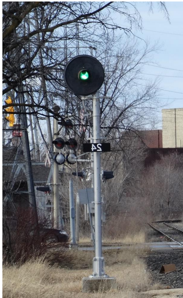
Figure 11: Searchlight signal showing an 'all clear' signal ()
