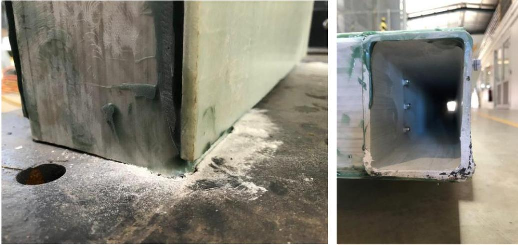
**Figure 4-10: Minor crushing of right-hand vertical stud, for panel FSE**
