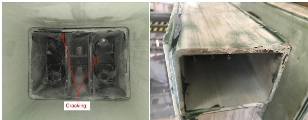
(a) Slight cracking of right-hand insert (b) Minor crushing of right-hand vertical stud
