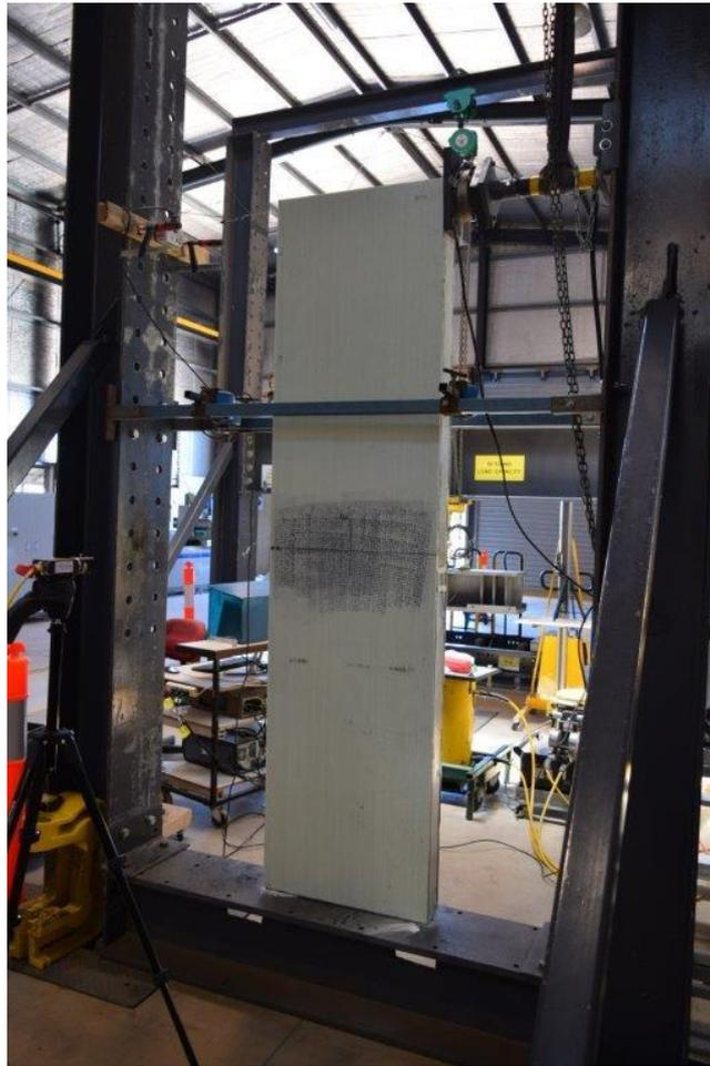
**Figure 4-5: Panel FSE installed in testing frame**
