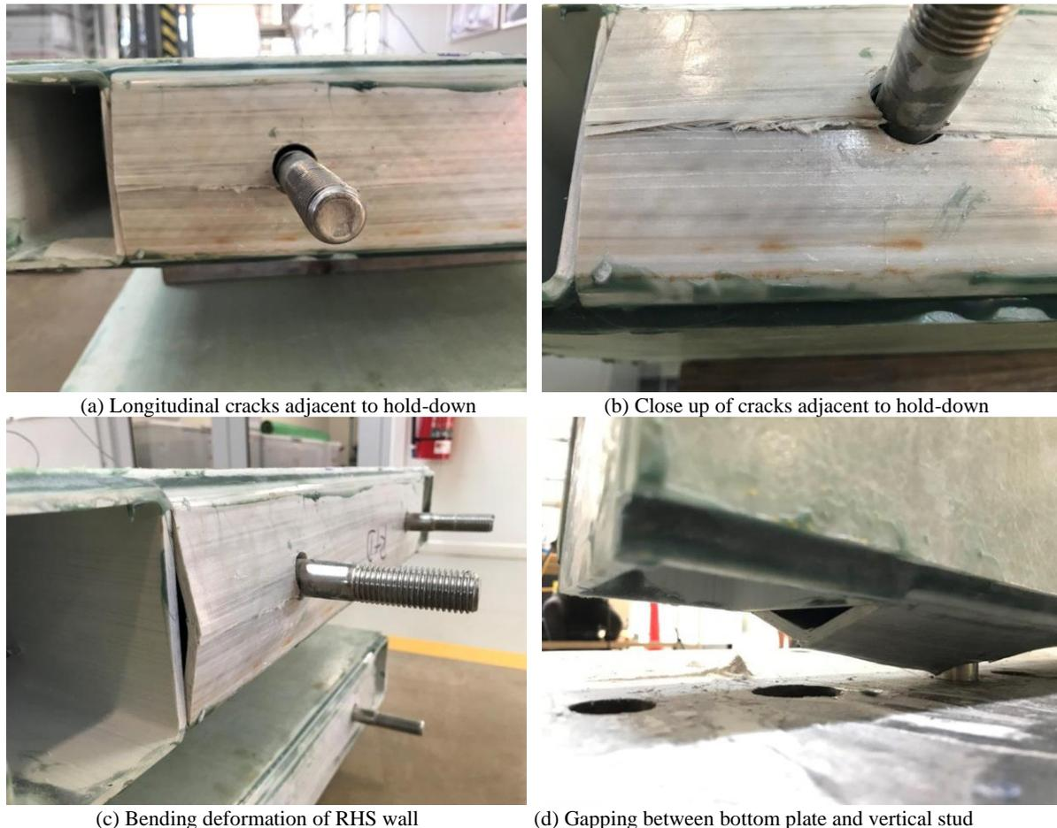
**Figure 4-17: Failure of the RHS bottom plate at left-hand hold down, with (a)-(b) longitudinal splitting, (c) bending deformation, and (d) gapping between bottom plate and vertical stud, for panel FSO37.5E**
