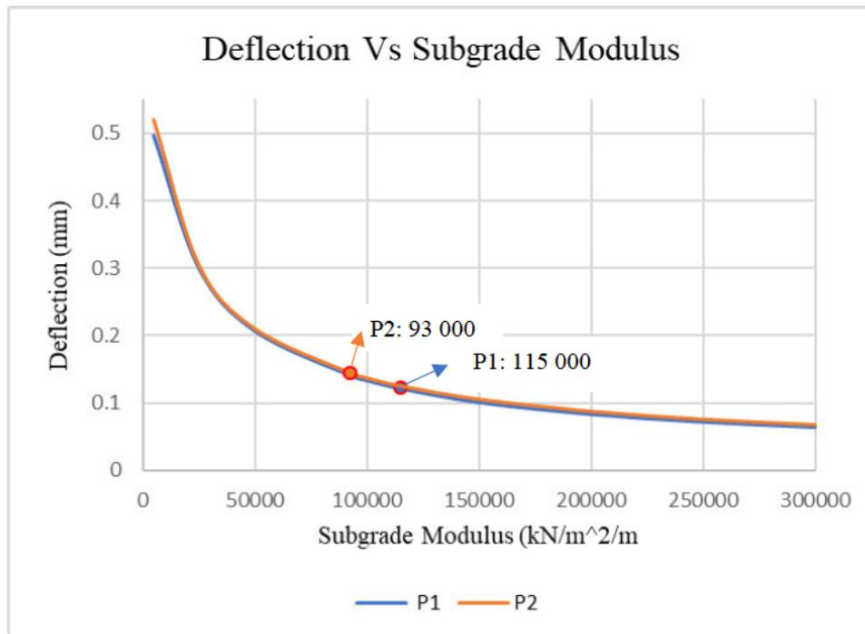
Figure 4.27: Deflection verse subgrade modulus
