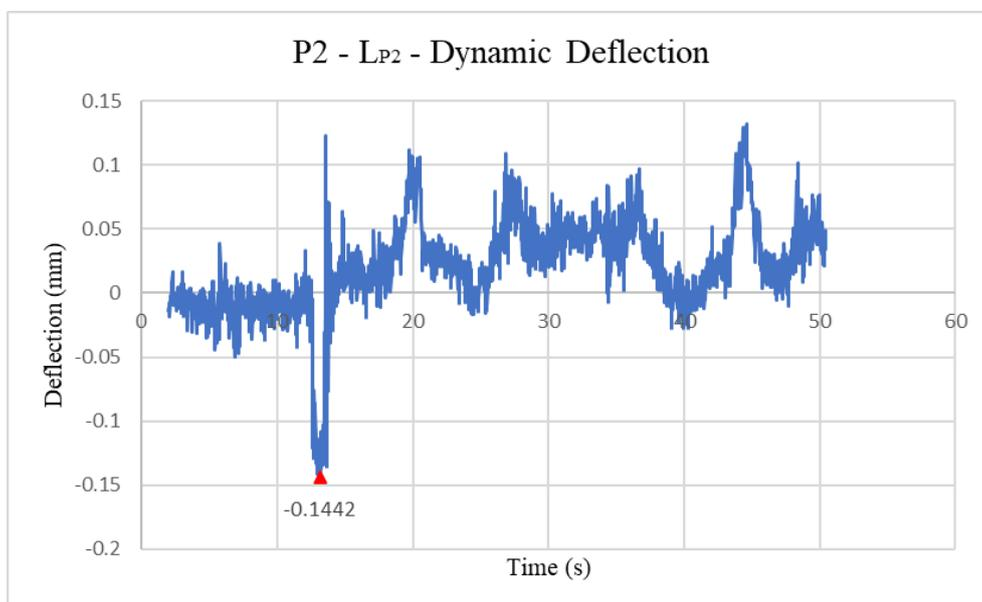
Figure 4.17: P2 – LP<sub>2</sub> – Dynamic Deflection at position 1
