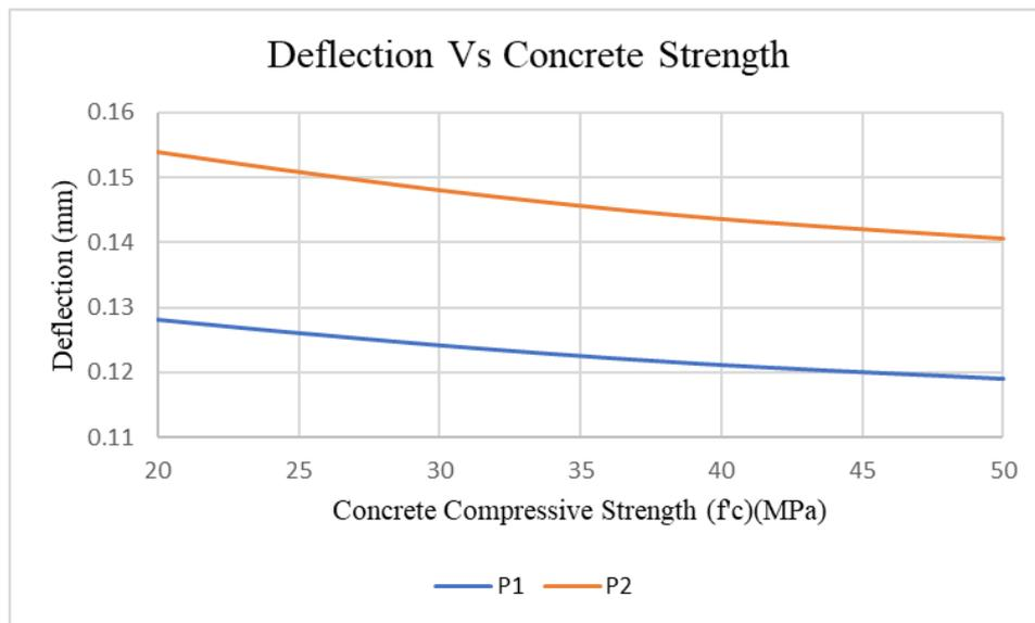
Figure 4.30: Deflection verse concrete compressive strength.
