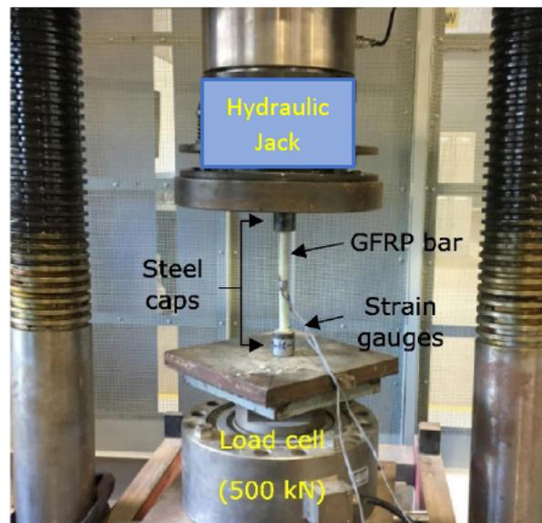
Figure 2.5: Compression testing (AlAjarmeh et al. 2019)
