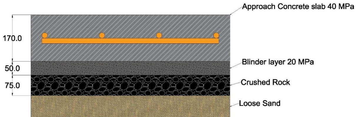
Figure 3.1: Cross section of subgrade preparation.
