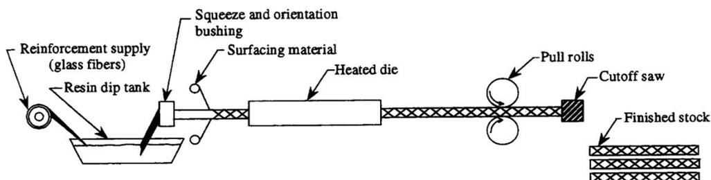
Figure 2.3: Fabrication process of GFRP (Benmokrane et al. 1995).
