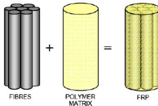
Figure 2.2: Basic material composition of FRP products (Abedini et al. 2017)
