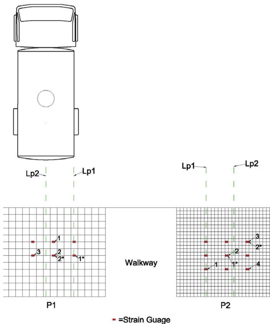
Figure 4.1: Strain gauge and load path locations.
