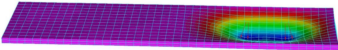
Figure 4.21: Model of slab P1 with loading applied demonstrating deflection.
