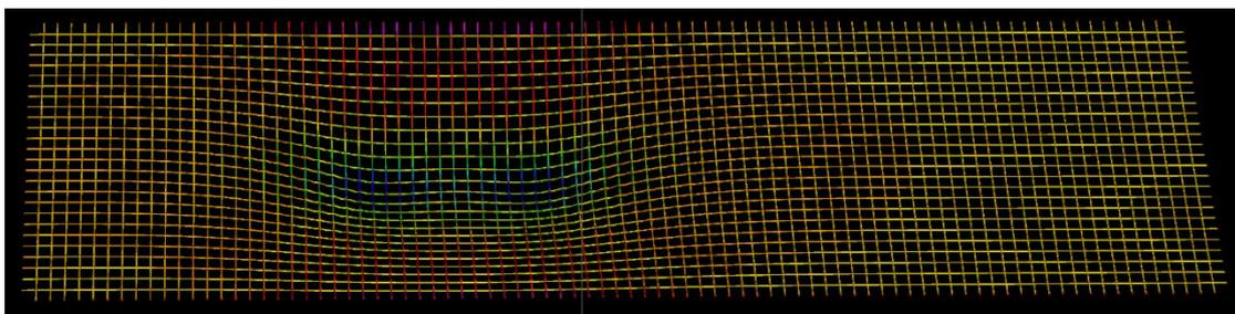
Figure 4.25: Stress concentrations in reinforcing mesh for slab P2
