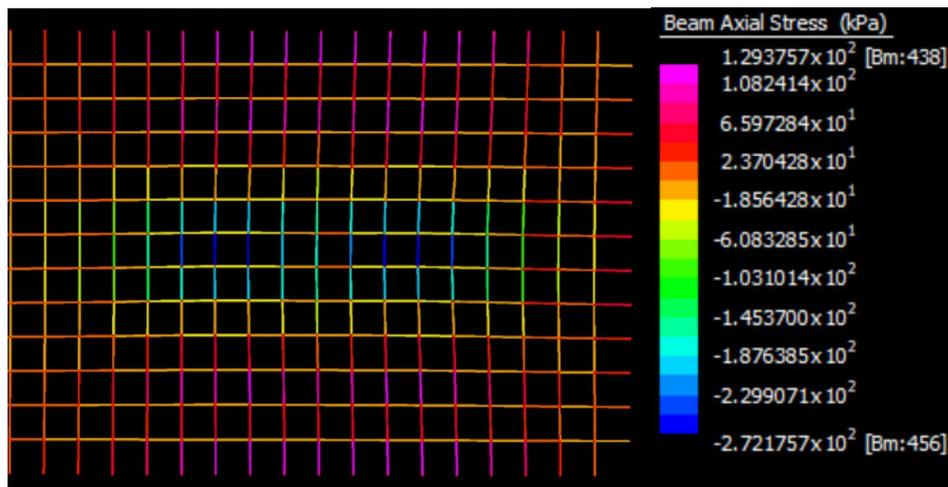
Figure 4.22: Stress in reinforcing mesh slab P1.
