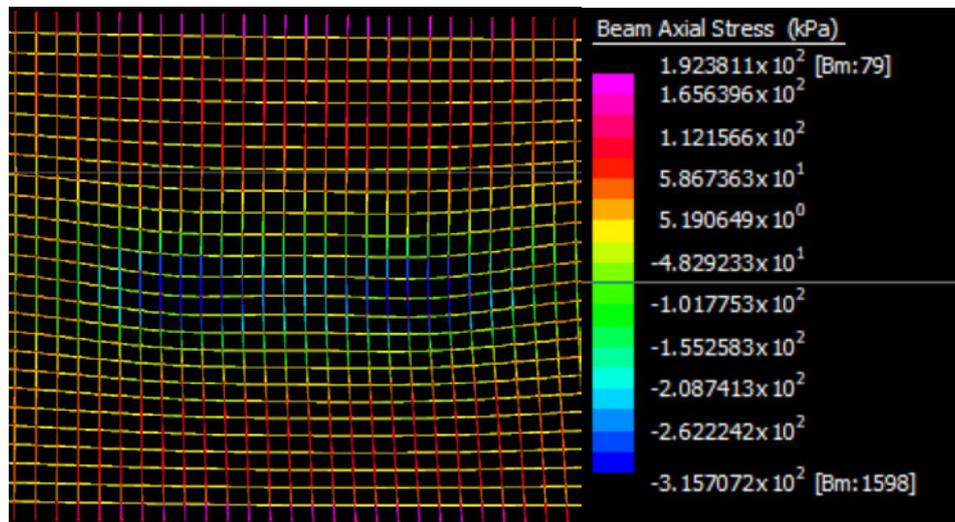
Figure 4.26: Stress distribution in slab P2
