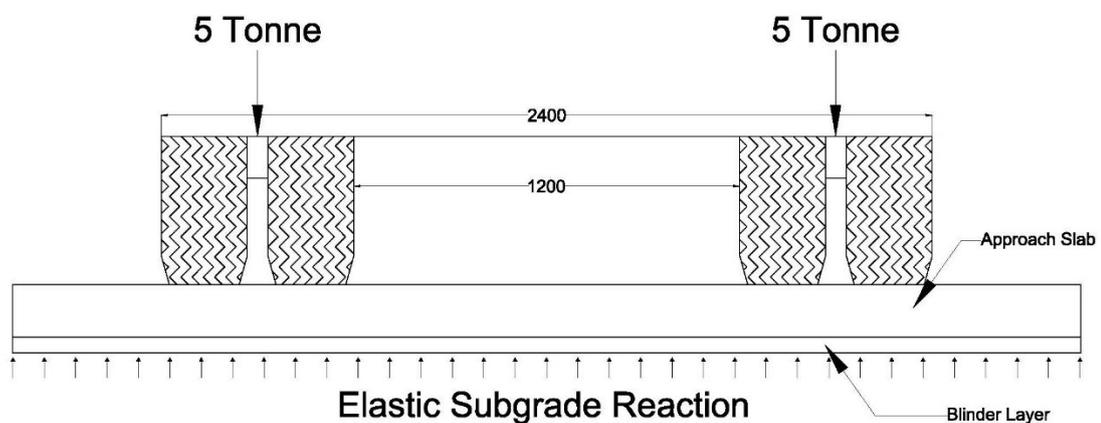
Figure 4.18: Loading Configuration.
