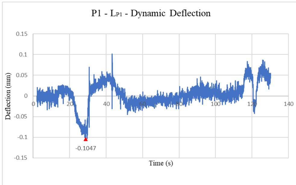
Figure 4.7: P1 – LP<sub>1</sub> – Dynamic Deflection at position 1\*
