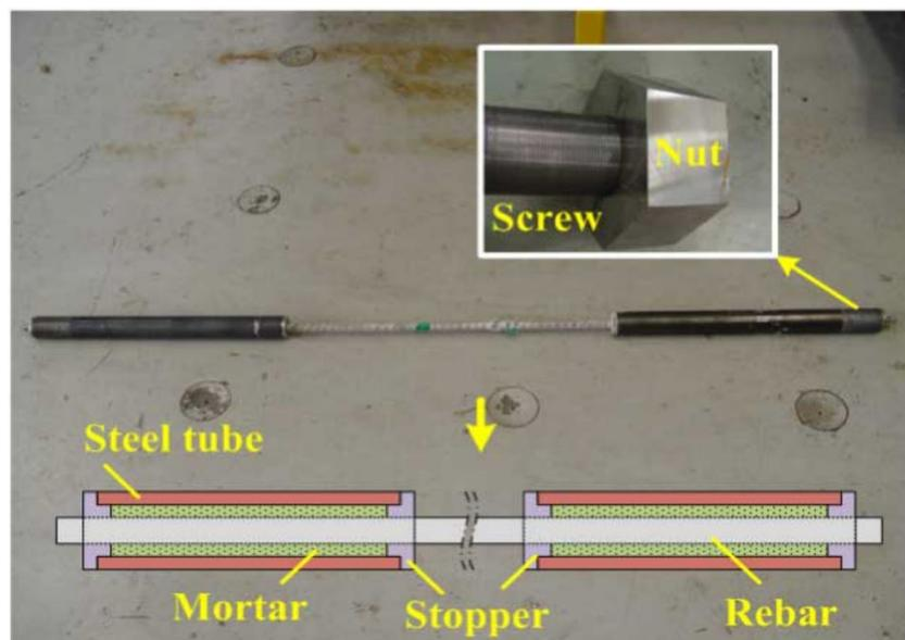
Figure 2.4: GFRP bar ready for tensile testing (You et al. 2015).
