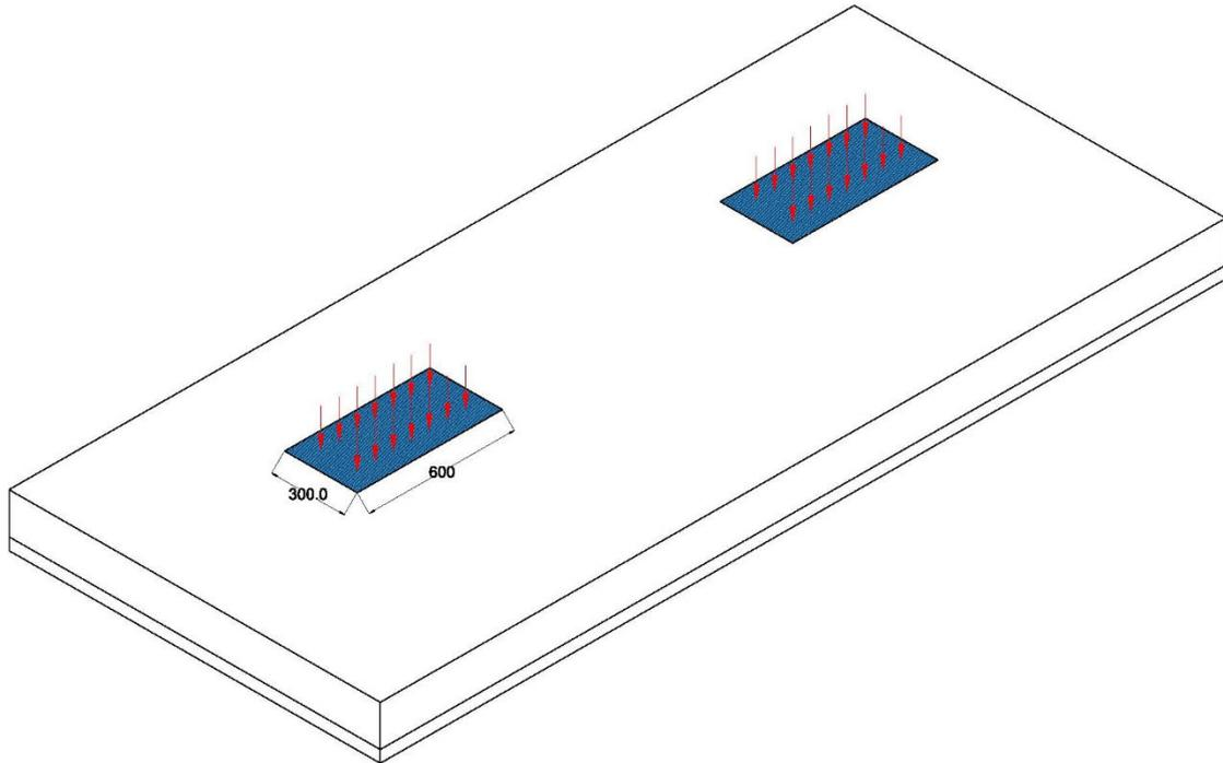
Figure 4.19: Truck tyre contact footprint.
