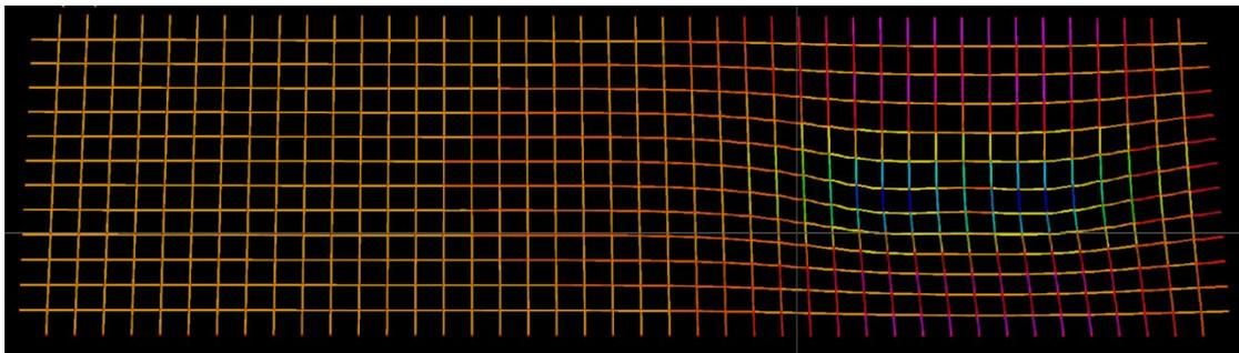
Figure 4.22: Stress concentrations in reinforcing mesh for slab P1
