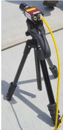
Figure 4.2: High-performance DIC camera
