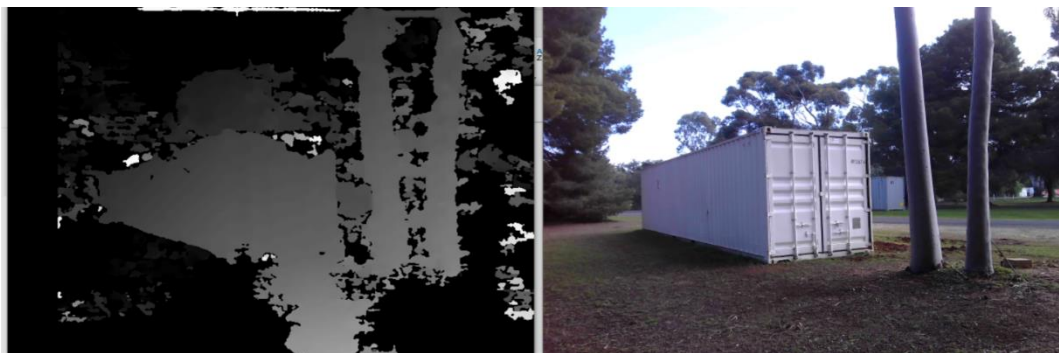
Figure 10 - Outdoor stereoSGBM Algorithm Results 640 x 480 Resolution 0.26m Baseline
