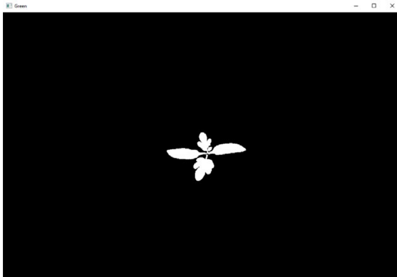
Figure 9: Binary black and white Image used for contour creation and area calculation
