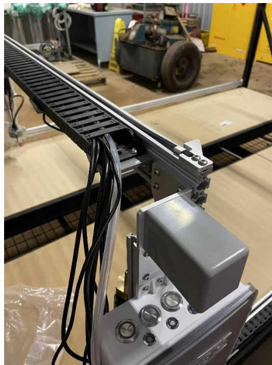
Figure 5: Completed installation of the Y axis cable carrier and cables.
