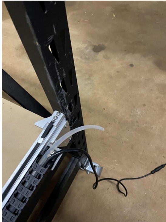
Figure 6: The completed installation of the X axis cable carrier and cables.
