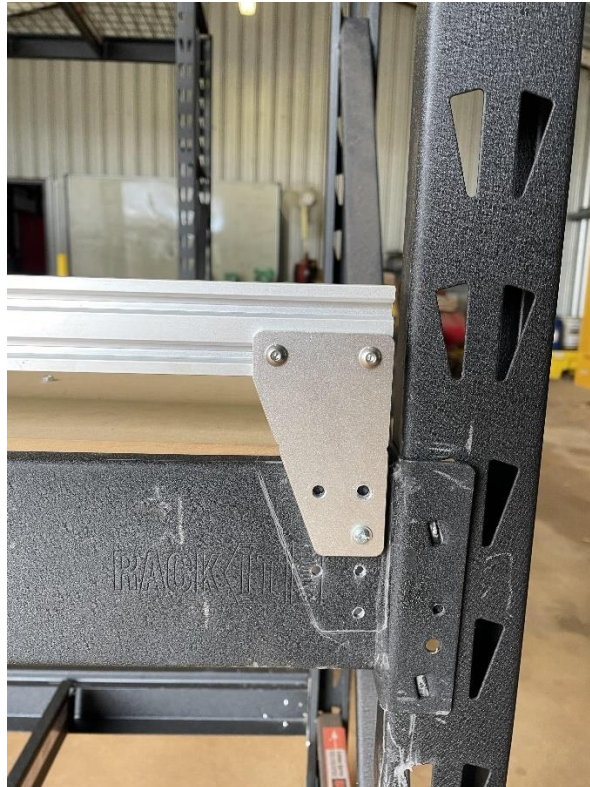
Figure 3: Incremental raising of the gantry tracks.
