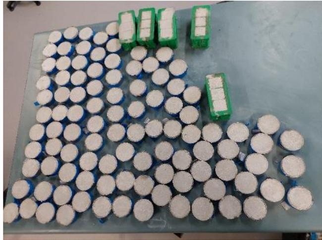
*Figure 27: Set Artificial Rock Joints*
