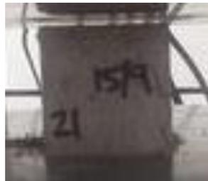
Figure 126: 21 Day Compression Testing Sample 4 (After Testing)
