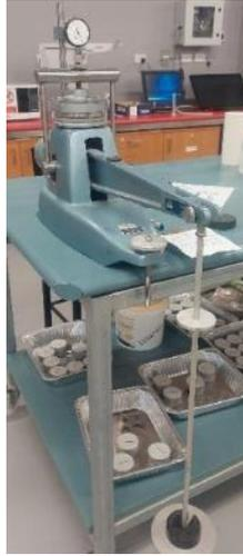
*Figure 47: First load applied to sample*
