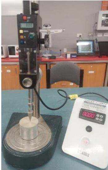
*Figure 39: Cone Penetrometer ready for release*
