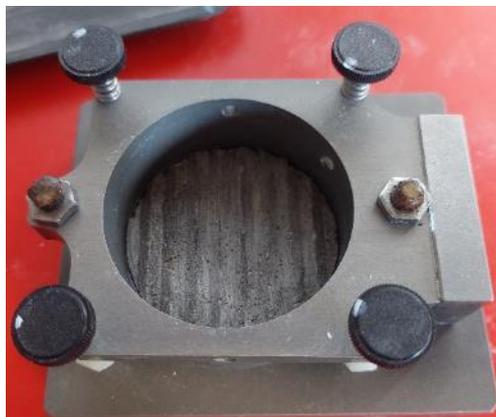
*Figure 64: Alignment of bottom joint in shear box*
