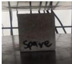
Figure 142: 28 Day Compression Testing Sample 5 (Before Testing)
