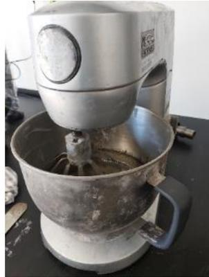
*Figure 25: Cement Grout Mixing*
