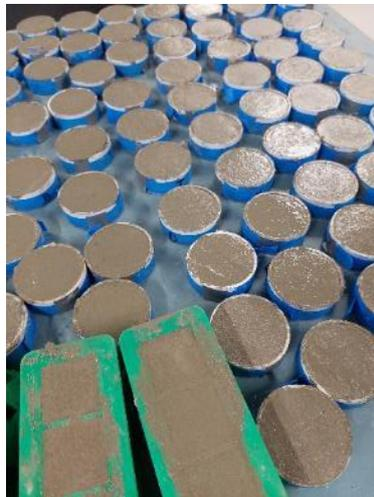
*Figure 26: Freshly Poured Moulds*
