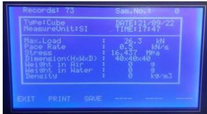
Figure 141: 28 Day Compression Testing Sample 4 (Results)
