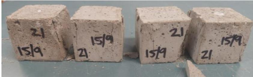
*Figure 128: 21 Day Compression Testing Samples (After Testing)*
