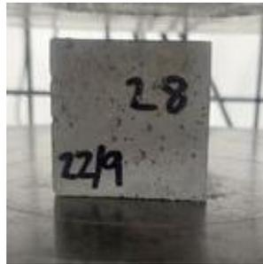
Figure 133: 28 Day Compression Testing Sample 2 (Before Testing)
