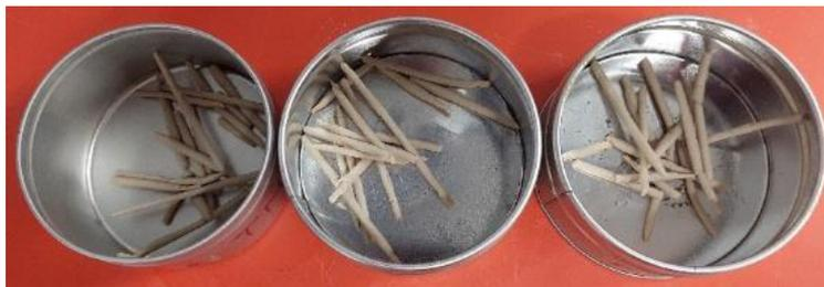
*Figure 42: Plastic Limit samples before oven drying to find moisture content*
