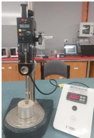
*Figure 40: Cone Penetrometer after release with penetration reading*
