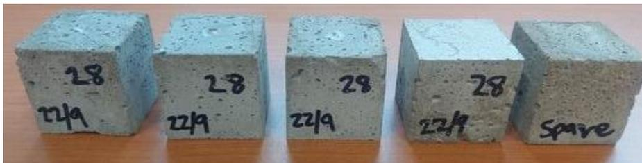
*Figure 129: 28 Day Compression Testing Samples (Before Testing)*
