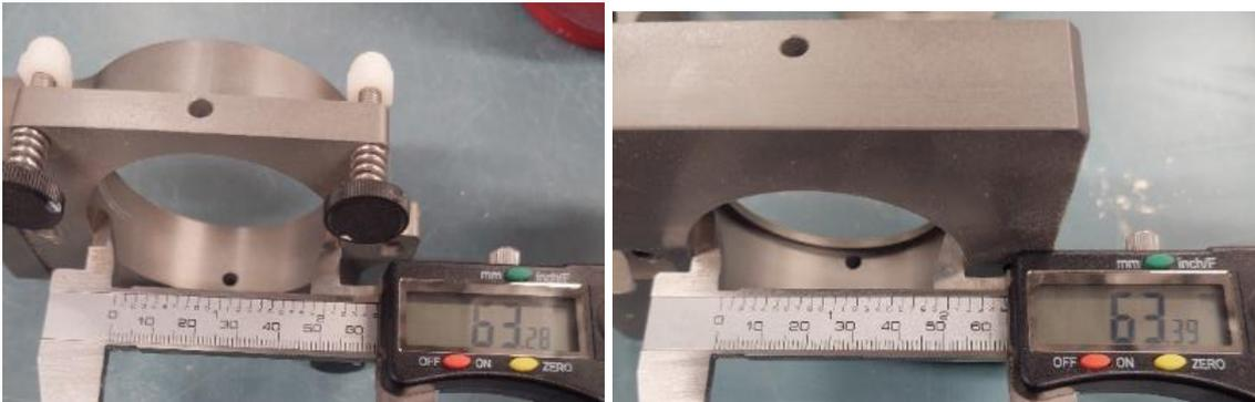
*Figure 53: Internal diameter of split box top (left) and bottom (right)*
