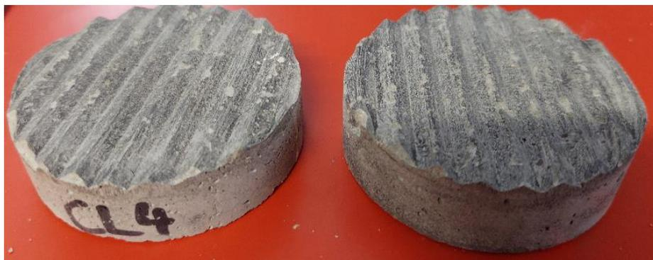
Figure 88: Joint CL4 (after testing)
