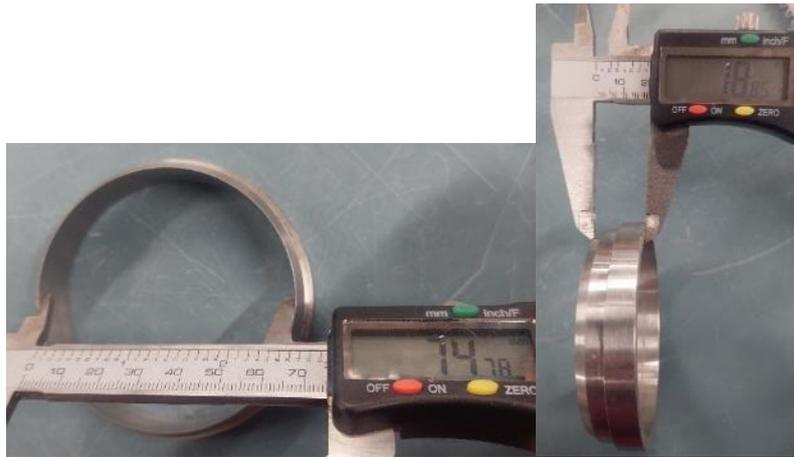
*Figure 45: Consolidation ring measurements diameter (left) and height (right)*
