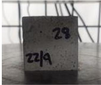
Figure 136: 28 Day Compression Testing Sample 3 (Before Testing)
