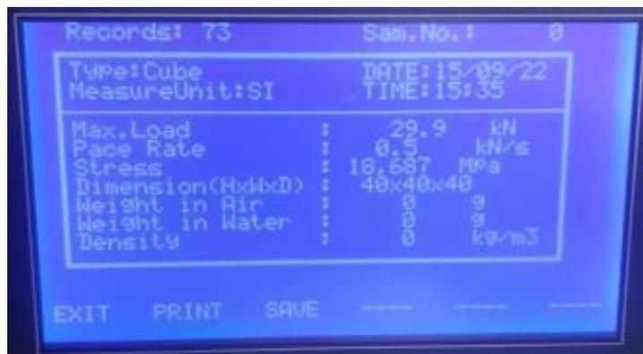
Figure 127: 21 Day Compression Testing Sample 4 (Results)
