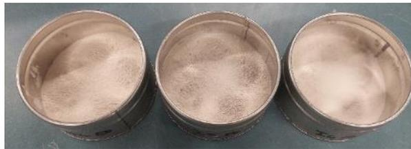
*Figure 36: Soil samples (natural state) ready for oven drying*
