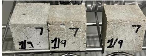
*Figure 93: 7 Day Compression Testing Samples (Before Testing)*
