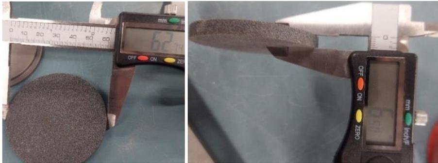
*Figure 55: Diameter (left) and thickness (right) of porous plate*
