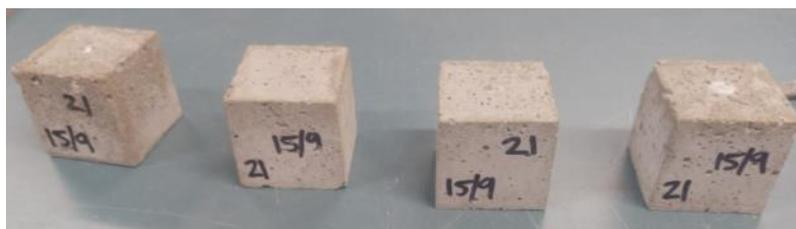
Figure 115: 21 Day Compression Testing Samples (Before Testing)
