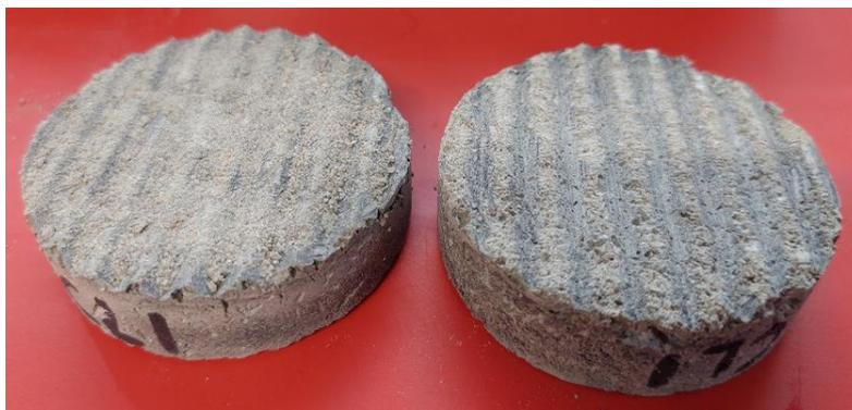
Figure 85: Joint Failure on Sample CL1
