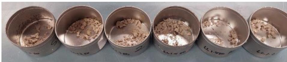
*Figure 41: Liquid Limit samples after oven drying to find moisture content*
