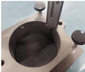
Figure 58: Total height of split box with base plate and one (1) porous stone installed
