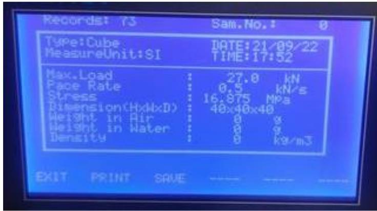
Figure 144: 28 Day Compression Testing Sample 5 (Results)
