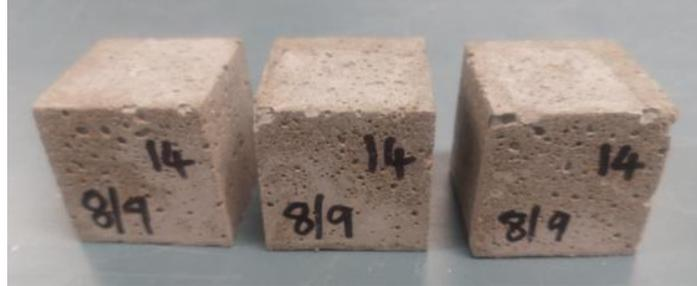
*Figure 104: 14 Day Compression Testing Samples (Before Testing)*
