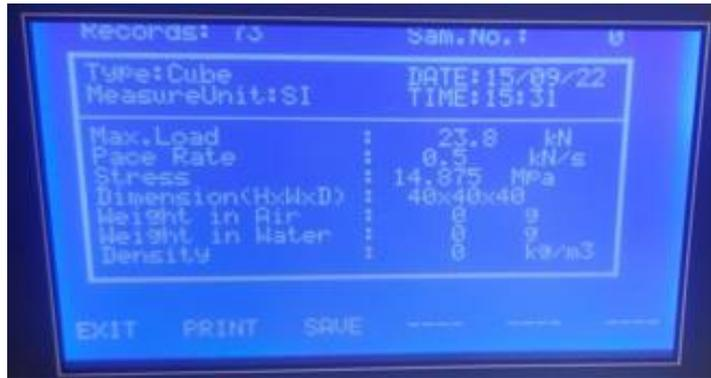
Figure 124: 21 Day Compression Testing Sample 3 (Results)
