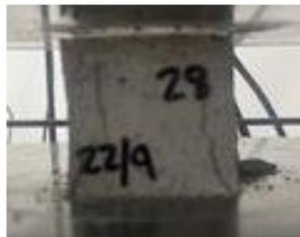
Figure 137: 28 Day Compression Testing Sample 3 (After Testing)
