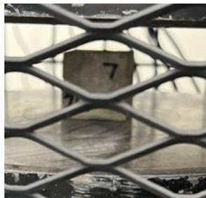
Figure 97: 7 Day Compression Testing Sample 2 (Before Testing)
