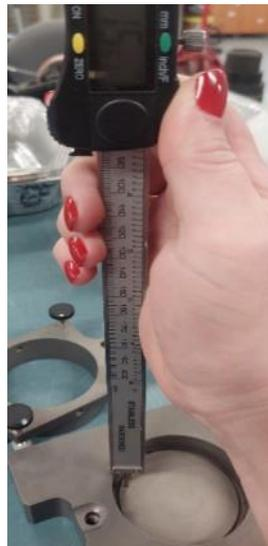
*Figure 56: height of bottom split box with base plate installed*
