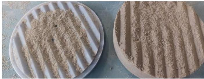
Figure 24: Demoulding of Initial Cement Grout Mix
