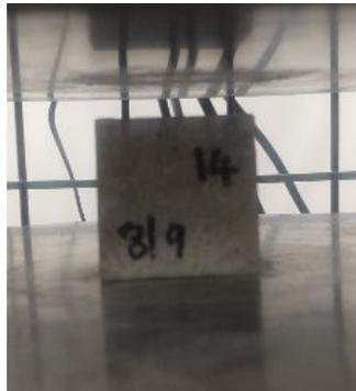
Figure 111: 14 Day Compression Testing Sample 3 (Before Testing)
