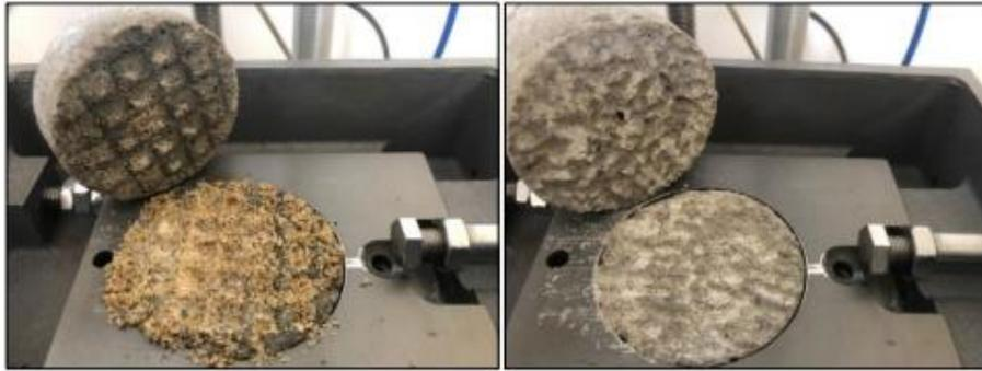
Figure 7: Sawtooth and Sinusoidal Joint Profiles (Zohaib, Mirzagherbanali, Helwig, Azzia, Gregor, Rastegarmanesh & McDougall 2020)
