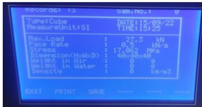
*Figure 118: 21 Day Compression Testing Sample 1 (Results)*
