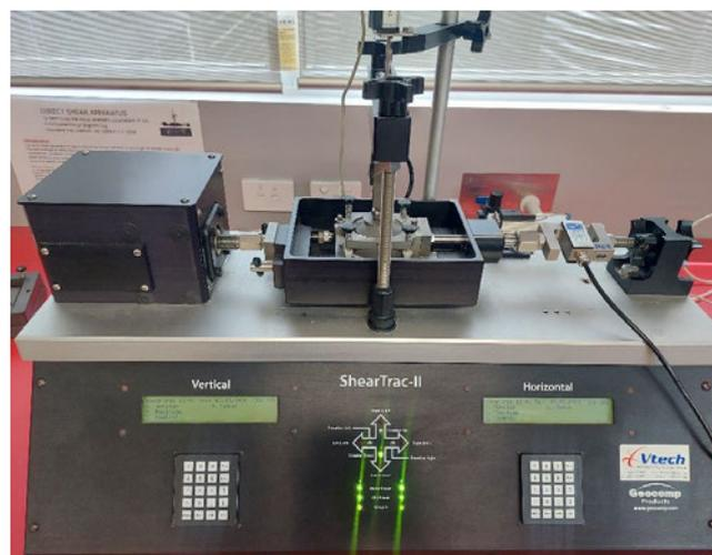
*Figure 13: ShearTrac2 Shear Apparatus*
