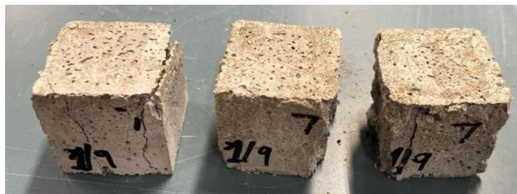
Figure 103: 7 Day Compression Testing Samples (After Testing)
