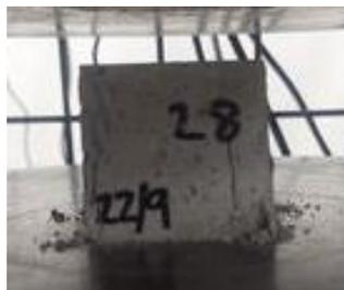
Figure 134: 28 Day Compression Testing Sample 2 (After Testing)
