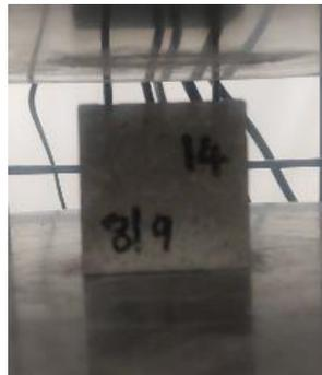
Figure 108: 14 Day Compression Testing Sample 2 (Before Testing)
