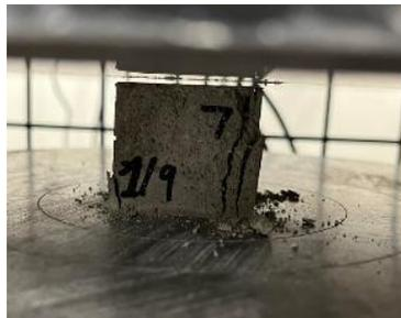
Figure 98: 7 Day Compression Testing Sample 2 (After Testing)
