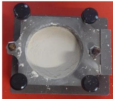
*Figure 61: Soil material in shear box*
