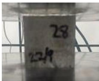
Figure 139: 28 Day Compression Testing Sample 4 (Before Testing)
