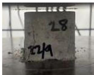
*Figure 131: 28 Day Compression Testing Sample 1 (After Testing)*
