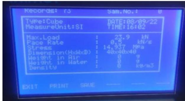
Figure 113: 14 Day Compression Testing Sample 3 (Results)
