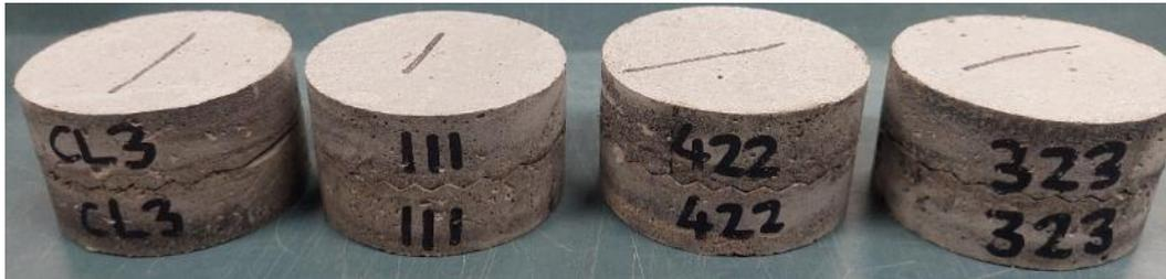
Figure 62: Artificial rock joints with test codes
