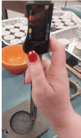
Figure 57: height of bottom split box with base plate and one (1) porous plate installed
