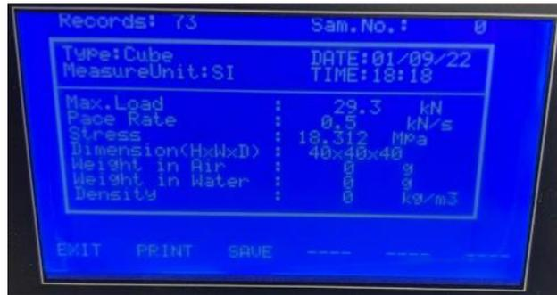
Figure 96: 7 Day Compression Testing Sample 1 (Results)
