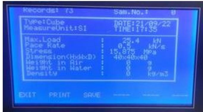
Figure 132: 28 Day Compression Testing Sample 1 (Results)
