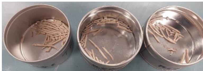
*Figure 43: Plastic Limit samples after oven drying to find moisture content*
