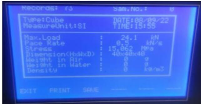
Figure 107: 14 Day Compression Testing Sample 1 (Results)
