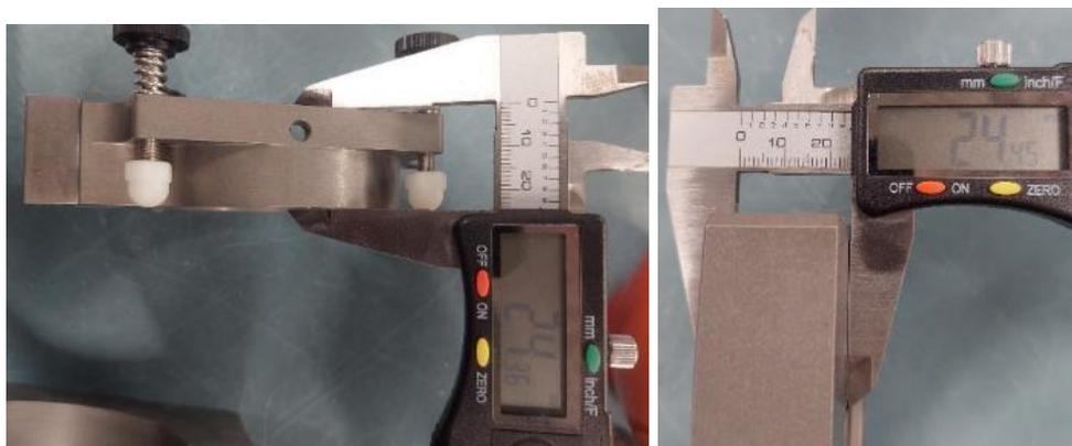
*Figure 54: Height of split box top (left) and bottom (right)*
