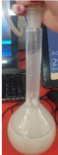
Figure 35: Applying partial vacuum to remove entrapped air
