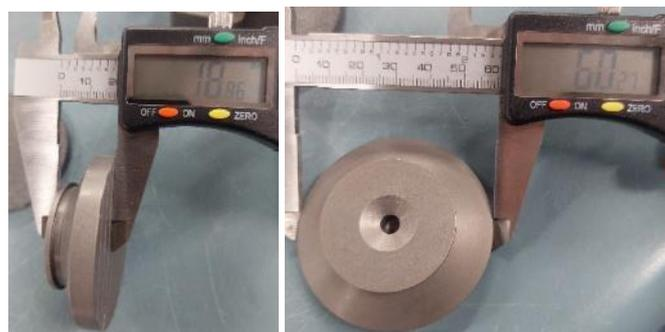
Figure 59: Dimensions of load pad height (left) and diameter (right)
