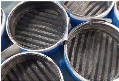
*Figure 22: Greased Moulds*
