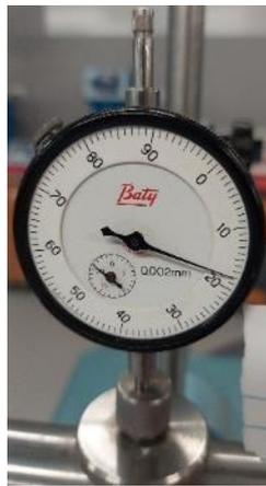
*Figure 48: Dial gauge reading at 24 hours for 1 kg weight*
