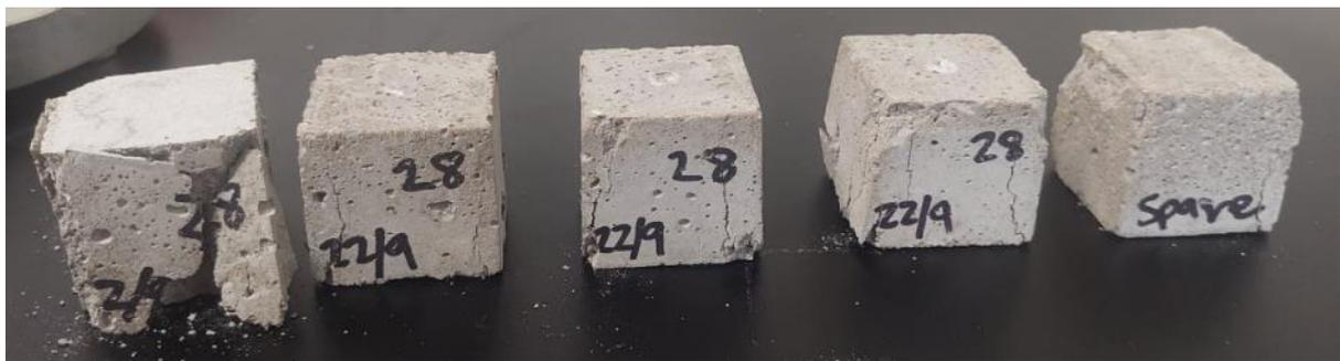
Figure 145: 28 Day Compression Testing Samples (After Testing)
