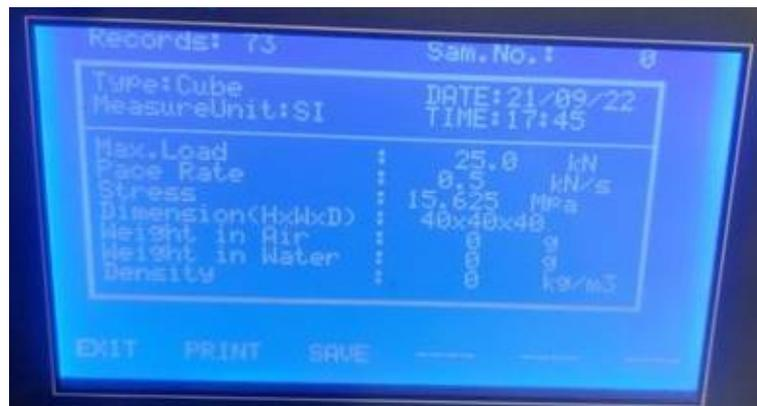
Figure 138: 28 Day Compression Testing Sample 3 (Results)
