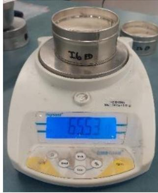
Figure 37: Weighing of dried soil sample
