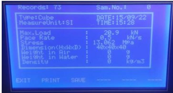
Figure 121: 21 Day Compression Testing Sample 2 (Results)
