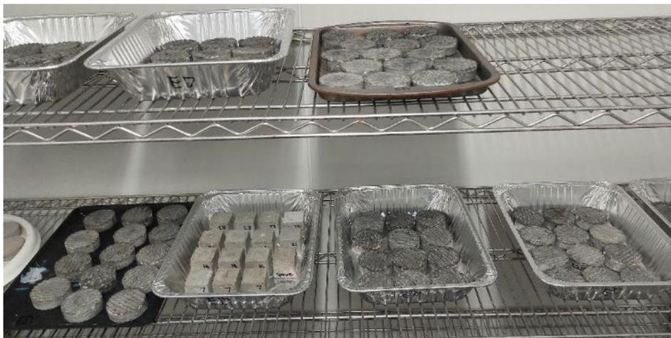
*Figure 29: Demoulded Samples in curing room*
