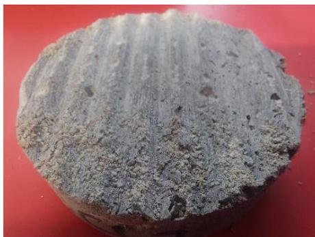
Figure 86: Joint Failure of Sample CL2
