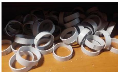
*Figure 20: 19mm DN65 DWV PVC pipe lengths*
