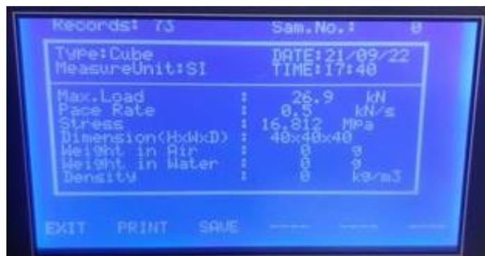
Figure 135: 28 Day Compression Testing Sample 2 (Results)
