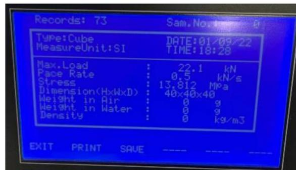
Figure 102: 7 Day Compression Testing Sample 3 (Results)
