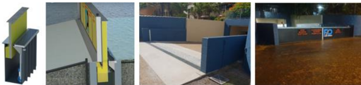
Figure 3.26: Flow Defence comes as a self-contained unit that is automatically raised by floodwaters entering the systems water storage tank (Flow Defence 2022).
