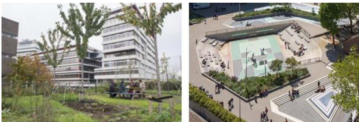
Figure 3.6(a) and 3.6(b): Rotterdam reduces stress on drainage systems by storing excess storm water in rooftop green spaces and a sunken basketball court (Baurick, Wendland, Granger 2020 and Van Duivenbode 2022)
