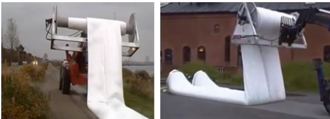
Figure 3.29: The barrier can be quickly deployed by a small truck or fork lift (Bluemont 2022).
