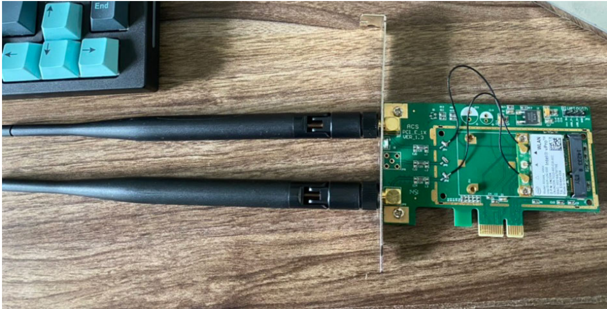
Figure 4.1: Intel 5300 802.11n NIC installed into PCI-E x16 NIC Adapter
