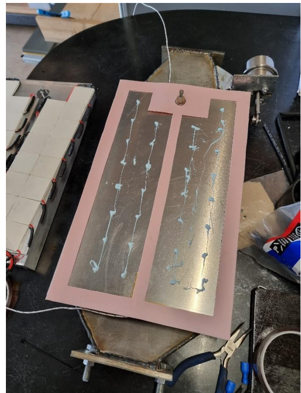
Figure 34 - Hotplate with thermal paste and silicone mat
