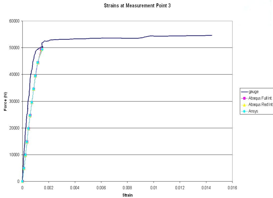
Figure 5.8: Results of FEA by ANSYS and ABAQUS for horizontally oriented hole compared to experimental measurements at position 3.
