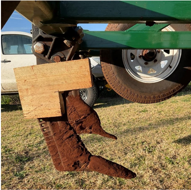
Figure 8 - Boards attached to the ripper shank to catch the large piece laying on the ground
