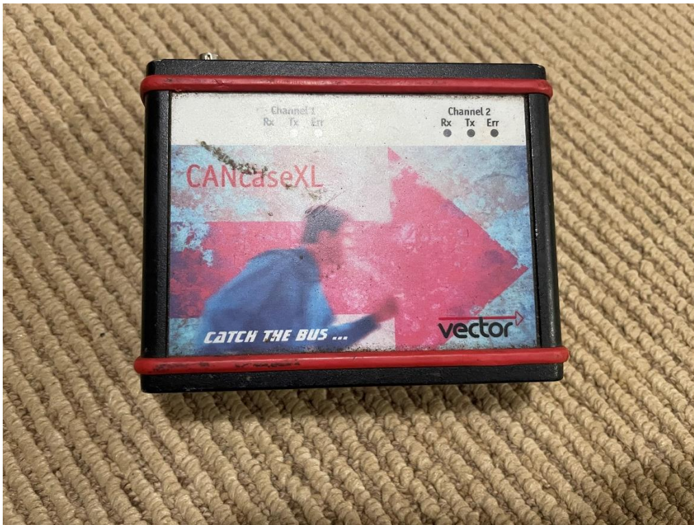
Figure 15 - Vector CANcaseXL that was used to communicate with the CAN Bus on the Joh Deere 6120R
