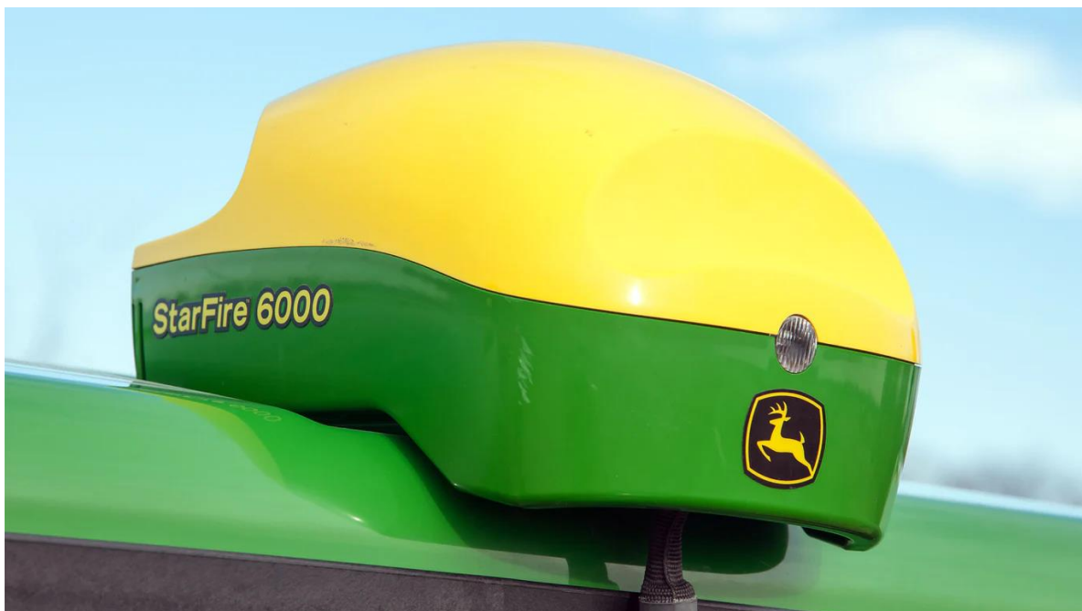
Figure 11 - John Deere Starfire 6000 GPS receiver that is fitted to the 6120R
