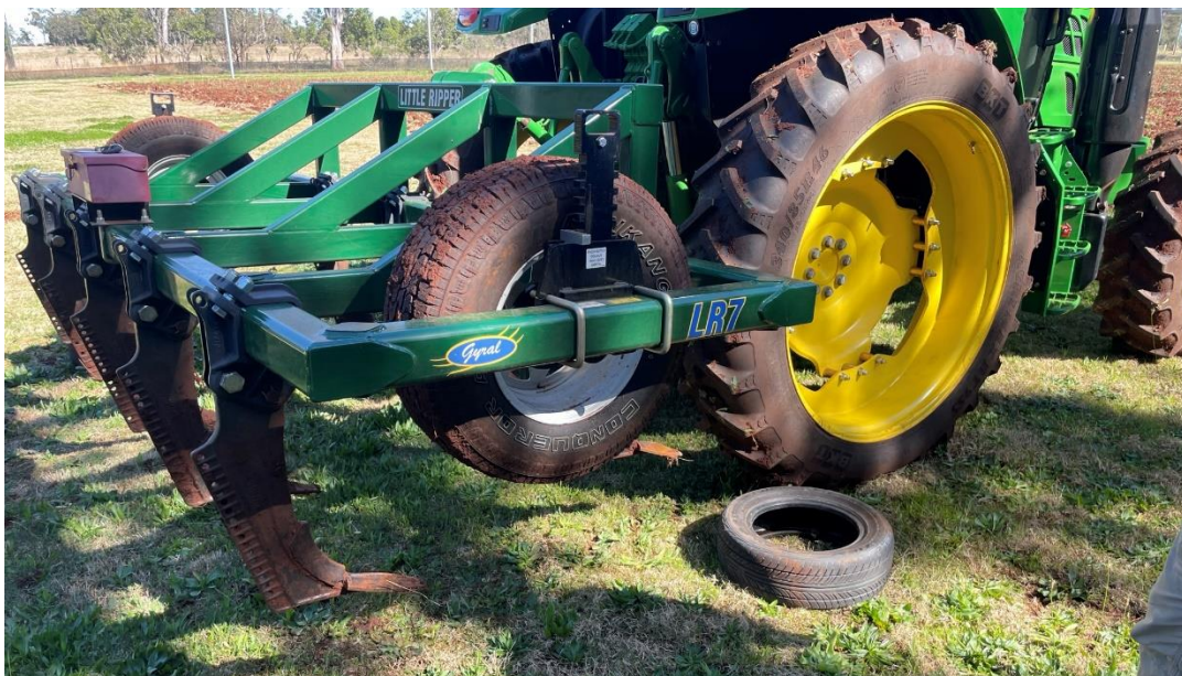
Figure 13 - Gyrat deep ripper fitted to the John Deere 6120R tractor
