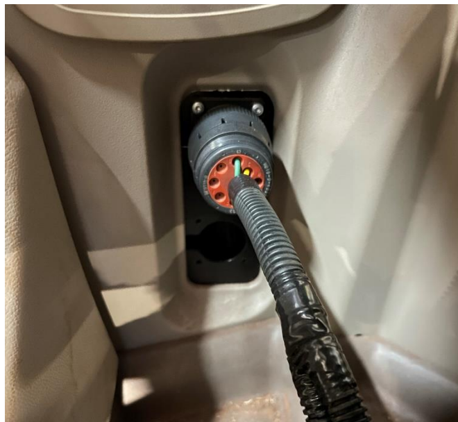
Figure 16 - Diagnostic connector and harness used for CAN Bus communication
