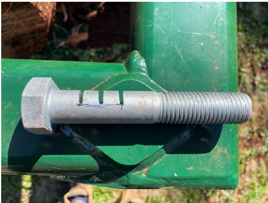
Figure 6 - M24 Bolts used as shear pins for the ripper shank breakage testing
