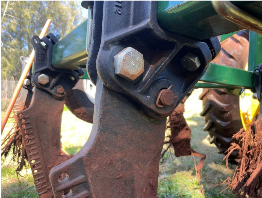
Figure 7 - Shear bolt installed in deep ripper ready for testing
