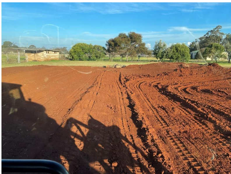
Figure 10 - Bank used to simulate the washout
