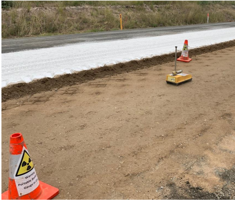
Figure 4. 5 – Density testing at the Braemar project (Source: Shaun Perkins 2020)
