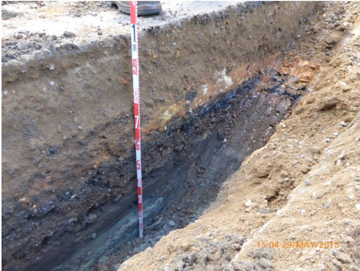
Figure 4. 2– Test pit in existing pavement at the Braemar project (Source: Roads and Maritime Services 2019)
