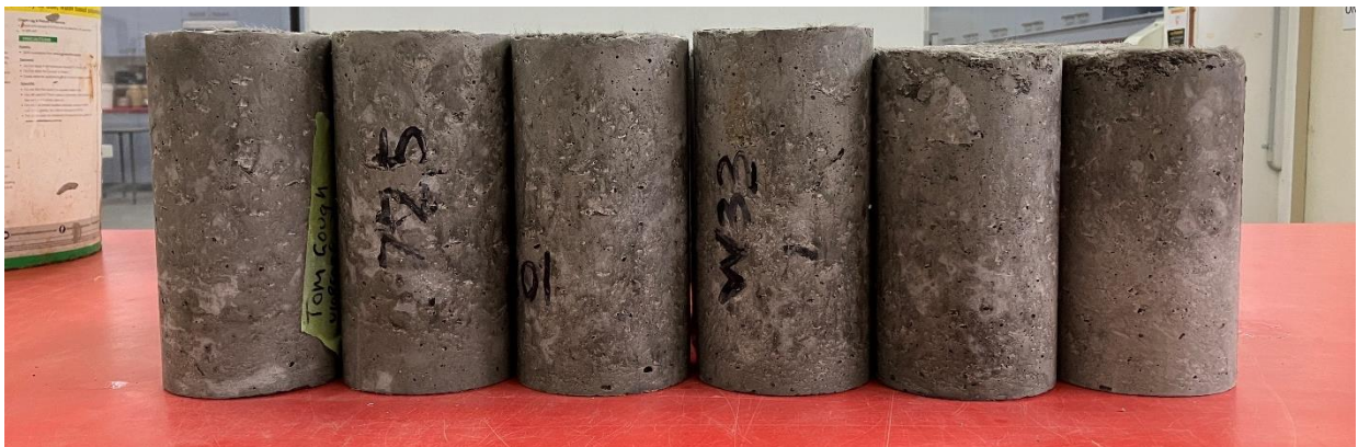
Figure 4.15 – Cylinder height variations in the control batch
