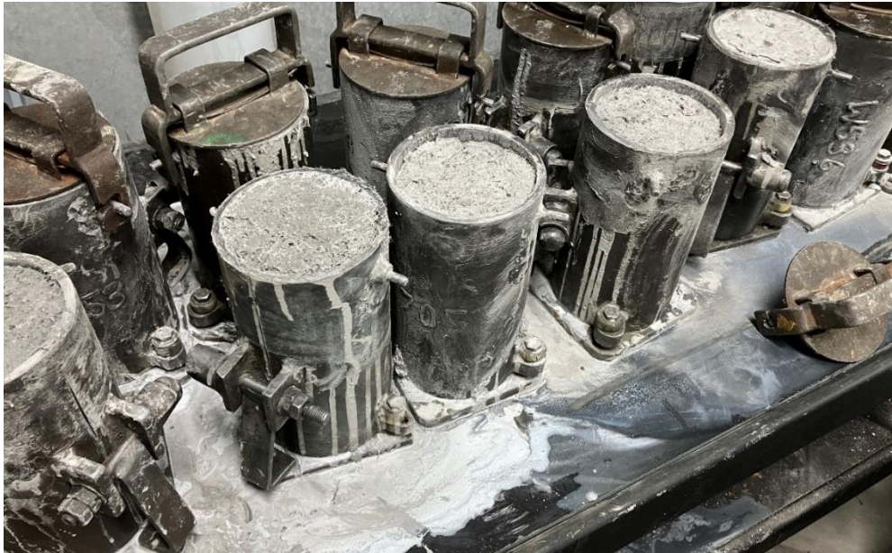
Figure 4.11 – Control batch cylinder paste loss and table accumulation
