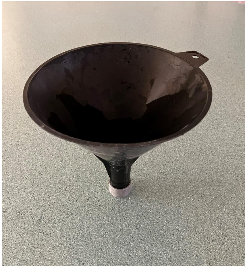
Figure 3.4 – Custom made flow funnel used to indicate plastic viscosity
