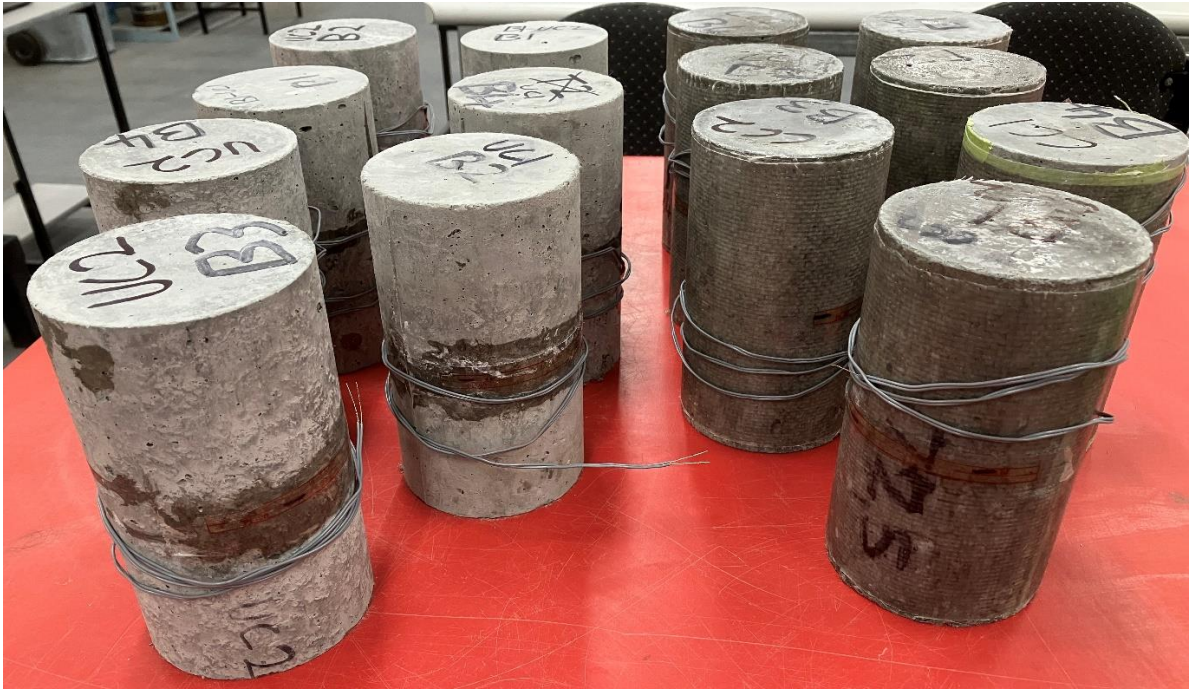
Figure 4.18 – Compression cylinders ready for testing
