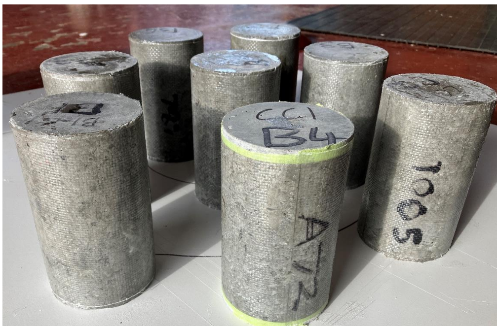
Figure 4.17 – GFRP wrapped cylinders
