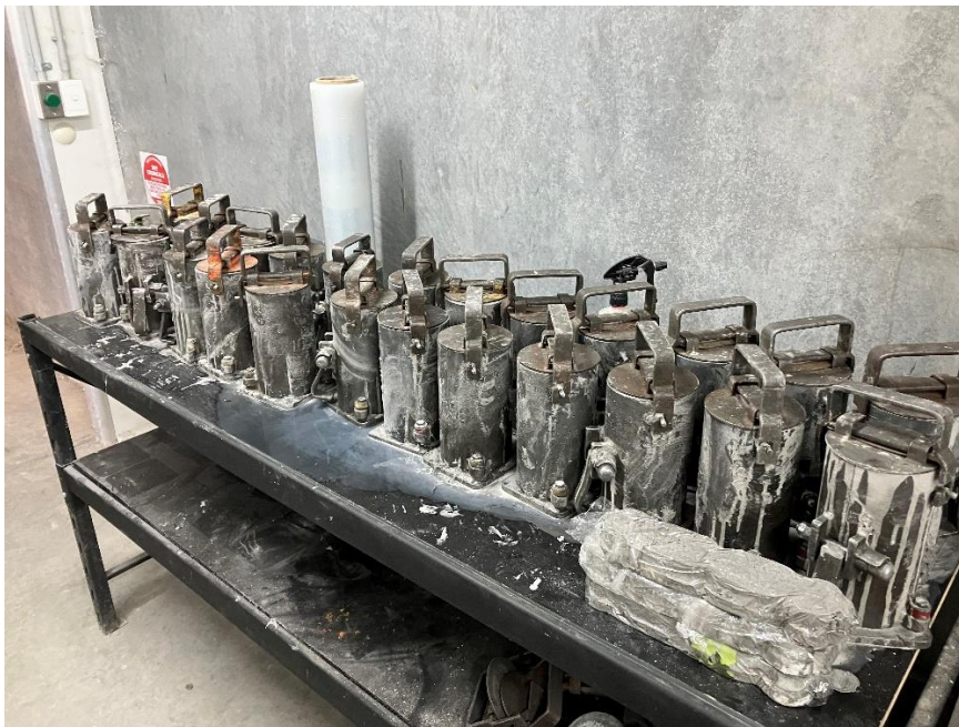
Figure 4.10 – Cylinder and briquette specimens' initial cure
