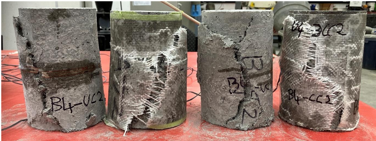
Figure 6.25 – Unconfined and Confined 50% PET-ECC failure patterns
