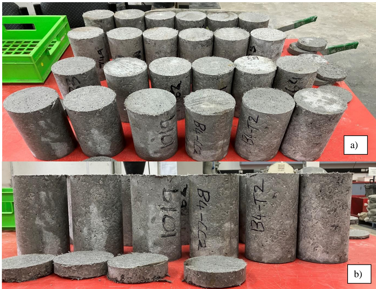
Figure 4.16 – a) top, b) side of all cylinders cut level to 170 mm height
