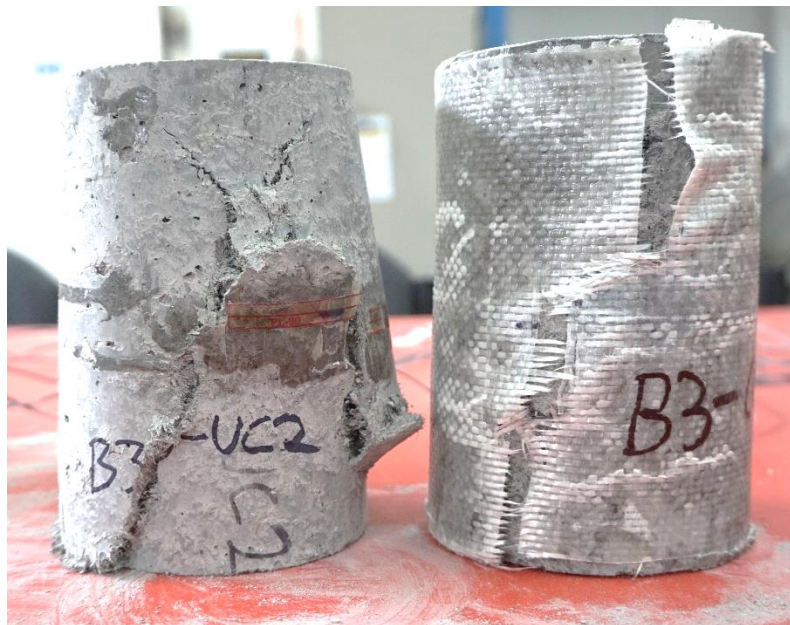
Figure 6.23 – Unconfined and confined 30% PET-ECC failure patterns
