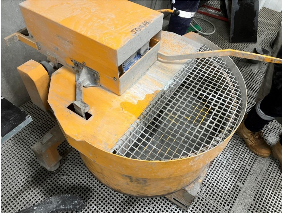
Figure 3.1 – Bennett equipment pan mixer
