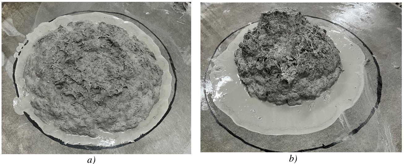
Figure 4.8 – ECC slump flow tests a) 0% PET-ECC, b) 50% PET-ECC
