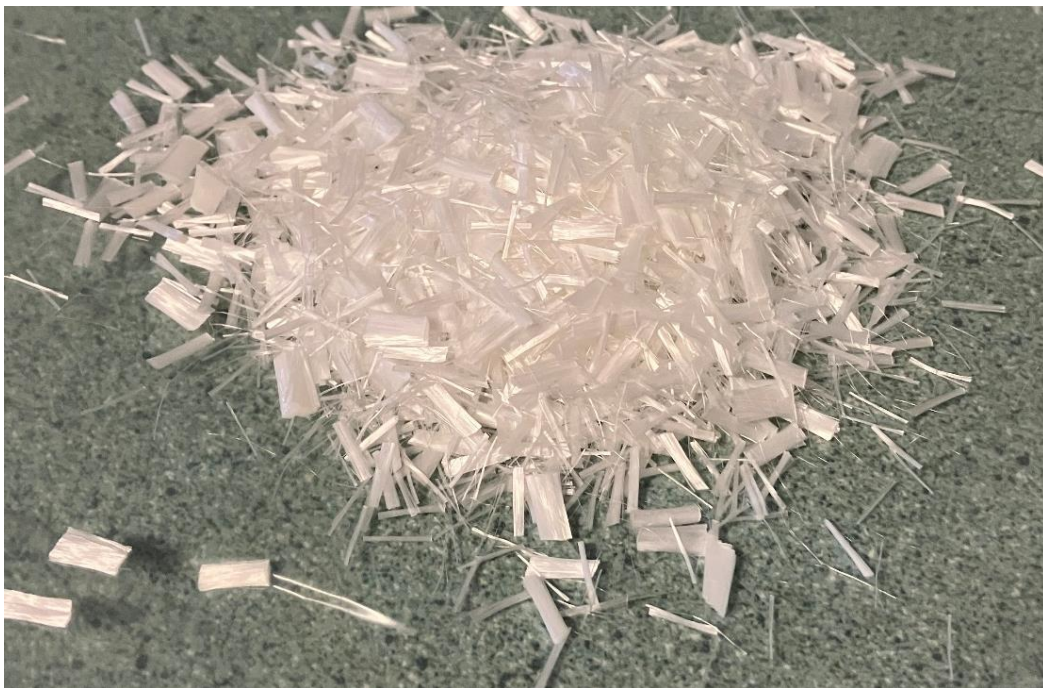
Figure 4.2 – RECS15 PVA fibre
