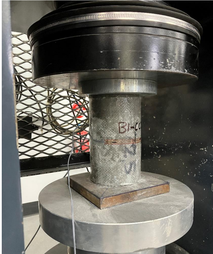
Figure 4.24 – Control GFRP cylinder under compression with centralized fibre rupture
