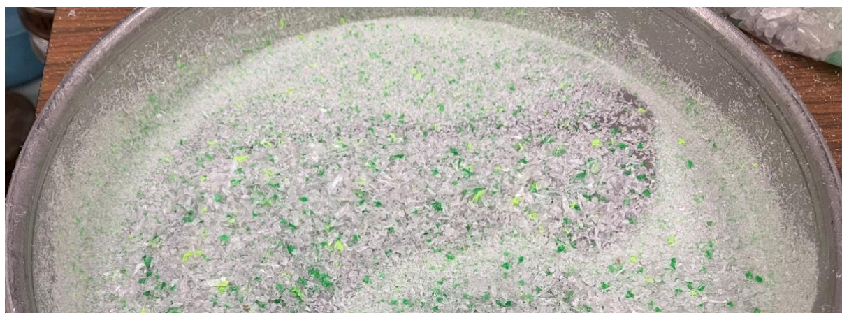
Figure 4.1 – Example particle sizes of the fine PET aggregate fraction
