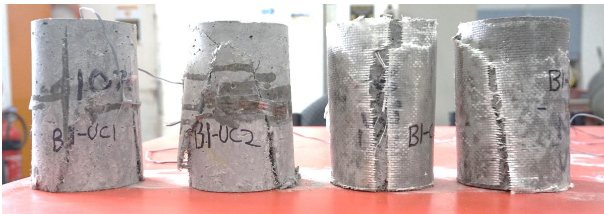
Figure 6.19 – Unconfined and confined control failure patterns
