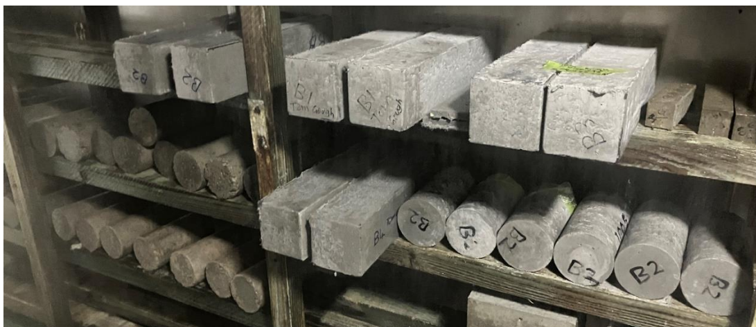
Figure 4.12 – Several PET-ECC specimens in the UniSQ fog room
