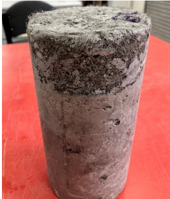
Figure 4.14 – Cylinder bleeding defect in 10% PET-ECC
