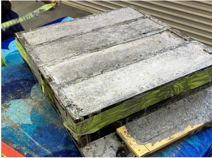
Figure 4.9 – Flexural specimens cast and covered in custom made form ply moulds
