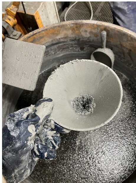
Figure 6.2 – 50% PET-ECC mortar aggregates stuck in flow cone
