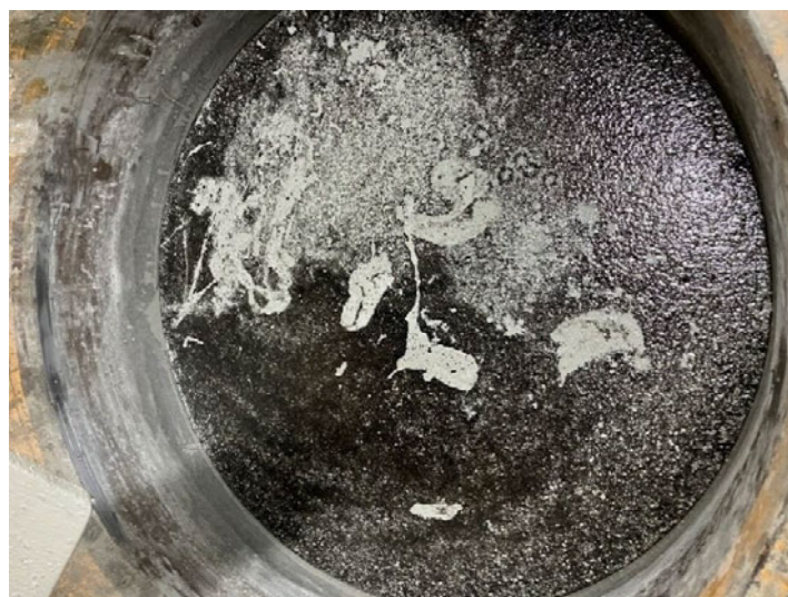
Figure 6.4 – In pan mortar reaction with 50% PET content
