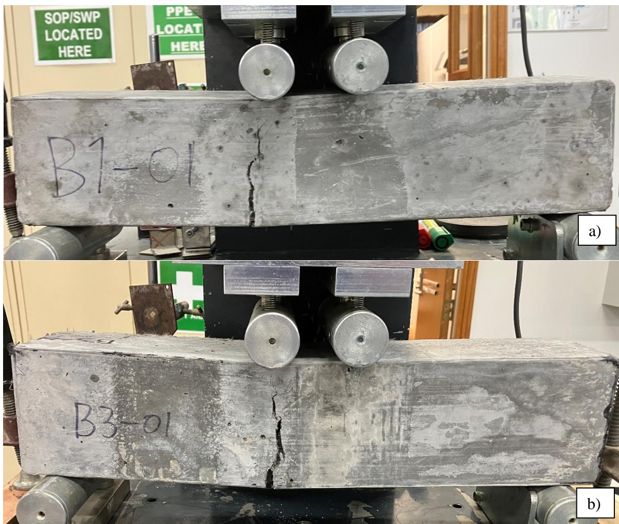
Figure 6.13 – Characteristic flexural tension failure a) control, b) 30% PET-ECC
