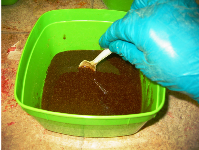
Figure 3. 5: Resin, sawdust and catalyst mixed by gradual stirring
