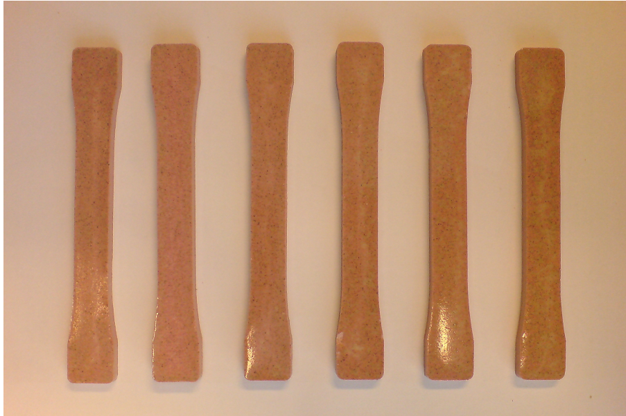
Figure 3. 8: Naturally cured specimen after removal from mold (Ready for heat treatment)
