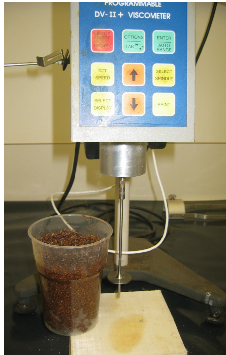
Figure E. 1: Brookfield Programmable DV-II+ viscosity testing machine
