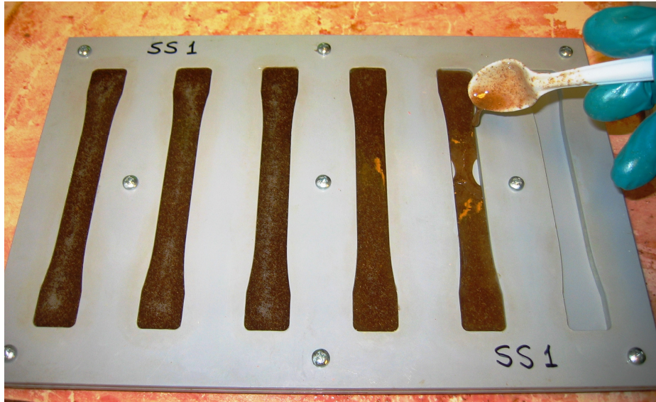
Figure 3. 6: Resin, catalyst and sawdust mixture poured in the mold
