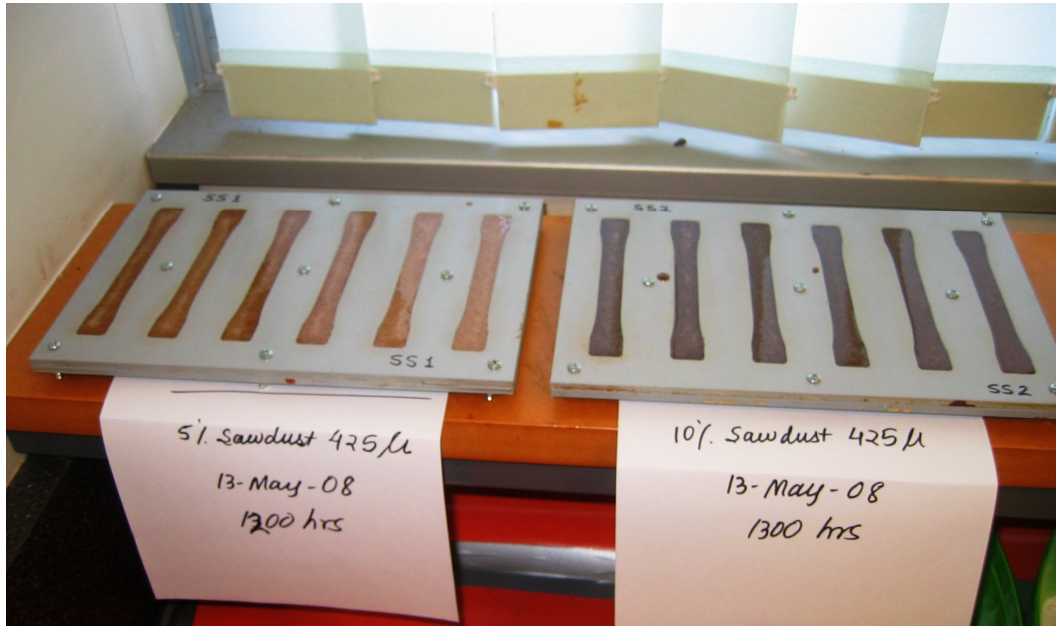
Figure 3. 7: Natural curing of resin mixture at room temperature for 48 hours or more
