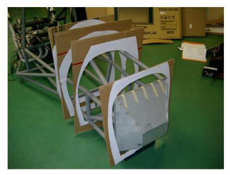
Figure 6.14: Checking nosecone fit with cardboard sections
