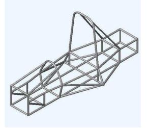
Figure 6.1: Solid model of the chassis
