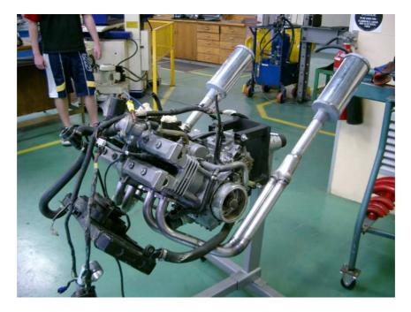
Figure 6.4: The exhaust system mounted to the engine
