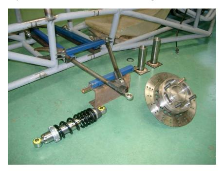
Figure 6.9: Modified front suspension under construction
