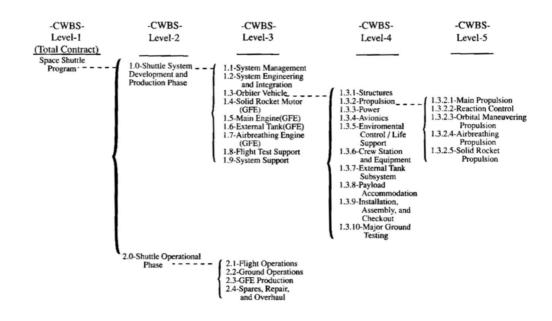
Figure 5.2: Work Breakdown Structure for a space shuttle program
