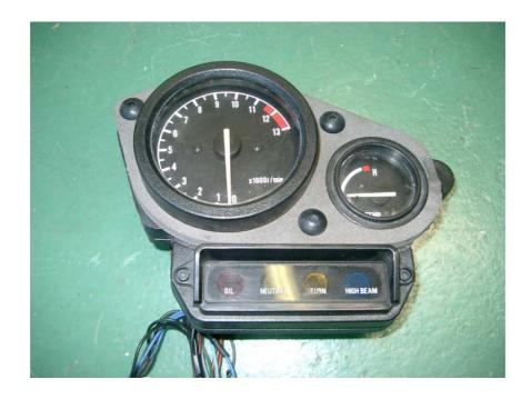
Figure 6.13: Jettison 1 uses a modified gauge cluster from the donor bike
