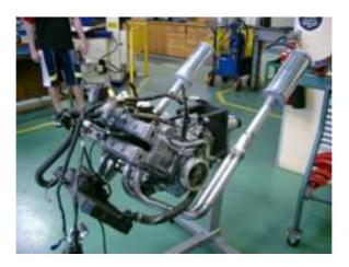
Figure D.3: Twin exhaust and custom mufflers results in equal back-pressure to all cylinders and facilitates tuning of the system.
