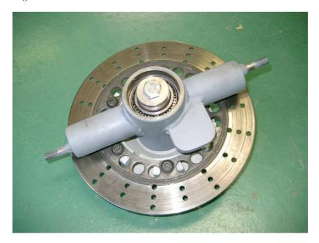
Figure 6.6: Front upright, hub and rotor assembly prior to modification
