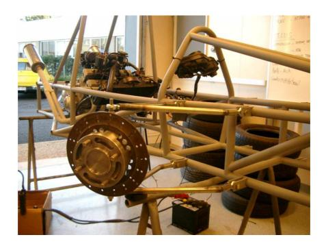
Figure 6.8: Initial front suspension design showing the angled wishbones
