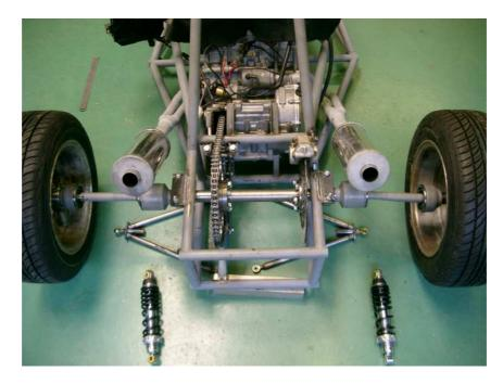
Figure 6.7: Rear suspension under construction
