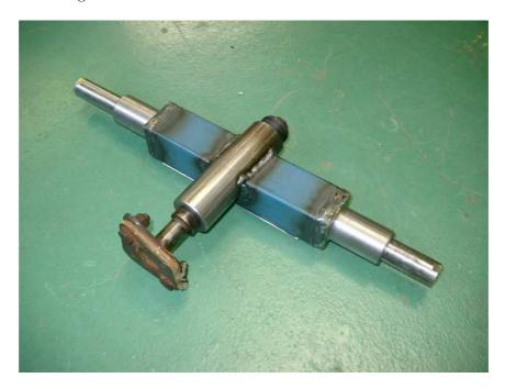
Figure 6.5: The modified steering rack during construction
