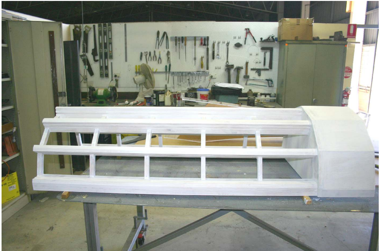
Figure 3. – Construction of Wooden Inlet Tower
