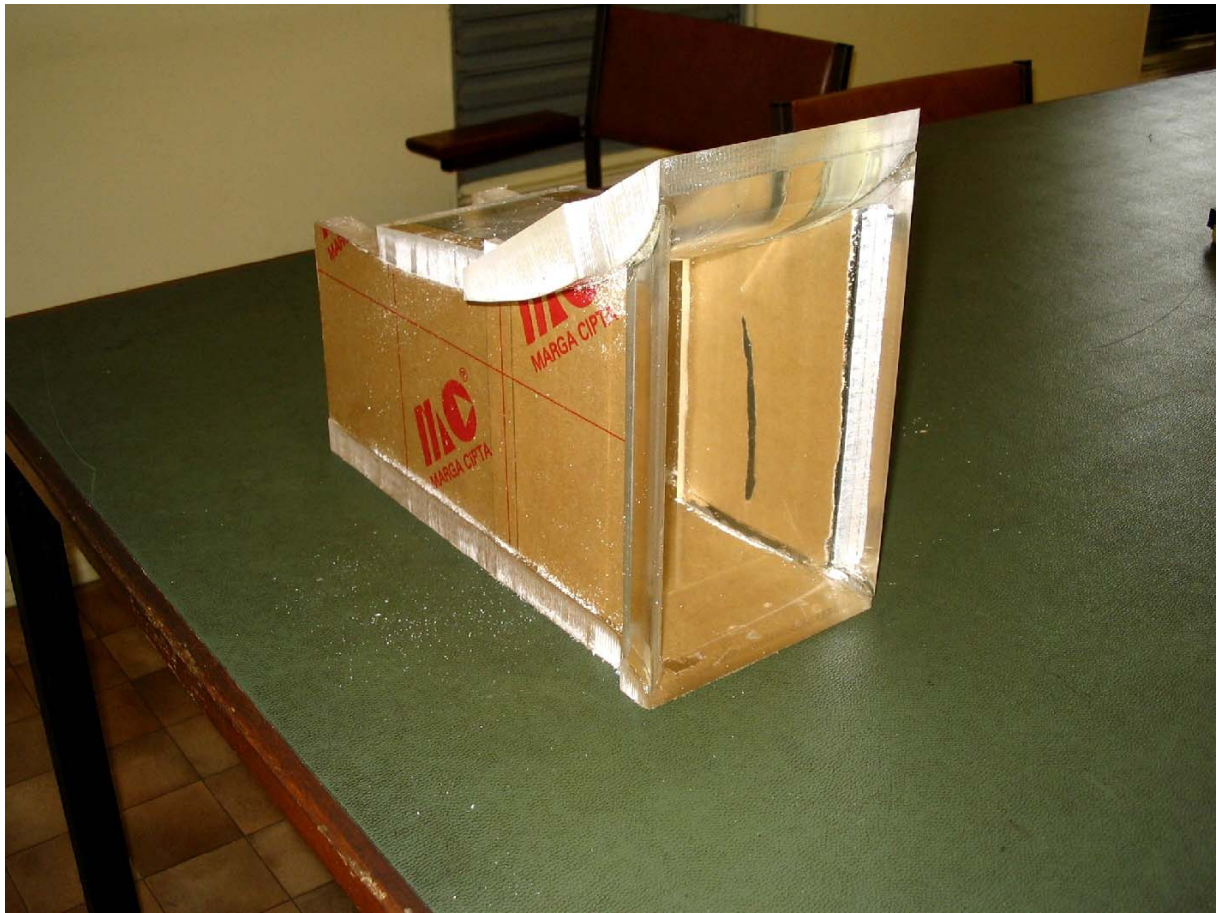
Figure 4. – Machined Rectangular Bellmouth
