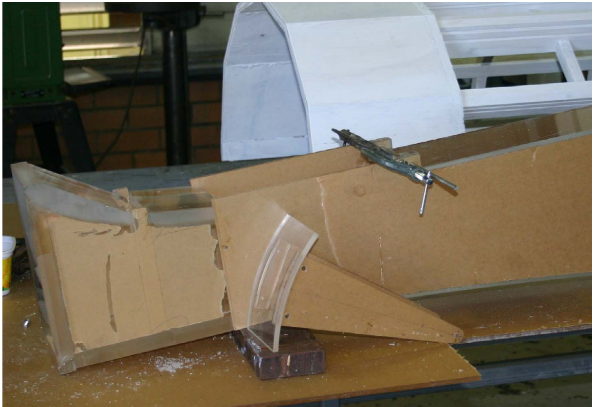
Figure 5. – Construction of Radial Gate and Outlet Chute
