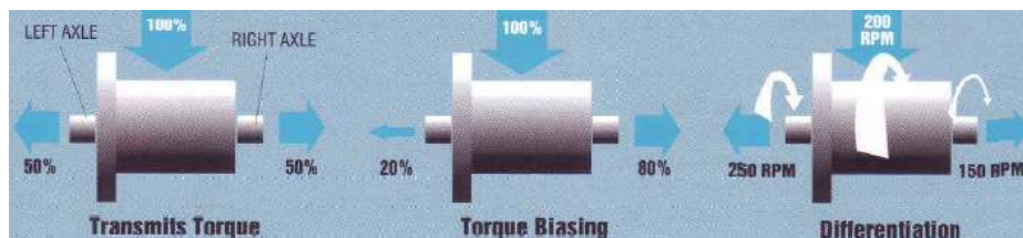
Figure 5.4: Torque biasing action
