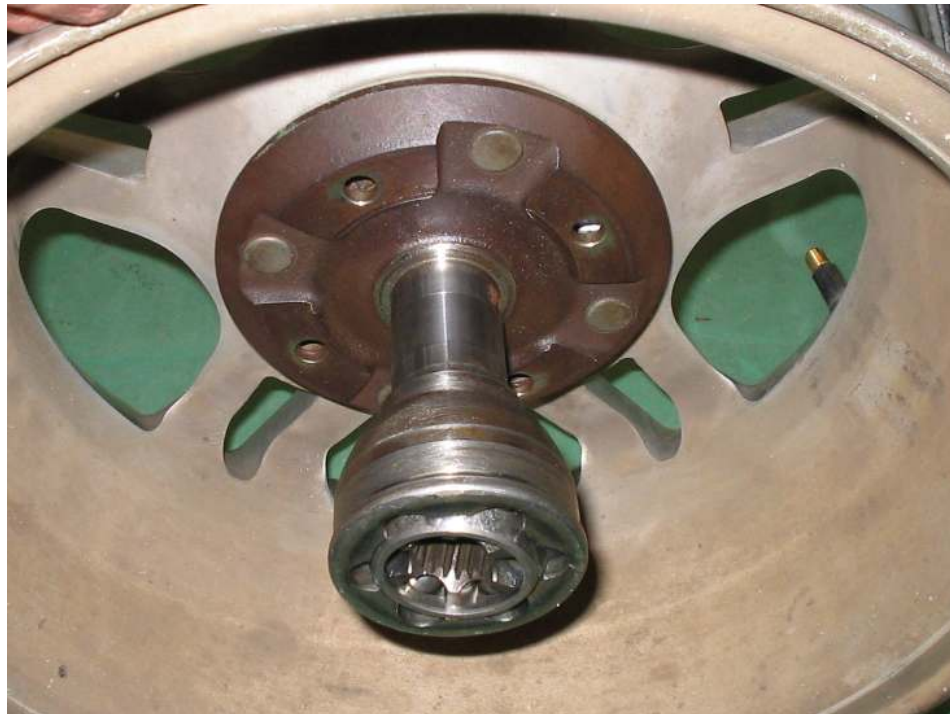
Figure 6.4: Outer CV and hub fitted to wheel
