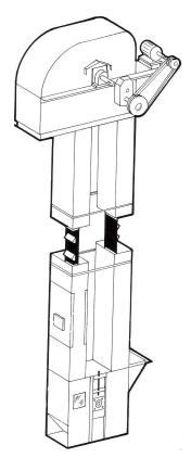
Figure 1-1 Bucket Elevator
