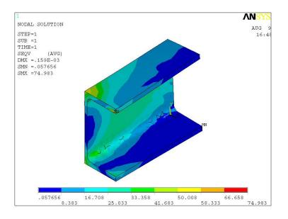
Figure 7-2 Motor Bracket Channel FEA Results
