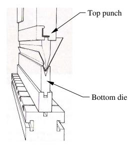
Figure 4-6 Brake press with gooseneck tooling
