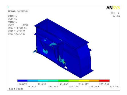
Figure 7-9 FEA results with worn end panels
