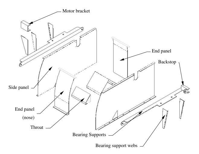
Figure 3-2 Head Structure Exploded view
