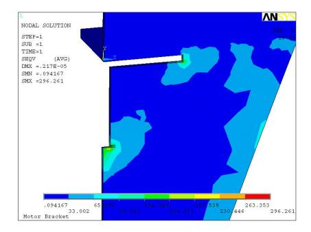
Figure 7-3 Motor Bracket with Omitted Angle FEA Results
