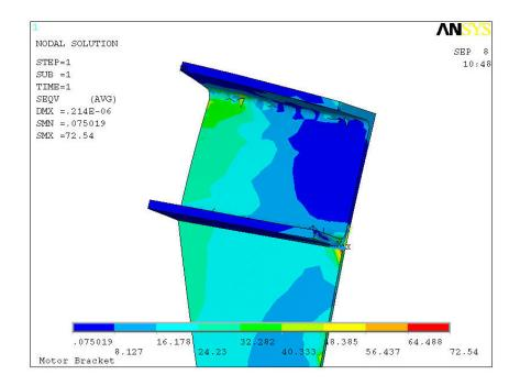
**Figure 7-4 Motor Bracket Final FEA Results**
