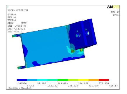
Figure 7-6 Backstop Bracket with Weld Fillet FEA Results
