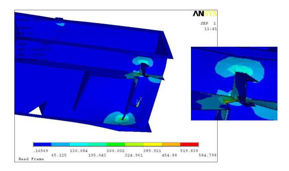
Figure 7-11 FEA results with motor in reverse
