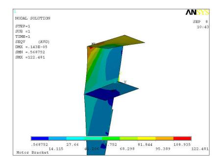
Figure 7-1 Motor Bracket Shell Model FEA Results
