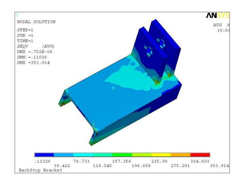
Figure 7-5 Backstop Bracket FEA Results
