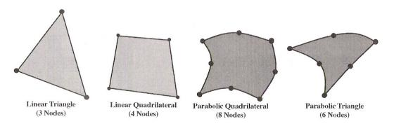
Figure 5-2 Linear h-elements & Parabolic p-elements
