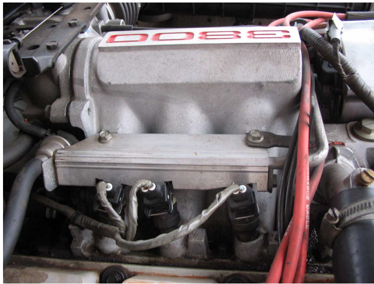
Figure 5.13: Typical cast inlet manifold, promoting charge robbery
