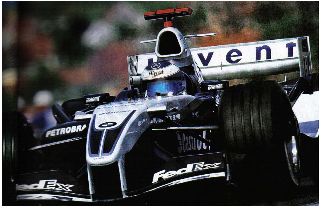
Figure 5.2: Airbox used in open-wheel racing
