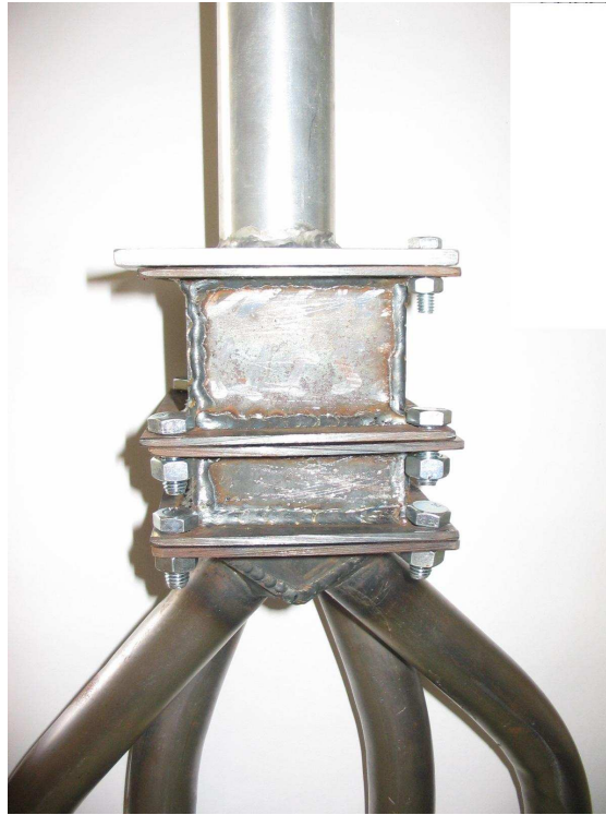
Figure 6.15: Restrictor, plenum spacers and manifold assembly
