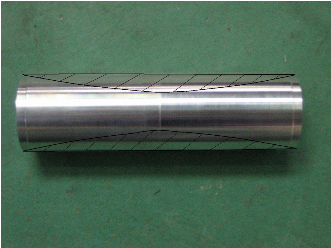
Figure 6.23: Aluminium restrictor, with proposed outside taper to reduce weight
