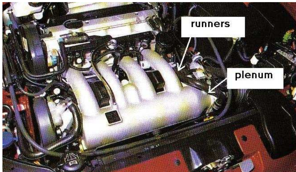
Figure 5.6: Intake runners extending from a common volume, or plenum
