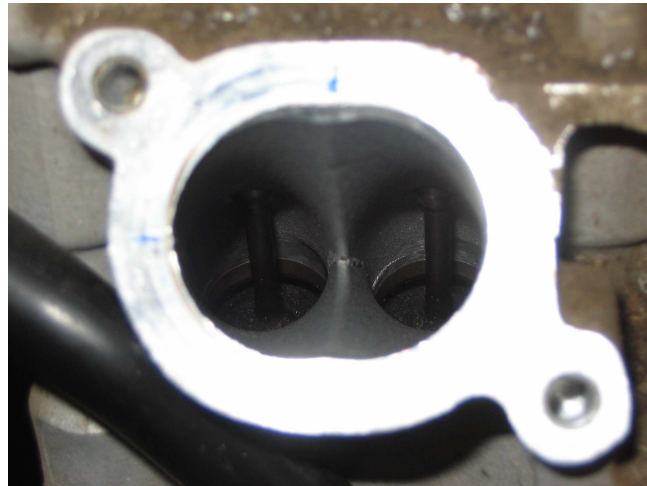
Figure 4.5: Steeply angled, direct inlet port of the 1994 YZF600
