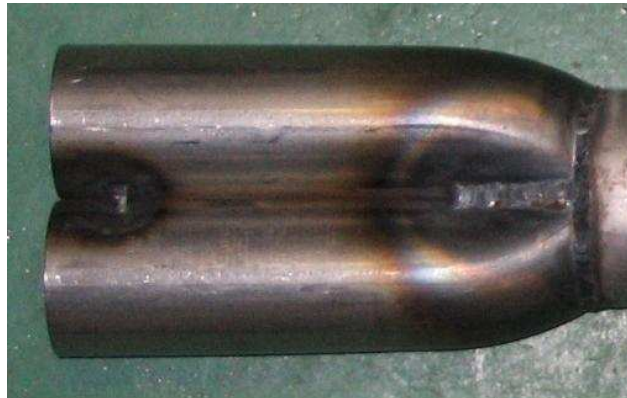
Figure 9.5: Free-flow collectors, created from 180° mandrel bends
