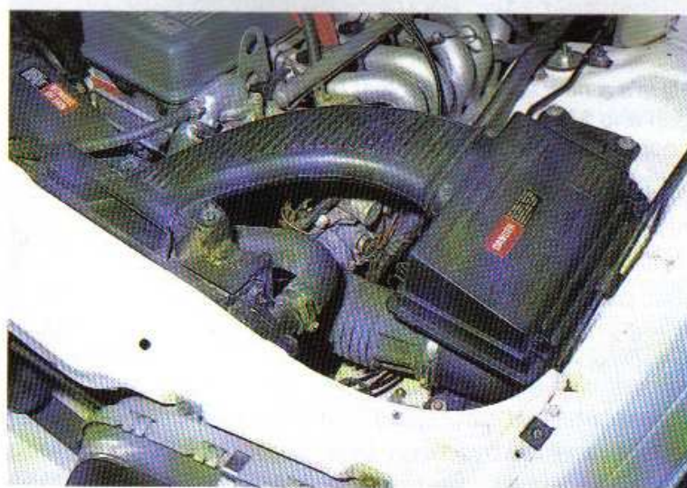
Figure 5.3: Air intake in standard road car, situated close to engine, increases intake air temperature
