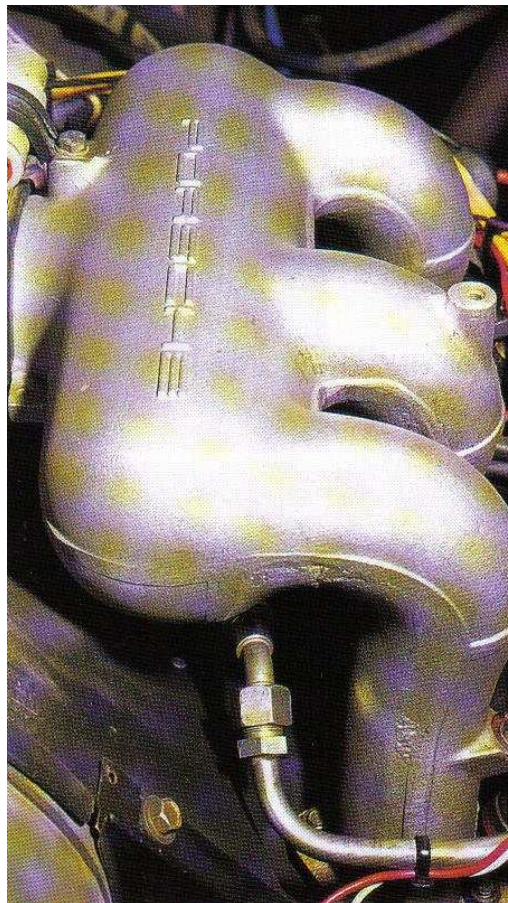
Figure 5.10: Direct path followed by intake charge from plenum to cylinders
