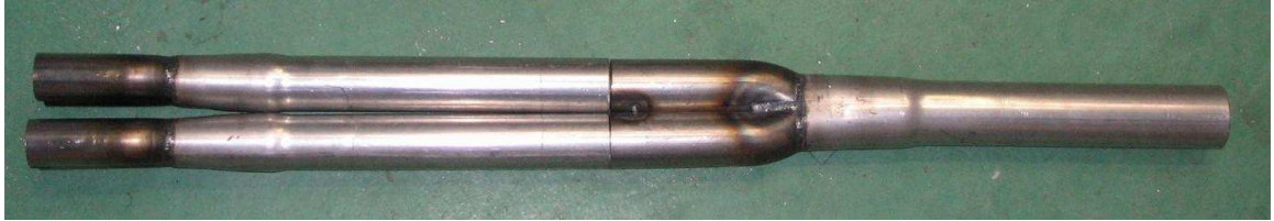
Figure 9.4: Secondary pipes feeding into 'tertiary' tailpiece
