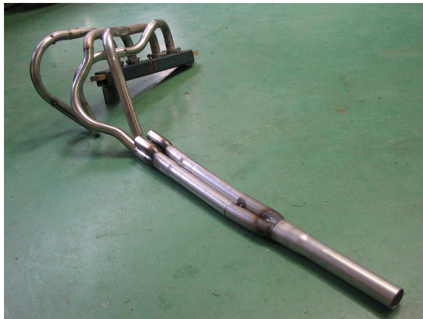
Figure 9.9: The 2005 exhaust system mid-construction, made from mild steel
