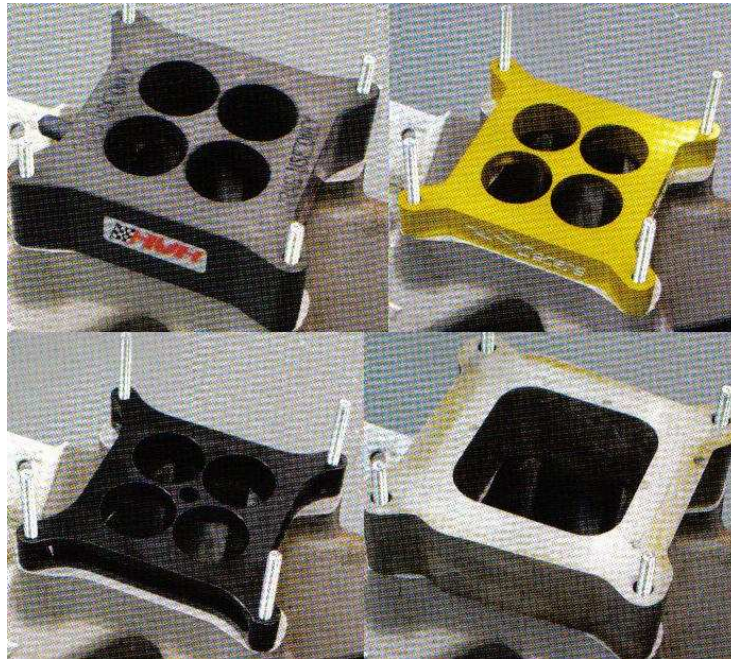
Figure 4.10: Some of the variety of manifold spacers available, each offering different wave tuning characteristics
