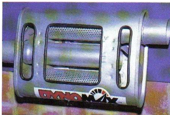
Figure 9.6: Cut-away view showing complicated path of exhaust gases through reverse-flow muffler
