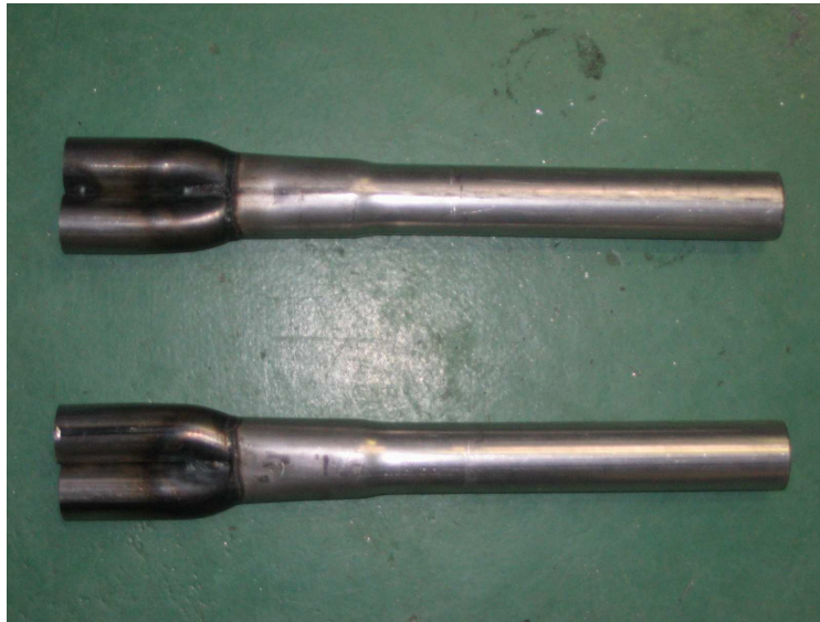
Figure 9.3: Secondary pipes for 2005 exhaust system
