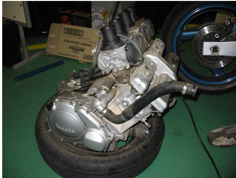
Figure 2.2: 1994 Yamaha YZF600 engine for use in 2005 USQ race car
