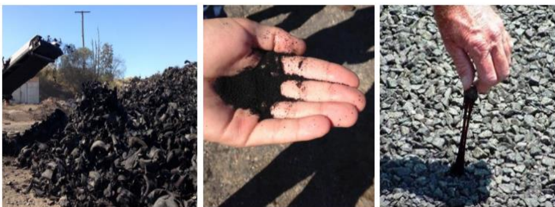
FIG 18: Crumb Rubber in CRM Binder (Department of Transport and Main roads, 2020)
