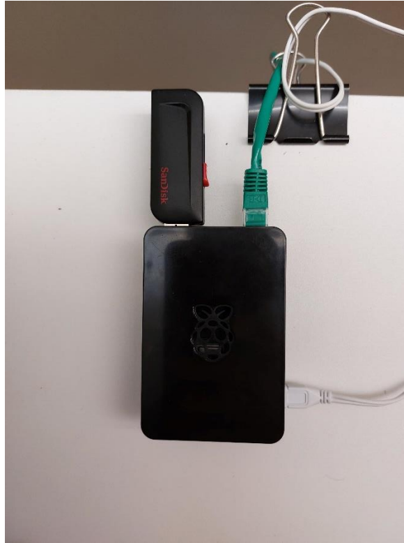
Figure 18. Raspberry Pi 3B+ with required connections for CSI capture
