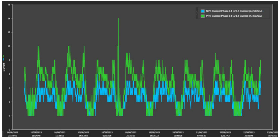
Figure 66 - Ratio of NPS/PPS Current Plot at Low Load from Ausgrid Device
