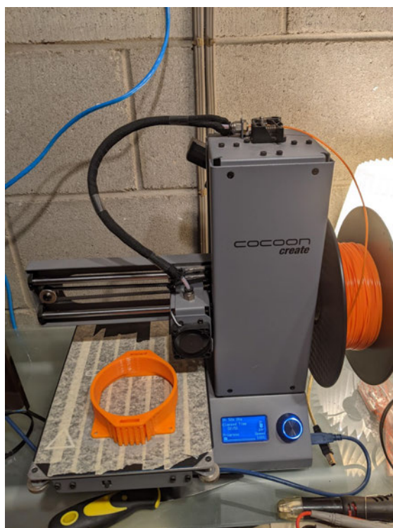
Figure 10: The FDM 3D printer used to produce physical parts of the apparatus.
