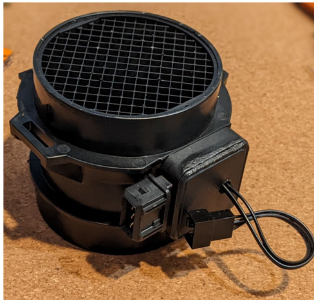
Figure 3: The Siemens VDO 5WK9605 MAF sensor.
